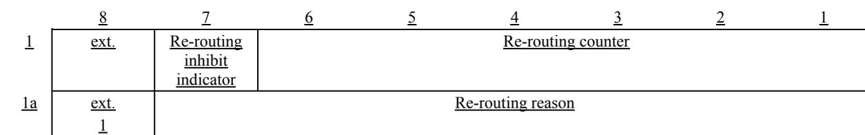
**Figure 95/Q.763 – Automatic re-routing parameter field**
