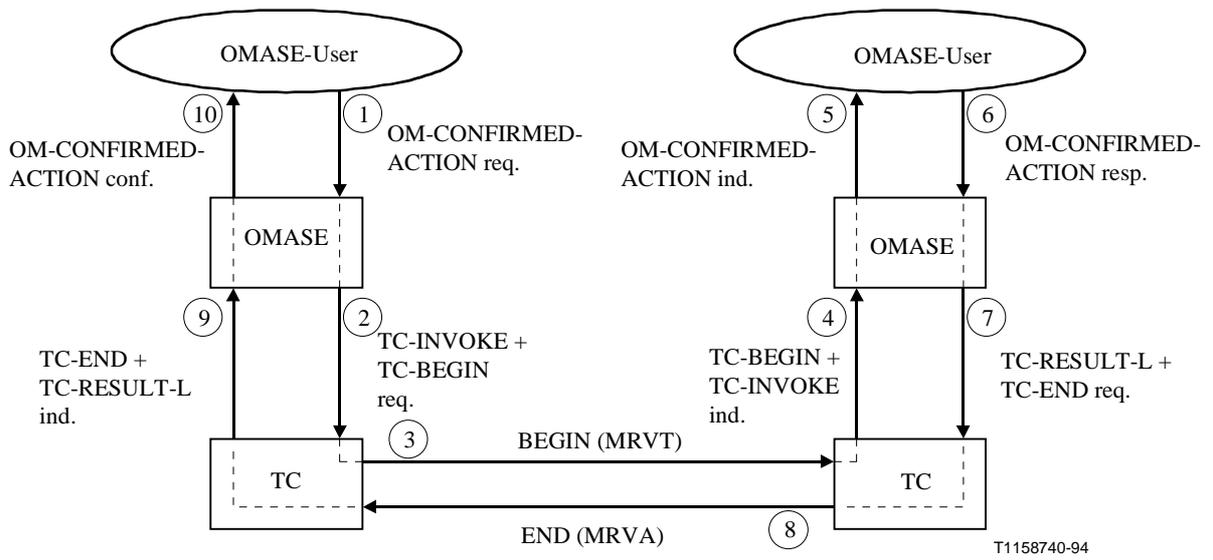
**Figure A.2/Q.754 – Example use of primitive interfaces**
