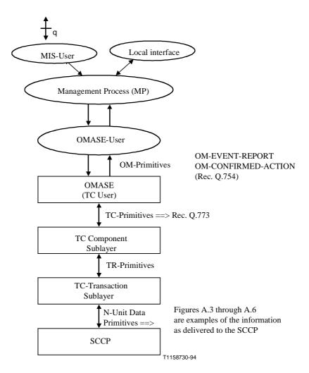
Figure A.1/Q.754 – Primitive interfaces
