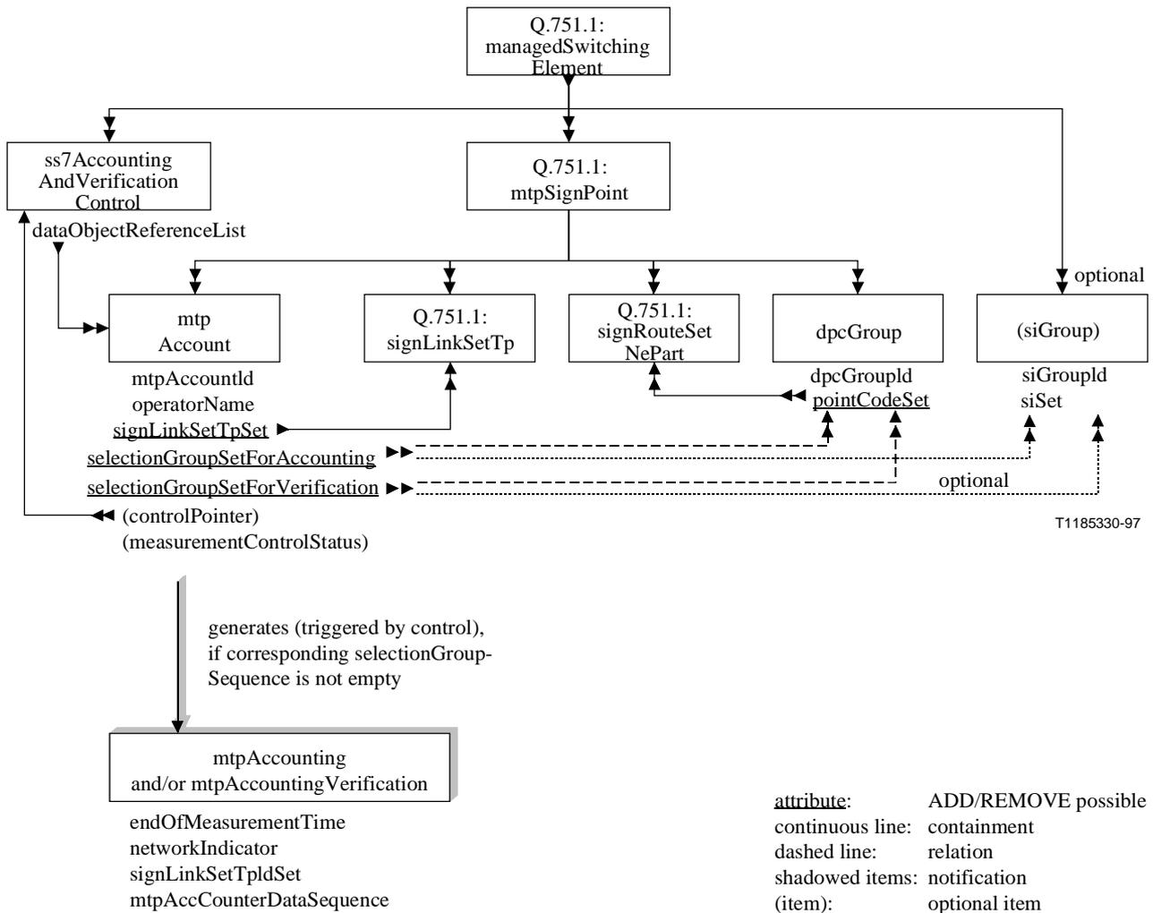
**Figure 2/Q.751.3 – ERD: Diagram for MTP accounting and verification**
