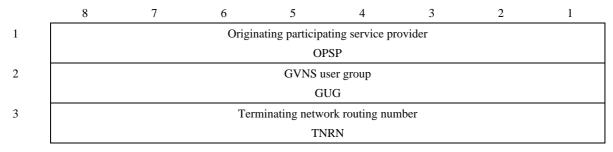
Figure 6-1/Q.735.6 – Forward GVNS parameter field
