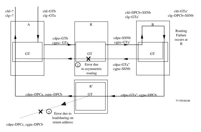
Figure 17/Q.715 – Example of message flow for return option in SCCP connectionless service
