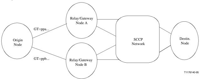
Figure 16/Q.715 – Network with replicated relay/gateway nodes
