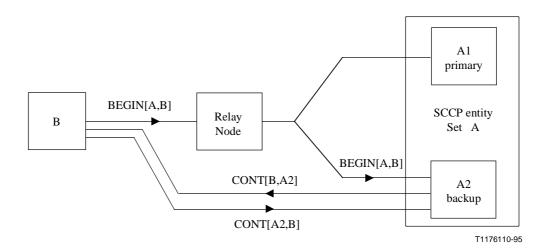
Figure 13/Q.715 – Addressing mechanism for TC based application, example
