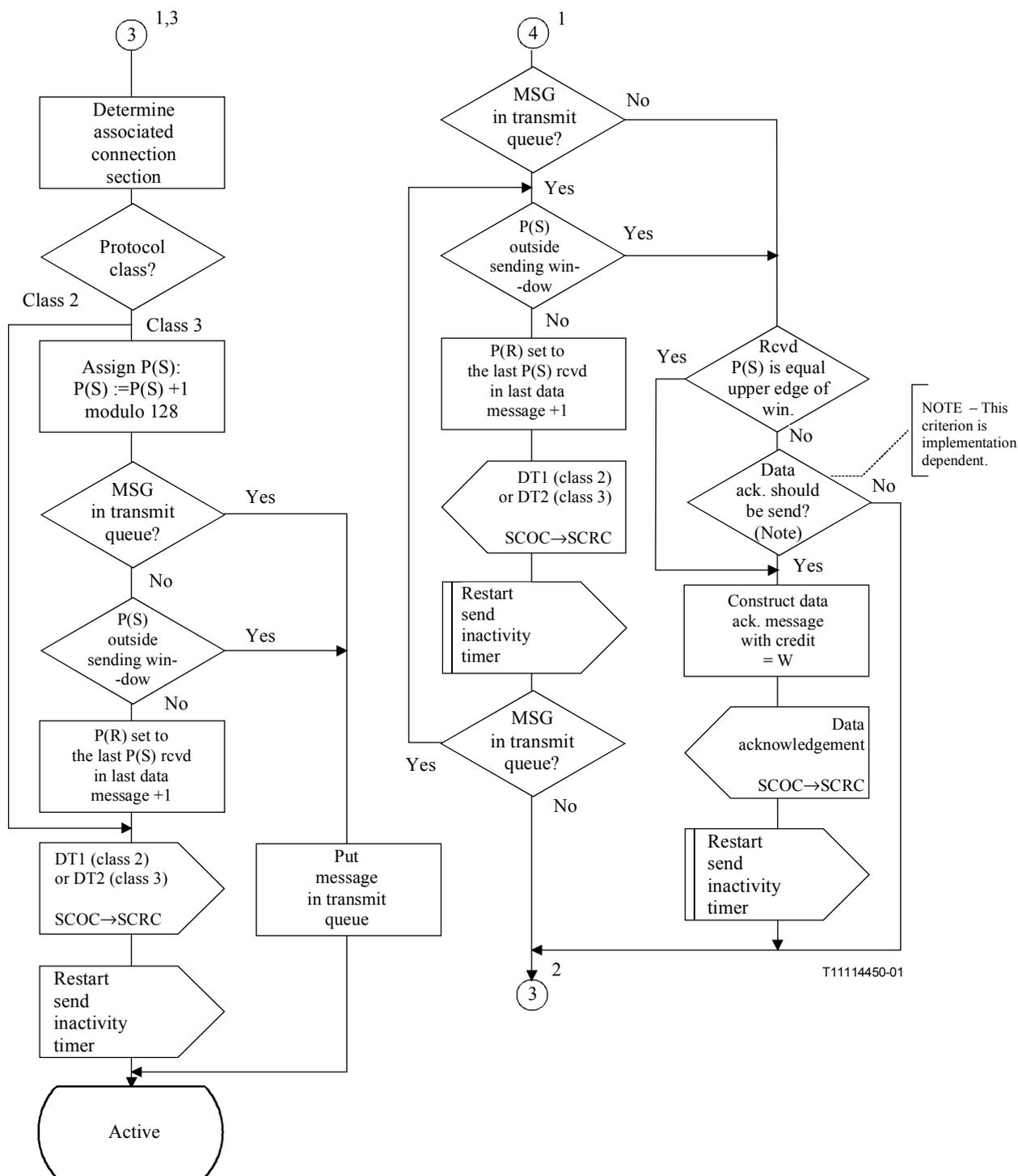
**Figure C.8/Q.714 – Data transfer procedures at relay node with coupling for SCCP connection-oriented control (SCOC) (sheet 3 of 4)**
