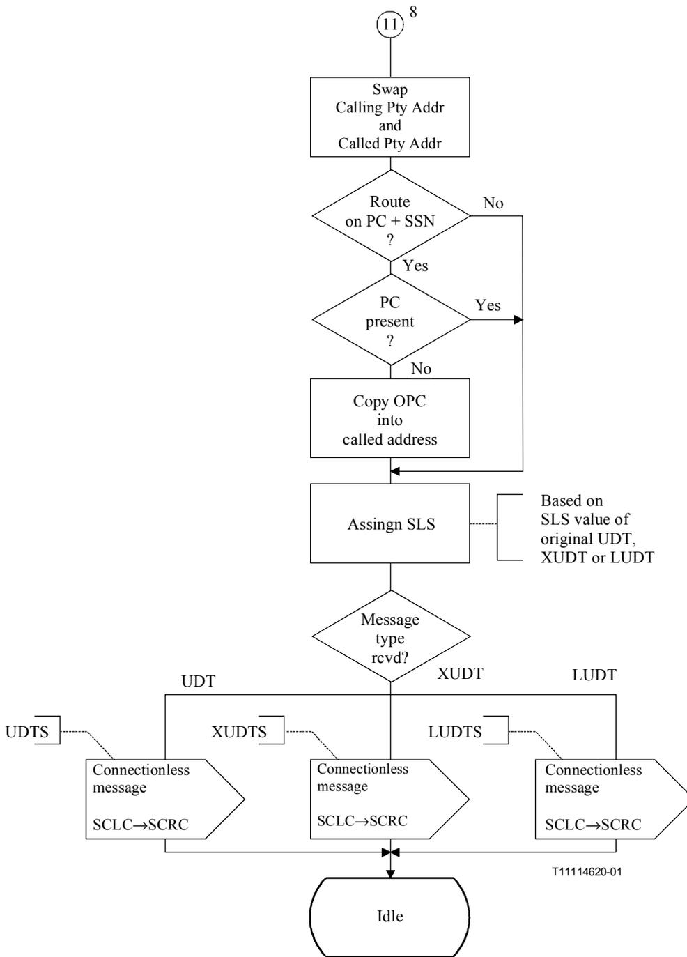
**Figure C.12/Q.714 – SCCP connectionless control (SCLC) (sheet 9 of 9)**
