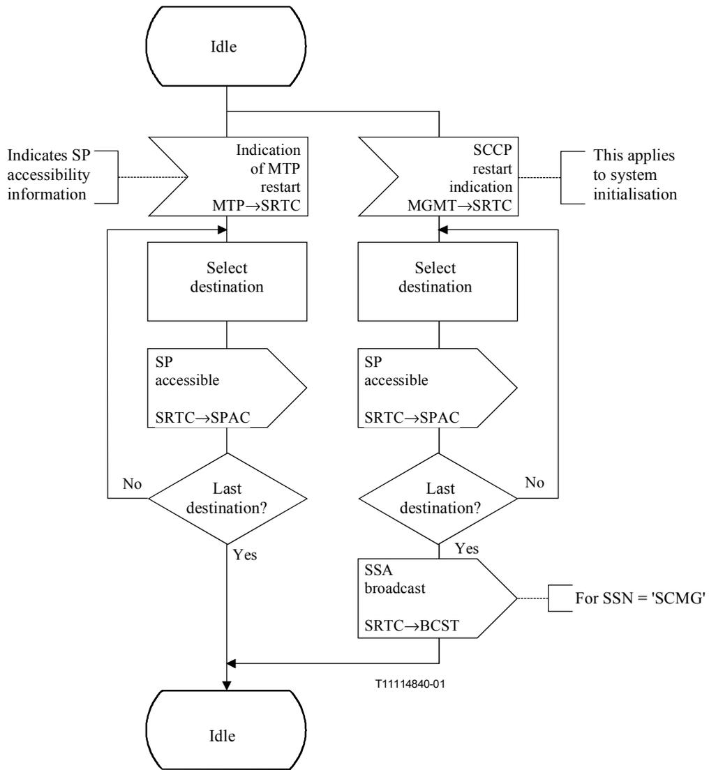
**Figure D.11/Q.714 – SCCP restart control (SRTC)**
