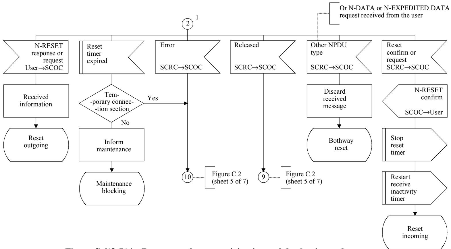
**Figure C.6/Q.714 – Reset procedures at originating and destination nodes for SCCP connection-oriented control (SCOC) (sheet 3 of 4)**
