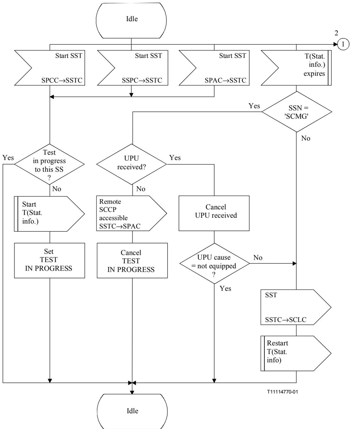
Figure D.7/Q.714 – Subsystem status test control (SSTC) (sheet 1 of 2)
