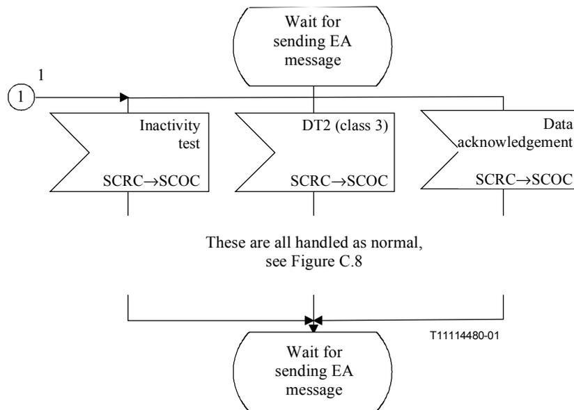
**Figure C.9/Q.714 – Expedited data transfer procedures at relay node with coupling for SCCP connection-oriented control (SCOC) (sheet 2 of 2)**
