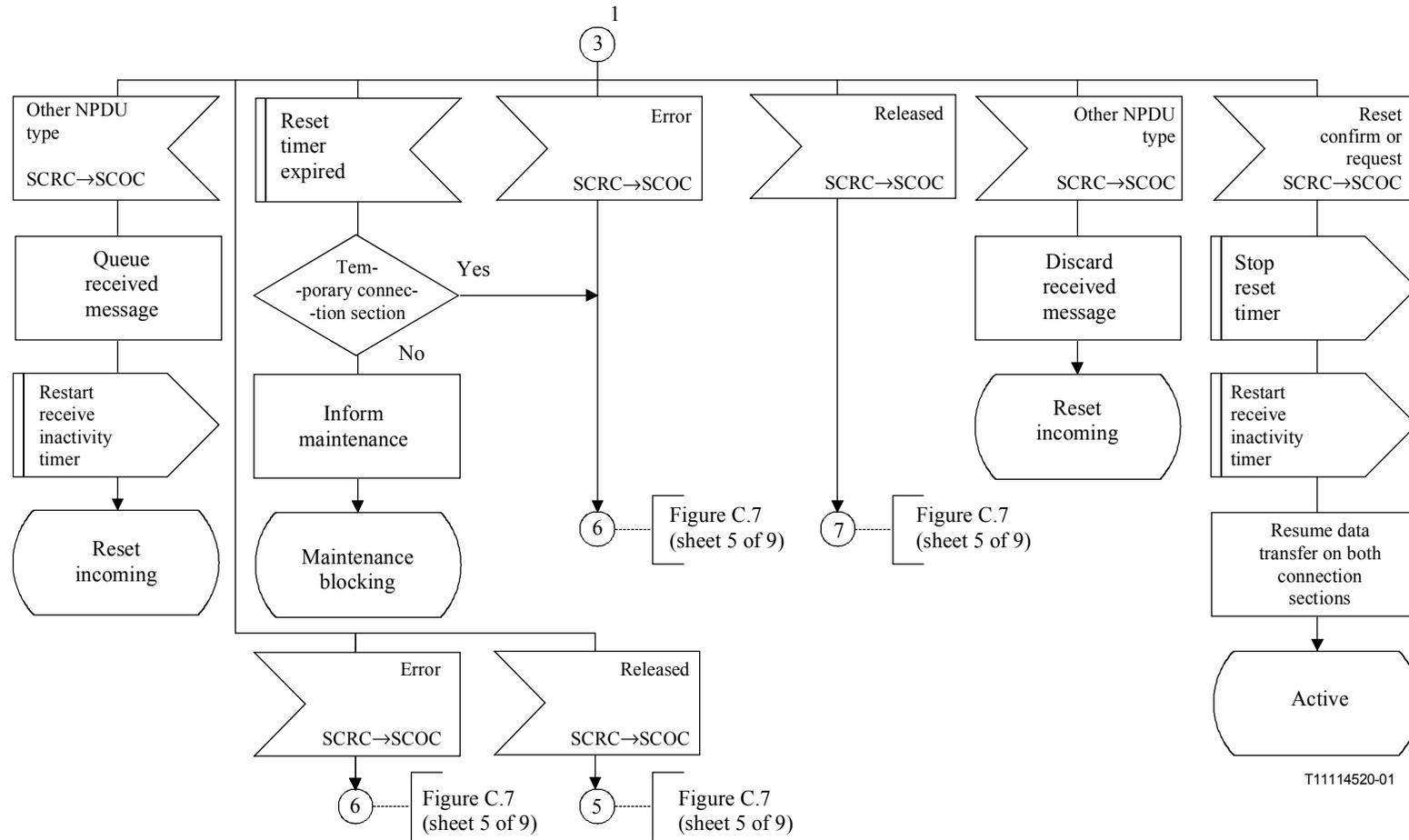
**Figure C.10/Q.714 – Reset procedures at relay node with coupling for SCCP connection-oriented control (SCOC) (sheet 4 of 4)**
