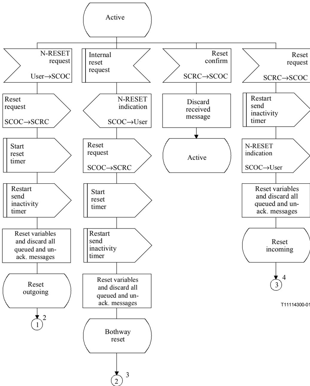
**Figure C.6/Q.714 – Reset procedures at originating and destination nodes for SCCP connection-oriented control (SCOC) (sheet 1 of 4)**
