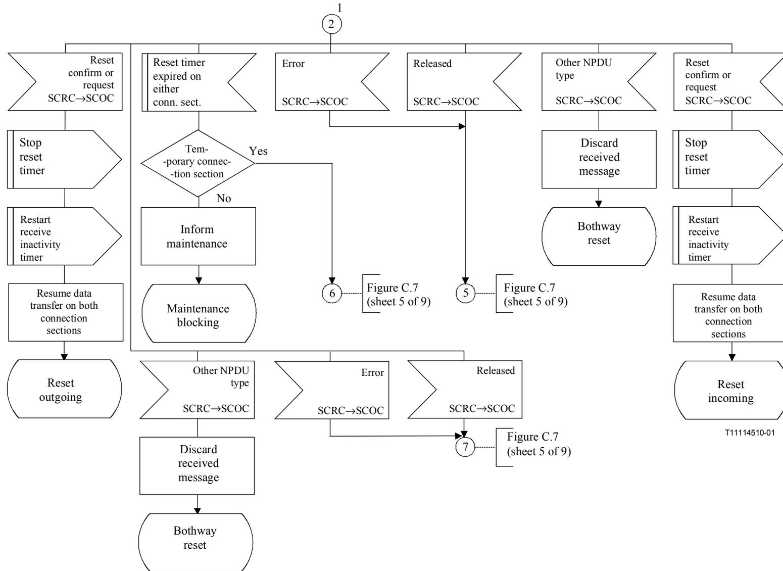
**Figure C.10/Q.714 – Reset procedures at relay node with coupling for SCCP connection-oriented control (SCOC) (sheet 3 of 4)**
