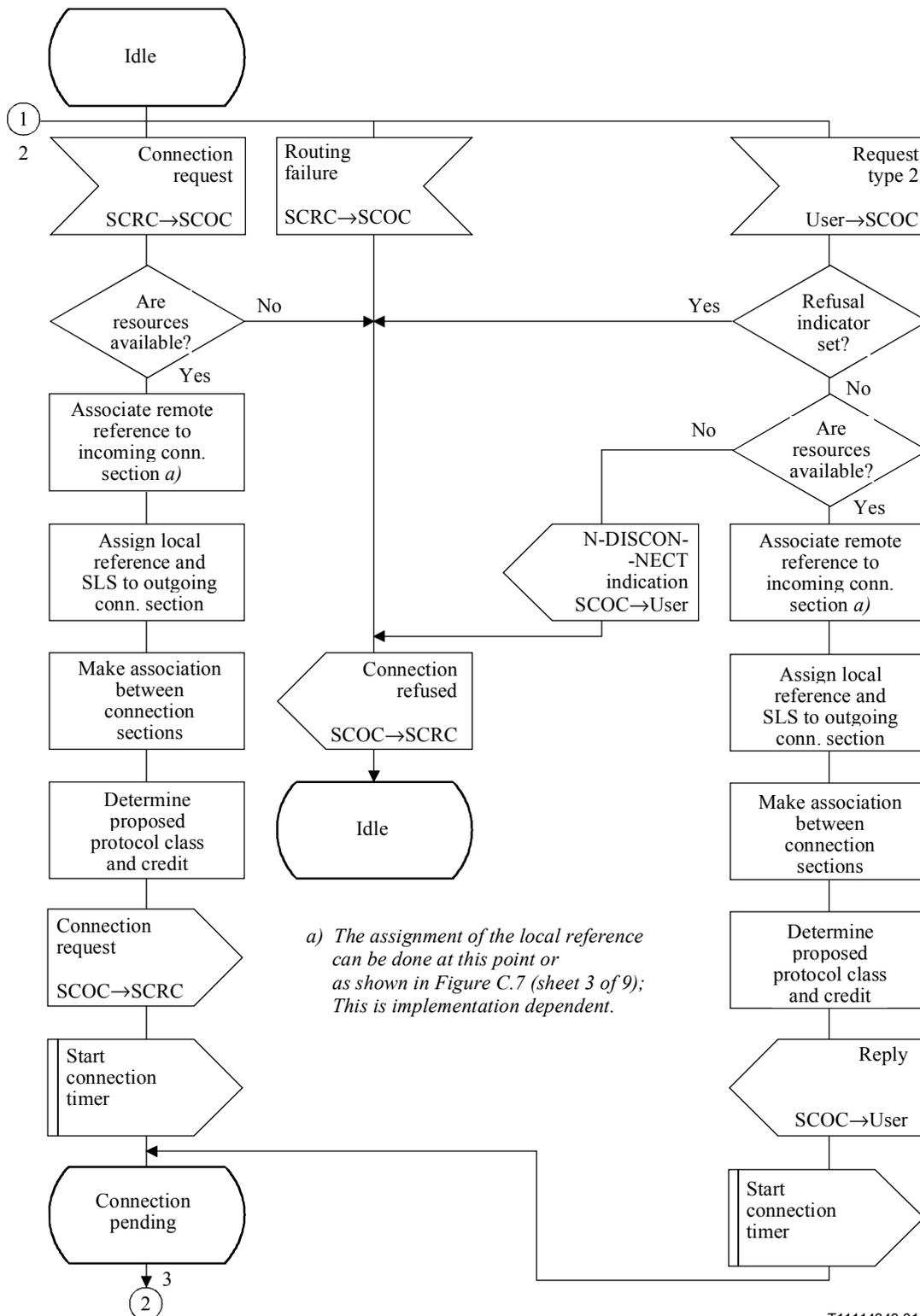
**Figure C.7/Q.714 – Connection establishment procedures at relay node with coupling for SCCP connection-oriented control (SCOC) (sheet 1 of 9)**
