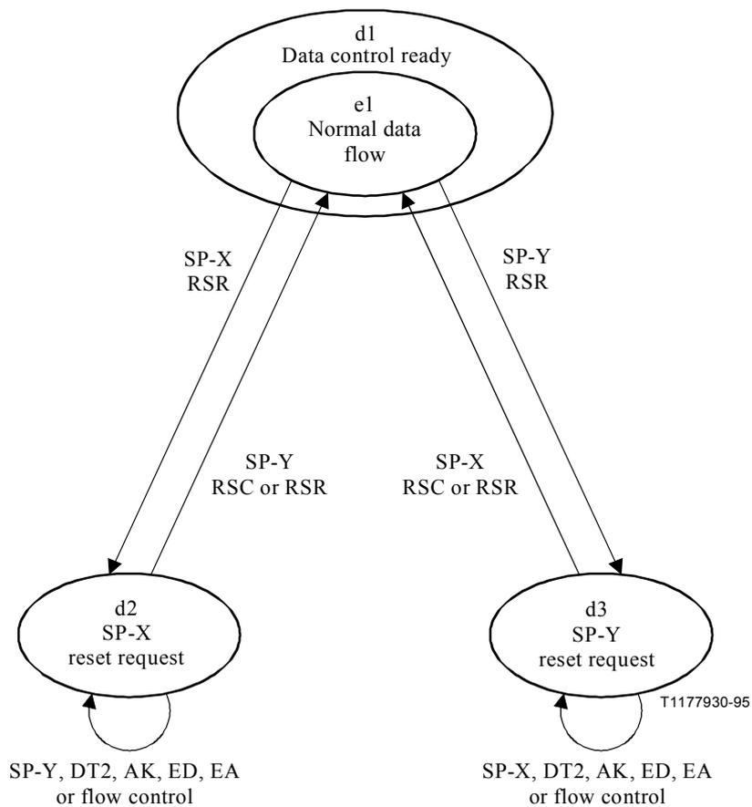
**Figure A.5/Q.714 – State transition diagram for the transfer of reset messages within the data transfer (c4) state**
