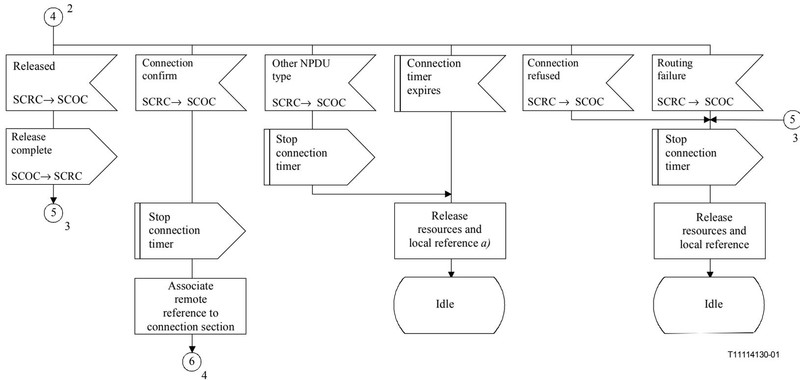
**Figure C.2/Q.714 – Connection establishment procedures at originating node for SCCP connection-oriented control (SCOC) (sheet 3 of 7)**
