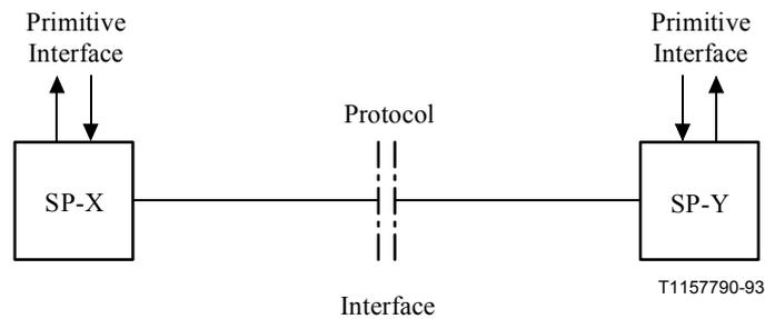
NOTE – SP-X and SP-Y are the signalling points X and Y denoting respectively the origin and destination of the connection section concerned.
