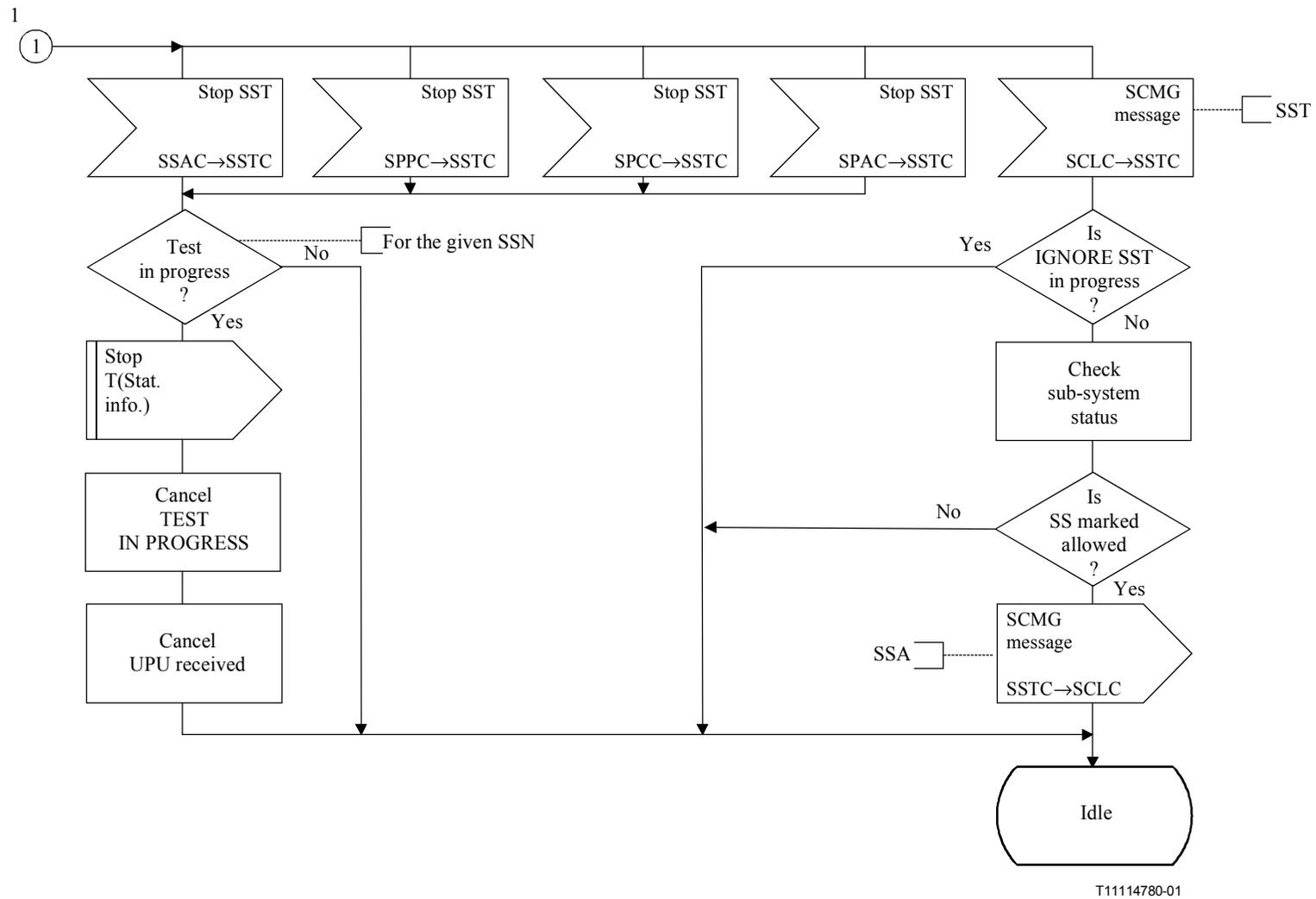
**Figure D.7/Q.714 – Subsystem status test control (SSTC) (sheet 2 of 2)**
