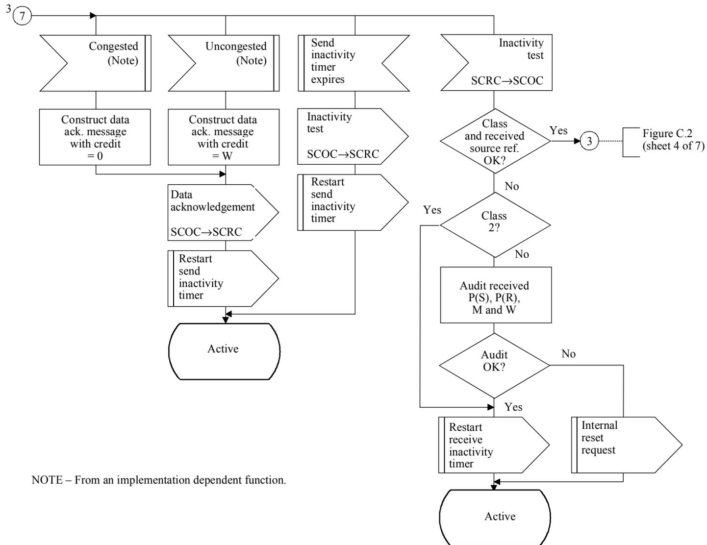
**Figure C.4/Q.714 – Data transfer procedures at originating and destination nodes for SCCP connection-oriented control (SCOC) (sheet 4 of 4)**
