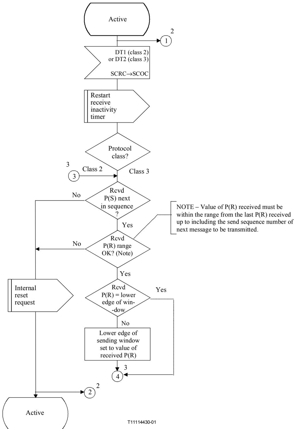
**Figure C.8/Q.714 – Data transfer procedures at relay node with coupling for SCCP connection-oriented control (SCOC) (sheet 1 of 4)**
