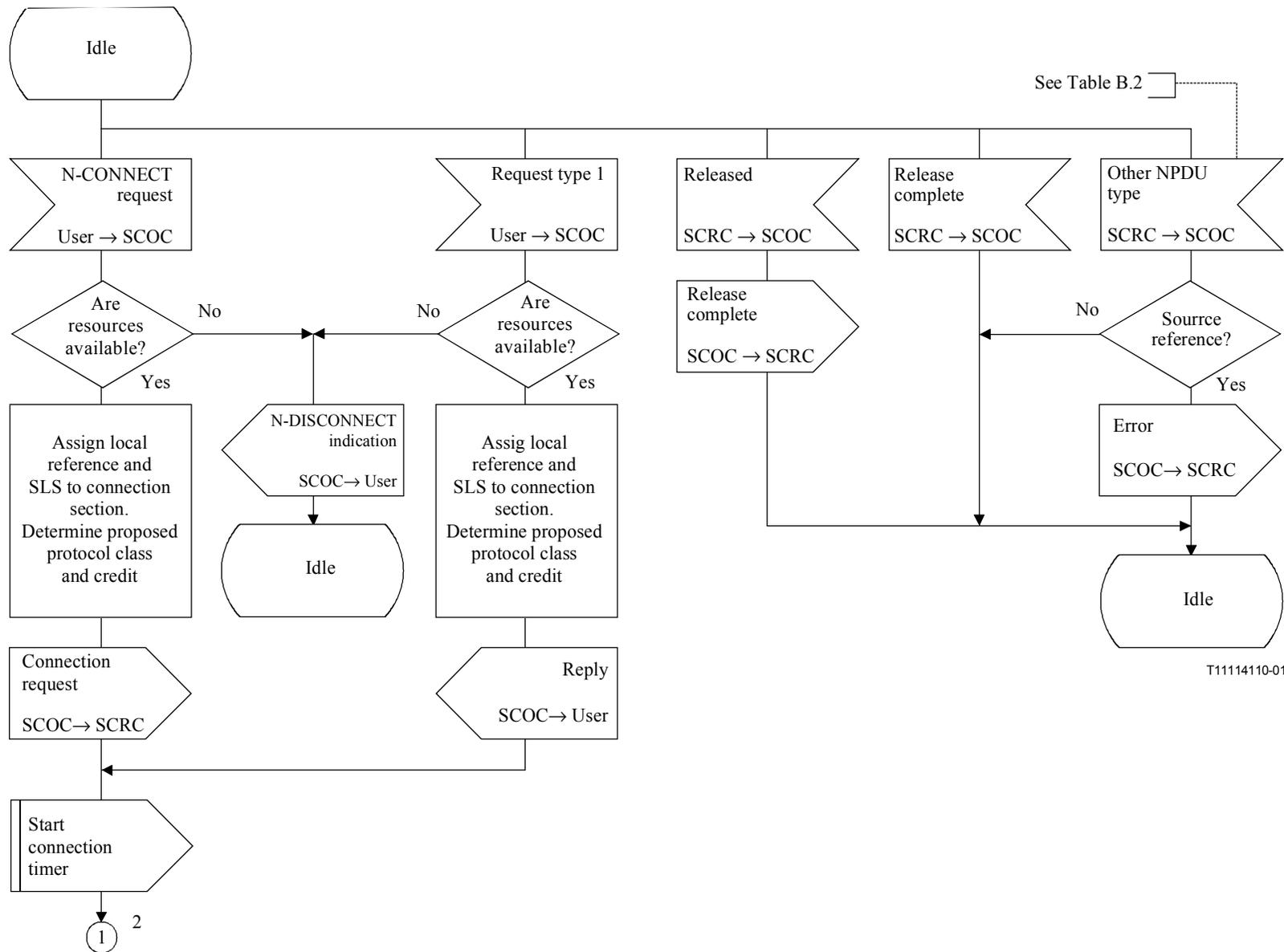
**Figure C.2/Q.714 – Connection establishment procedures at originating node for SCCP connection-oriented control (SCOC) (sheet 1 of 7)**
