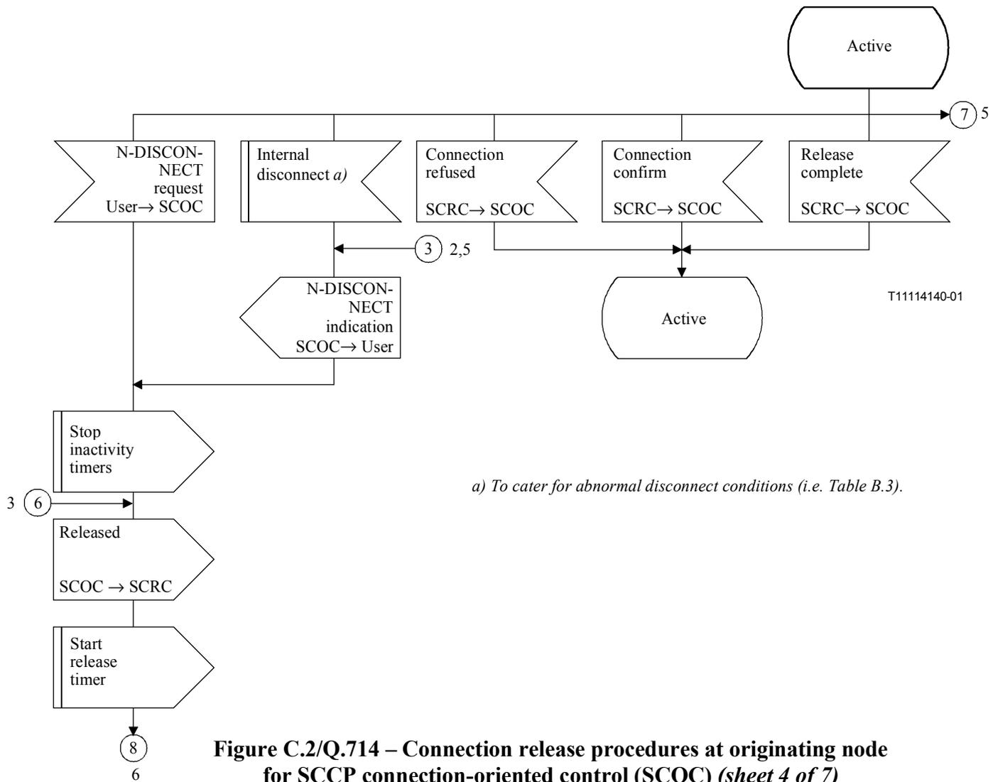
**Figure C.2/Q.714 – Connection release procedures at originating node for SCCP connection-oriented control (SCOC) (sheet 4 of 7)**
