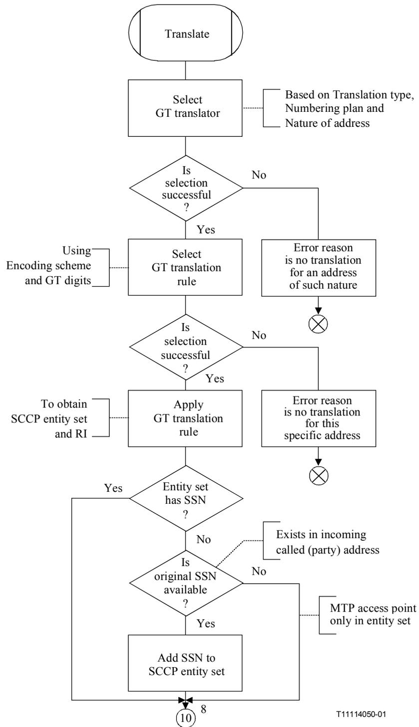
Figure C.1/Q.714 – SCCP routing control procedures (SCRC) (sheet 7 of 12)
