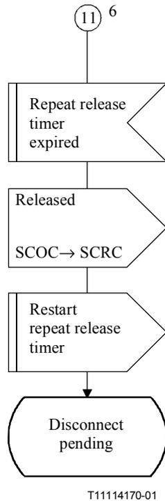
**Figure C.2/Q.714 – Connection release procedures at originating node for SCCP connection-oriented control (SCOC) (sheet 7 of 7)**
