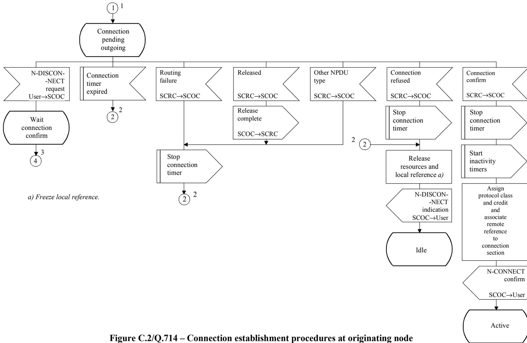
Figure C.2/Q.714 – Connection establishment procedures at originating node for SCCP connection-oriented control (SCOC) (sheet 2 of 7)
