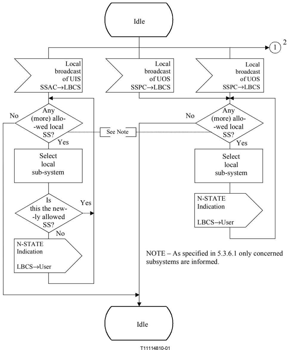
Figure D.9/Q.714 – Local broadcast (LBCS) (sheet 1 of 2)
