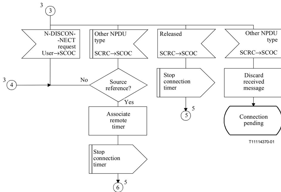
**Figure C.7/Q.714 – Connection establishment procedures at relay node with coupling for SCCP connection-oriented control (SCOC) (sheet 4 of 9)**
