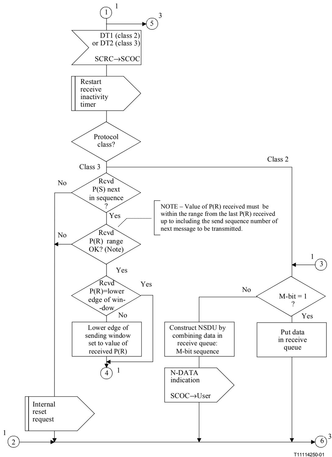
**Figure C.4/Q.714 – Data transfer procedures at originating and destination nodes for SCCP connection-oriented control (SCOC) (sheet 2 of 4)**
