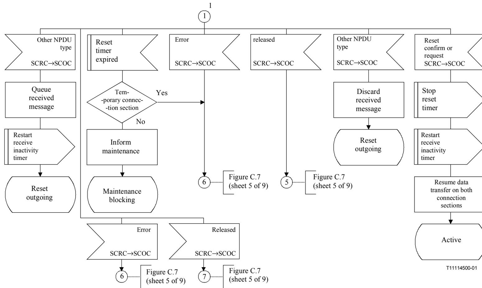
**Figure C.10/Q.714 – Reset procedures at relay node with coupling for SCCP connection-oriented control (SCOC) (sheet 2 of 4)**
