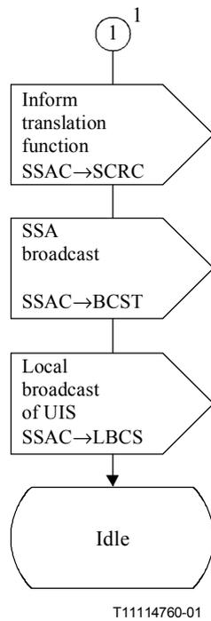
**Figure D.6/Q.714 – Subsystem allowed control (SSAC) (sheet 2 of 2)**
