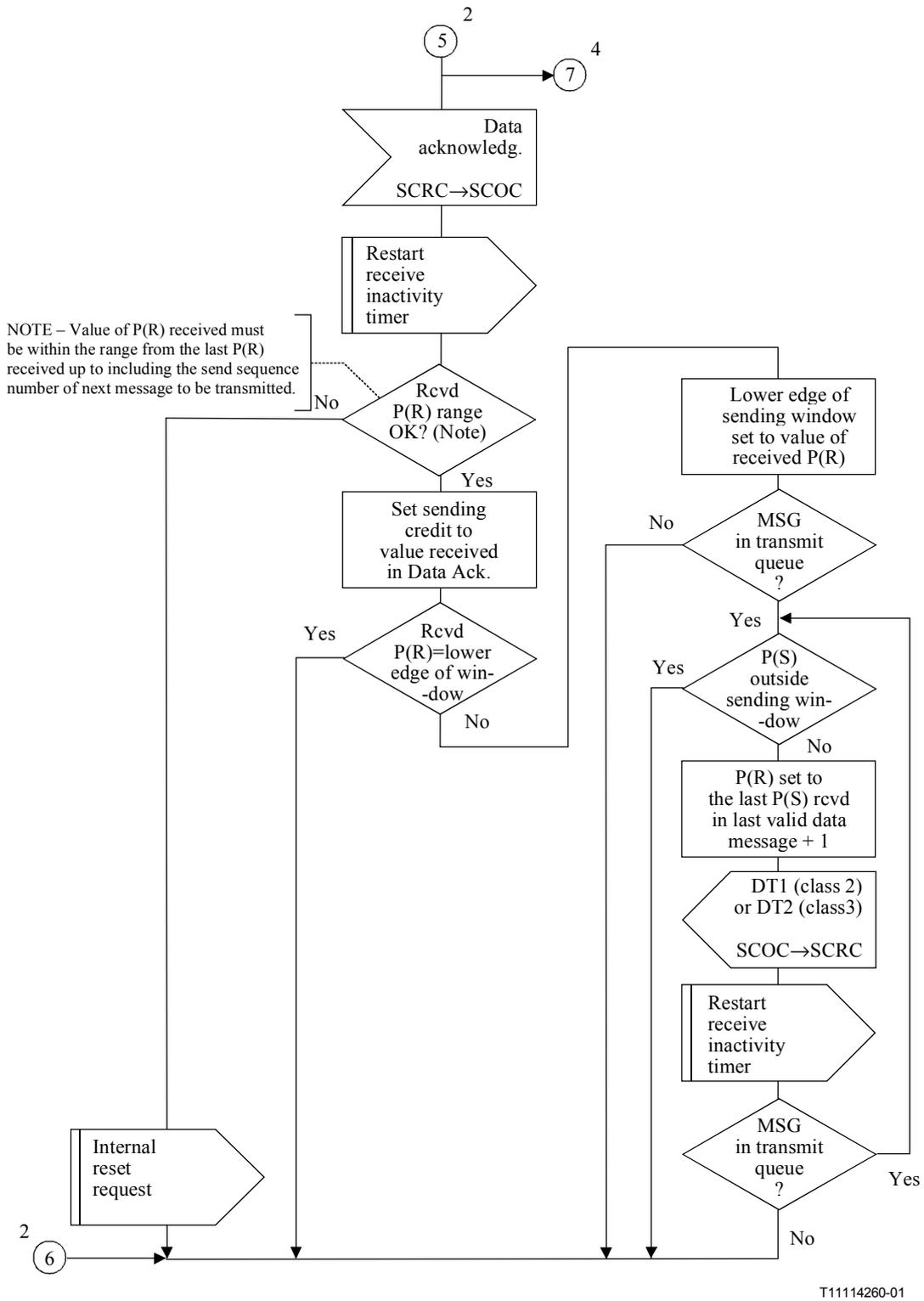
Figure C.4/Q.714 – Data transfer procedures at originating and destination nodes for SCCP connection-oriented control (SCOC) (sheet 3 of 4)
