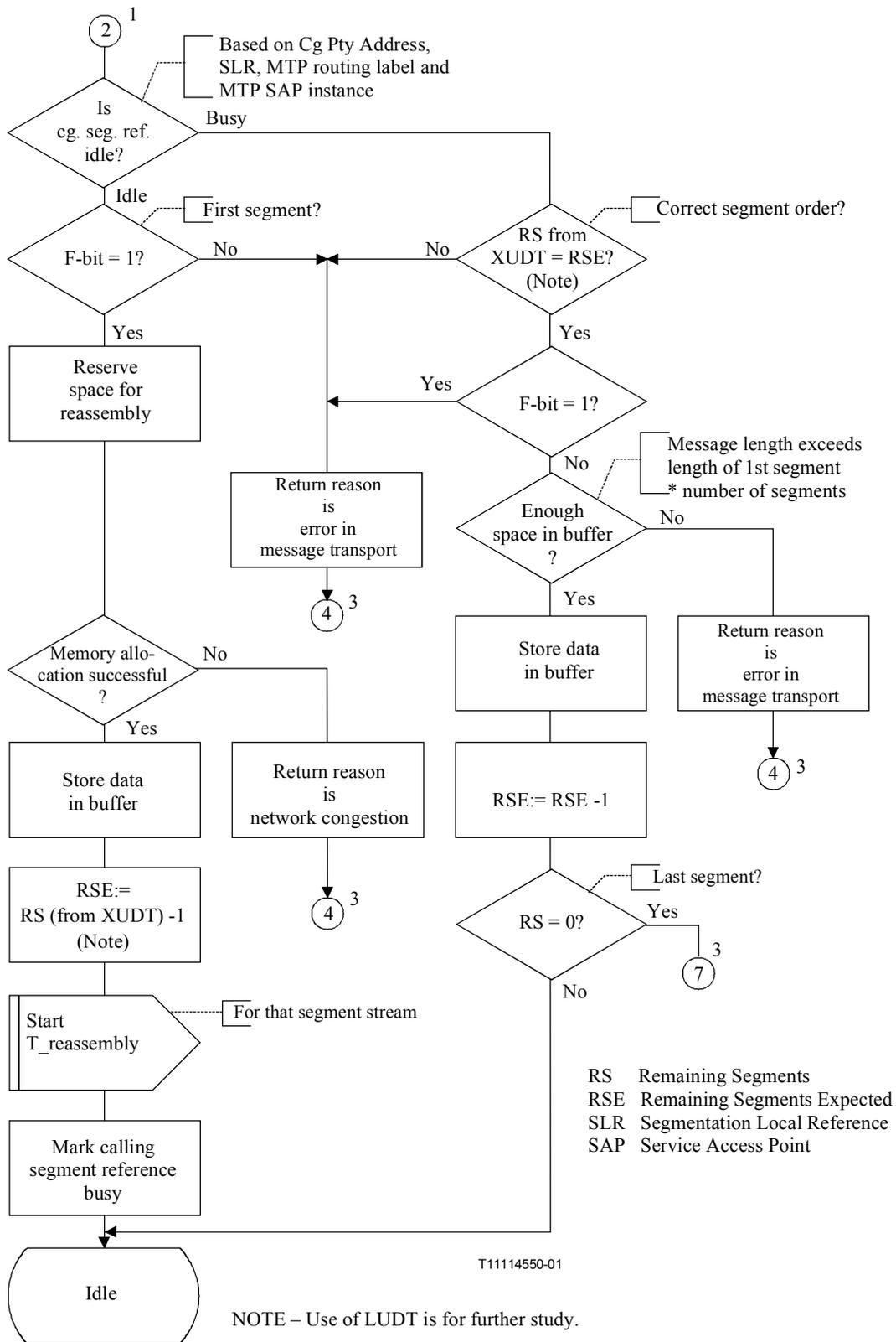
Figure C.12/Q.714 – SCCP connectionless control (SCLC) (sheet 2 of 9)
