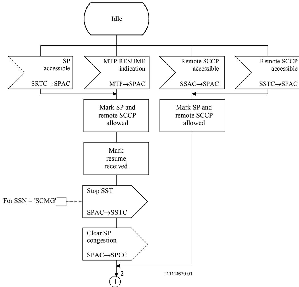
**Figure D.3/Q.714 – Signalling point allowed control (SPAC) (sheet 1 of 2)**
