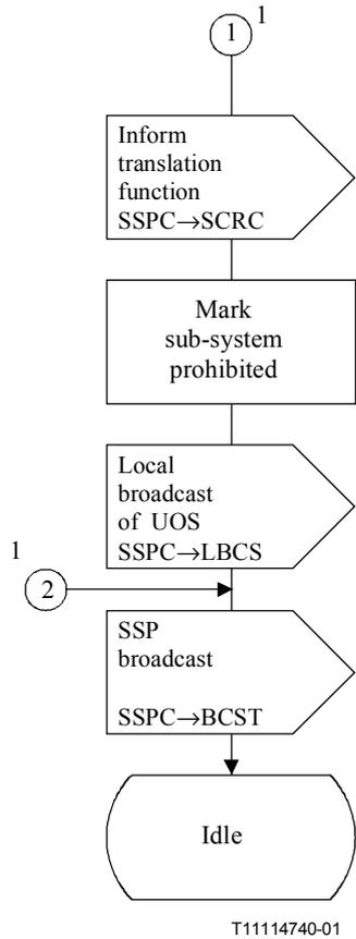
**Figure D.5/Q.714 – Subsystem prohibited control (SSPC) (sheet 2 of 2)**
