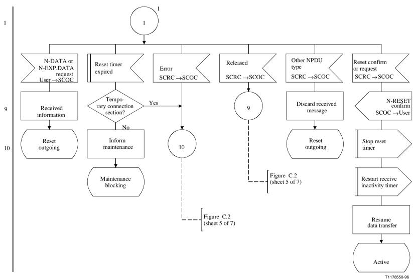
Figure C.6/Q.714 (sheet 2 of 4) – Reset procedures at originating and destination node for SCCP Connection-Oriented Control (SCOC)
