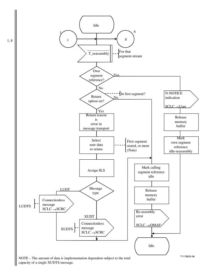
Figure C.12/Q.714 (sheet 5 of 9) – SCCP Connectionless Control (SCLC)
