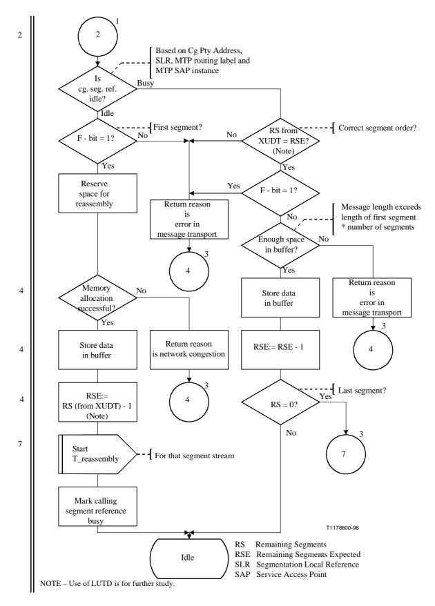
Figure C.12/Q.714 (sheet 2 of 9) – SCCP Connectionless Control (SCLC)
