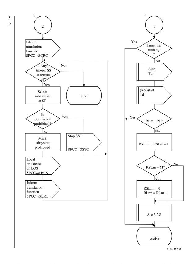
Figure D.4/Q.714 (sheet 3 of 4) – Signalling Point Congested Control (SPCC)
