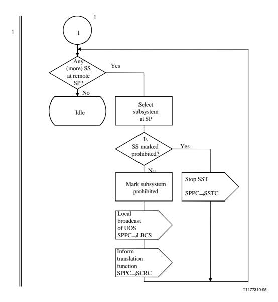
Figure D.2/Q.714 (sheet 2 of 2) – Signalling point prohibited control (SPPC)
