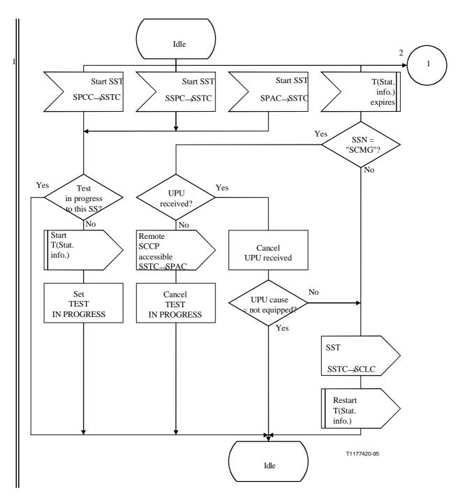
Figure D.7/Q.714 (sheet 1 of 2) – Subsystem Status Test Control (SSTC)
