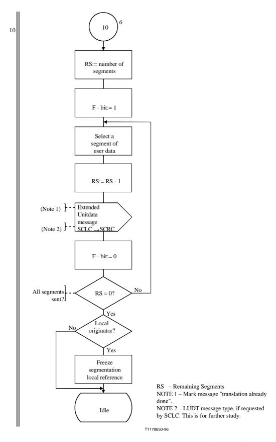
Figure C.12/Q.714 (sheet 7 of 9) – SCCP Connectionless Control (SCLC)
