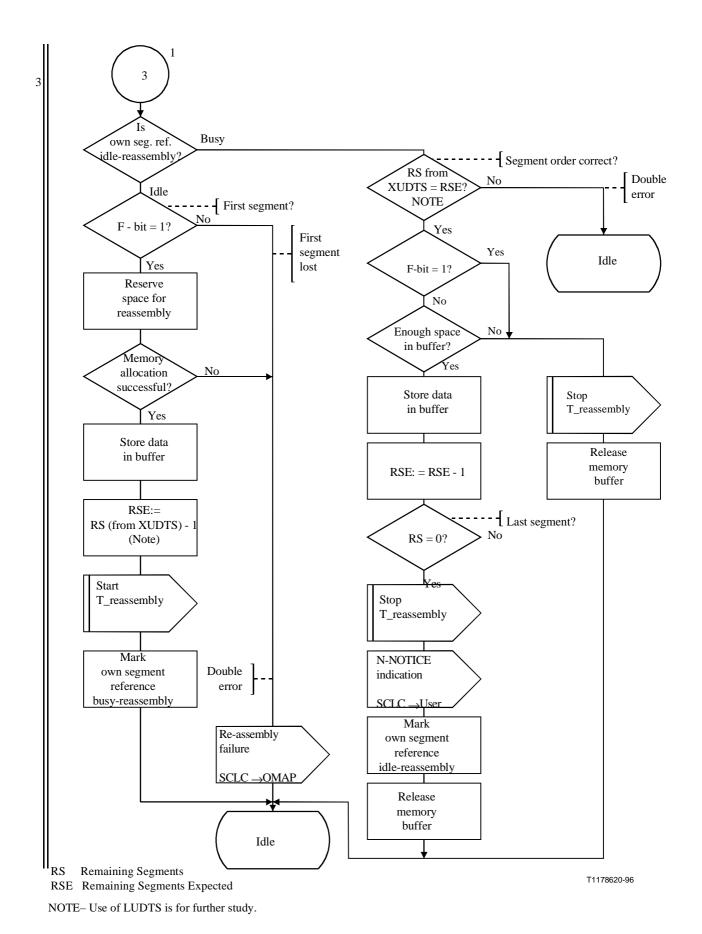
Figure C.12/Q.714 (sheet 4 of 9) – SCCP Connectionless Control (SCLC)
