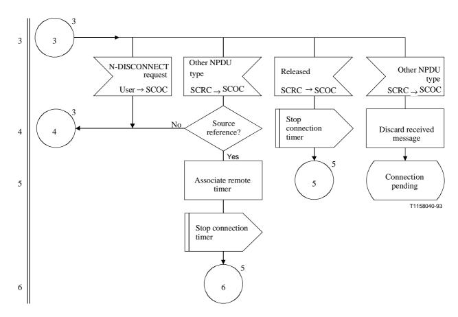
Figure C.7/Q.714/(sheet 4 of 9) – Connection establishment procedures at intermediate node with coupling for SCCP Connection-Oriented Control (SCOC)
