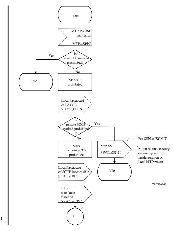
Figure D.2/Q.714 (sheet 1 of 2) – Signalling point prohibited control (SPPC)
