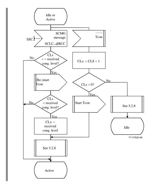
Figure D.13/Q.714 (sheet 1 of 2) – Remote SCCP and nodal congestion control (SRCC)
