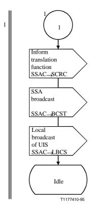
Figure D.6/Q.714 (sheet 2 of 2) – SubSystem Allowed Control (SSAC)
