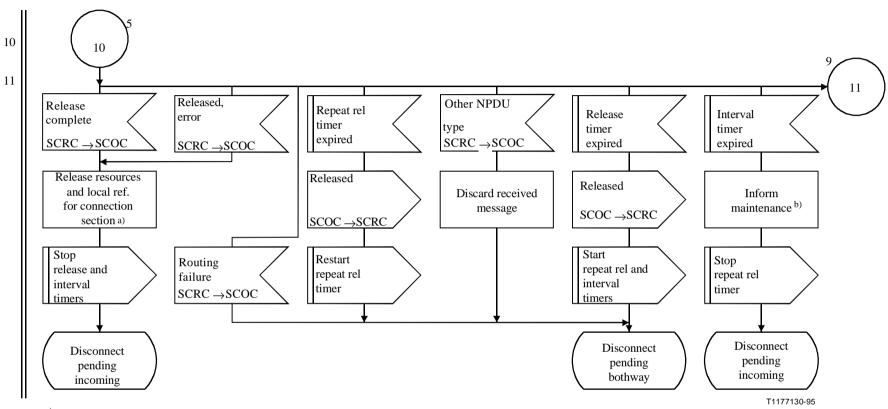
Figure C.7/Q.714 (sheet 8 of 9) – Connection release procedures at intermediate node with coupling for SCCP Connection-Oriented Control (SCOC)
