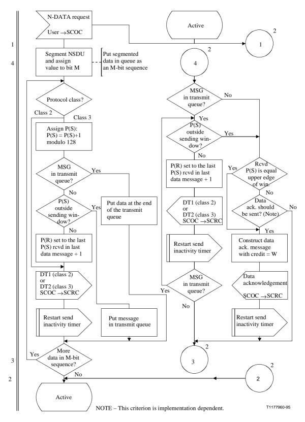
Figure C.4/Q.714 (sheet 1 of 4) – Data transfer procedures at originating and destination nodes for SCCP Connection-Oriented Control (SCOC)
