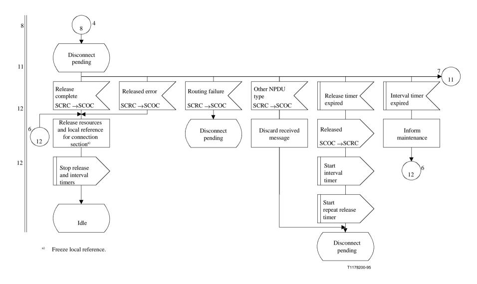
Figure C.2/Q.714 (sheet 6 of 7) – Connection release procedures at originating node for SCCP Connection-Oriented Control (SCOC)
