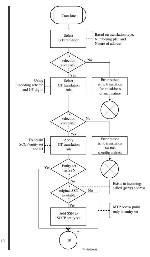
Figure C.1/Q.714 (sheet 6 of 11) – SCCP routing control procedures (SCRC)
