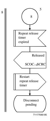
Figure C.3/Q.714 (sheet 6 of 6) – Connection release procedures at destination node for SCCP Connection-Oriented Control (SCOC)
