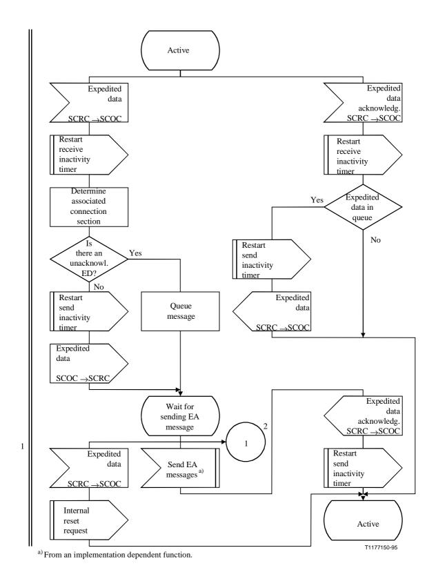
Figure C.9/Q.714 (sheet 1 of 2) – Expedited data transfer procedures at intermediate node with coupling for SCCP Connection-Oriented Control (SCOC)
