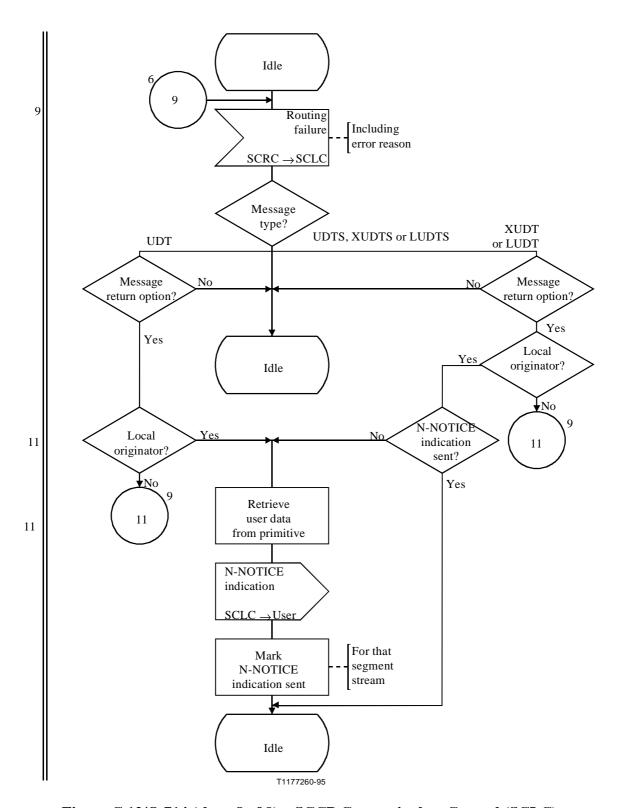
Figure C.12/Q.714 (sheet 8 of 9) – SCCP Connectionless Control (SCLC)
