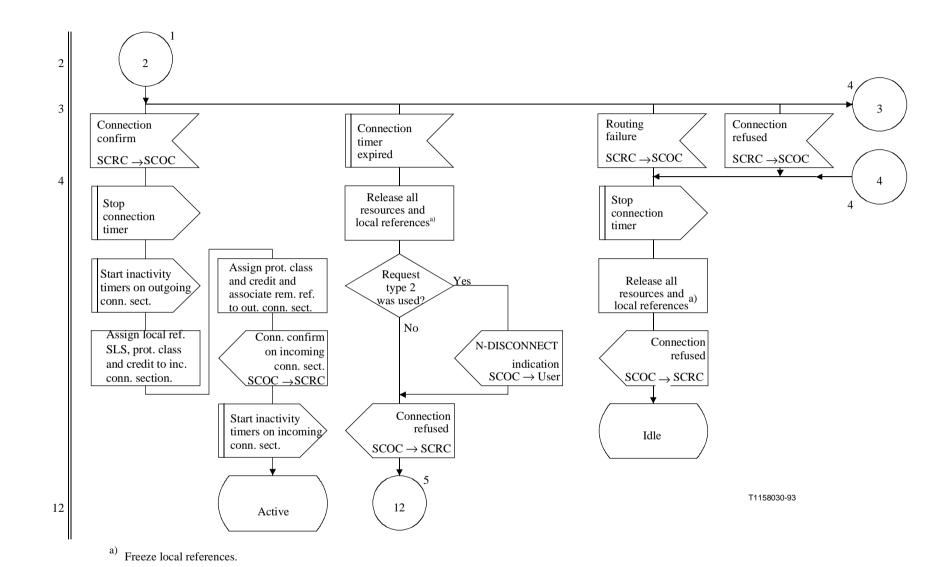
Figure C.7/Q.714 (sheet 3 of 9) – Connection establishment procedures at intermediate node with coupling for SCCP Connection-Oriented Control (SCOC)
