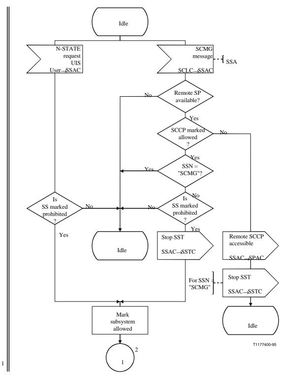
Figure D.6/Q.714 (sheet 1 of 2) – SubSystem Allowed Control (SSAC)
