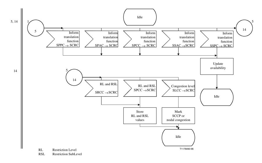
Figure C.1/Q.714 (sheet 5 of 11) – SCCP routing control procedures (SCRC)
