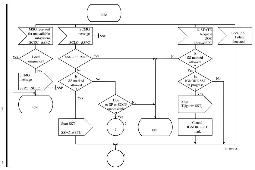
Figure D.5/Q.714 (Sheet 1 of 2) – SubSystem Prohibited Control (SSPC)
