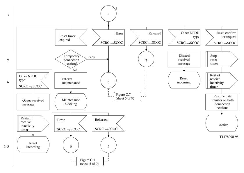
Figure C.10/Q.714 (sheet 4 of 4) – Reset procedures at intermediate node with coupling for **SCCP Connection-Oriented Control (SCOC)**
