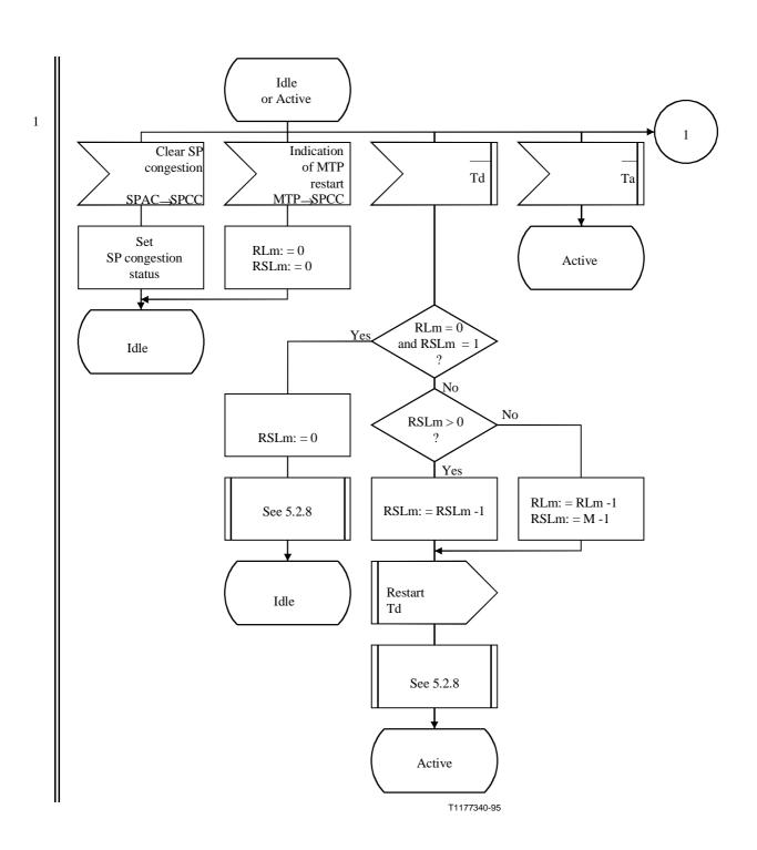
Figure D.4/Q.714 (sheet 1 of 4) – Signalling Point Congested Control (SPCC)
