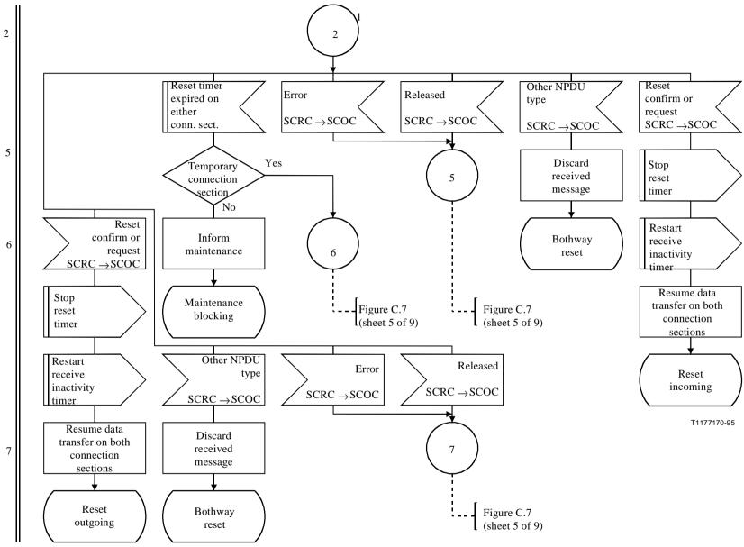
Figure C.10/Q.714 (sheet 3 of 4) – Reset procedures at intermediate node with coupling for SCCP Connection-Oriented Control (SCOC)
