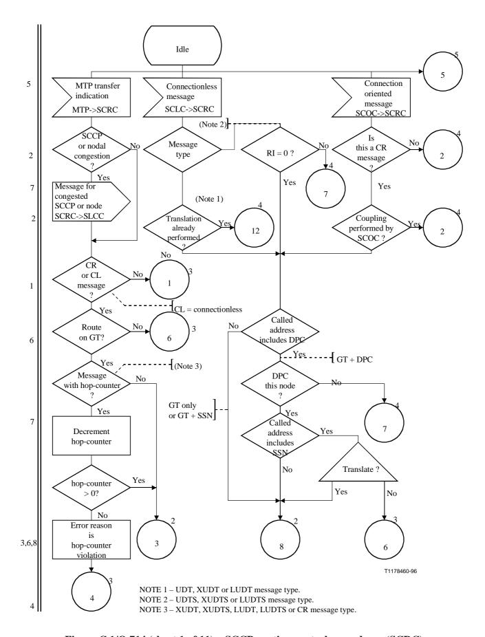
Figure C.1/Q.714 (sheet 1 of 11) – SCCP routing control procedures (SCRC)
