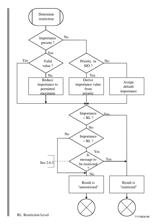
Figure C.1/Q.714 (sheet 11 of 11) – SCCP routing control procedures (SCRC)
