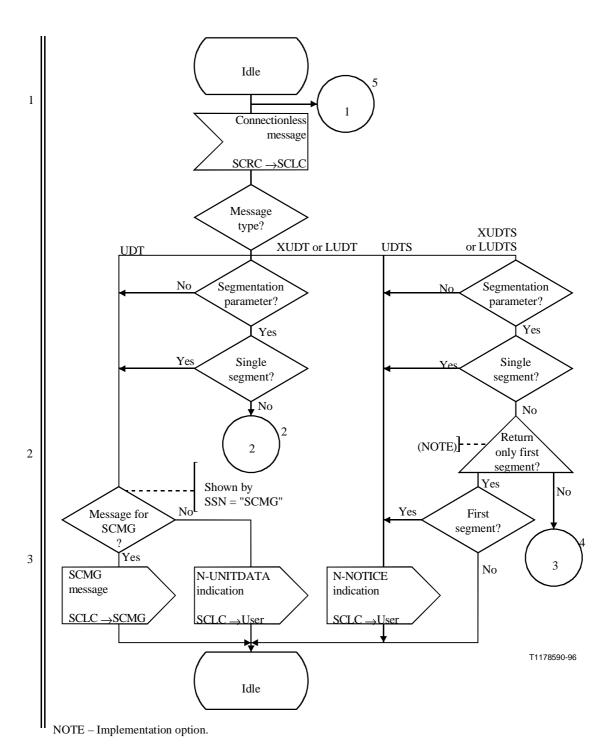
Figure C.12/Q.714 (sheet 1 of 9) – SCCP Connectionless Control (SCLC)
