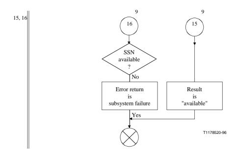
Figure C.1/Q.714 (sheet 10 of 11) – SCCP routing control procedures (SCRC)
