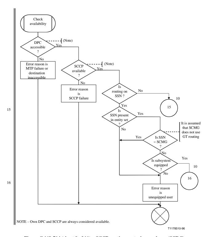
Figure C.1/Q.714 (sheet 9 of 11) – SCCP routing control procedures (SCRC)
