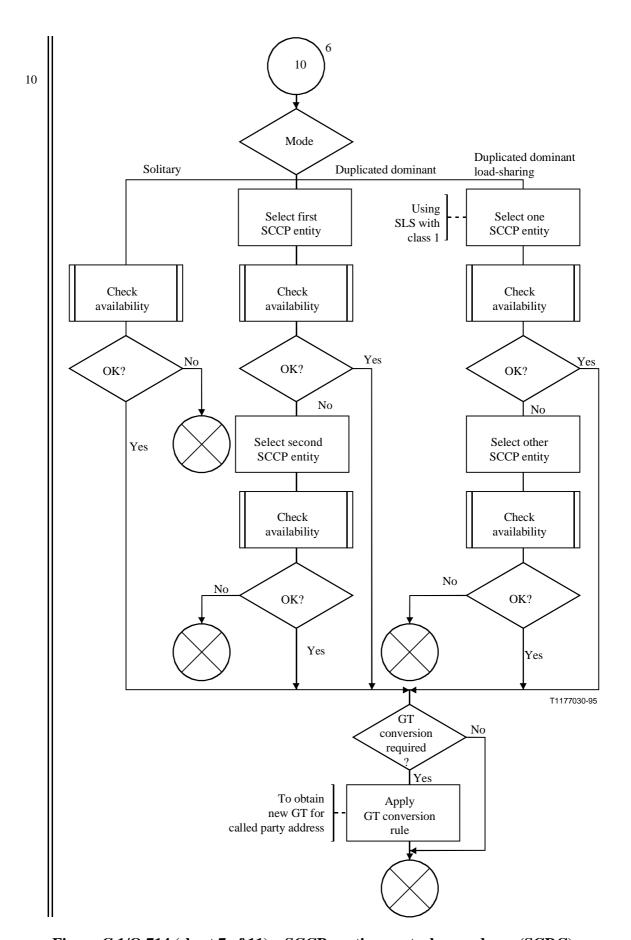
Figure C.1/Q.714 (sheet 7 of 11) – SCCP routing control procedures (SCRC)
