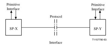
NOTE – SP-X and SP-Y are the signalling points X and Y denoting respectively the origin and destination of the connection section concerned.
