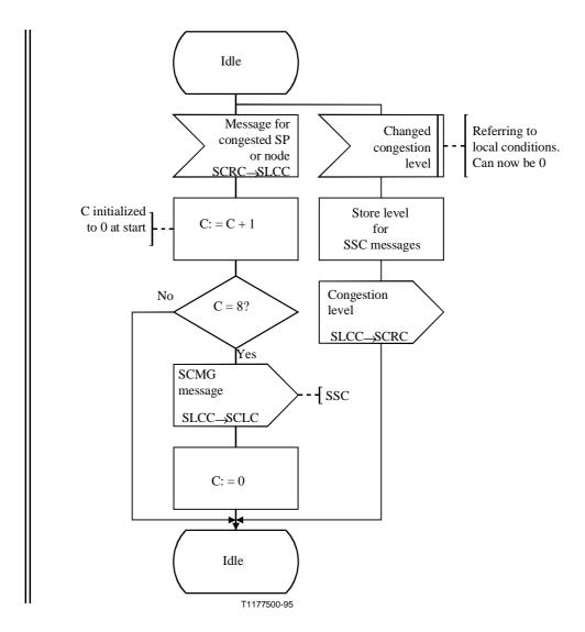
Figure D.12/Q.714 (sheet 1 of 2) – Local SCCP and nodal congestion control (SLCC)
