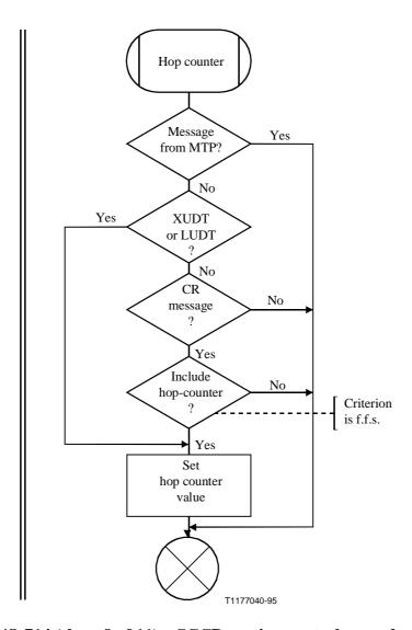
Figure C.1/Q.714 (sheet 8 of 11) – SCCP routing control procedures (SCRC)
