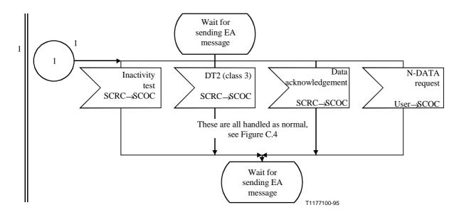
Figure C.5/Q.714 (sheet 2 of 2) – Expedited data transfer procedures at originating and destination node for SCCP Connection-Oriented Control (SCOC)
