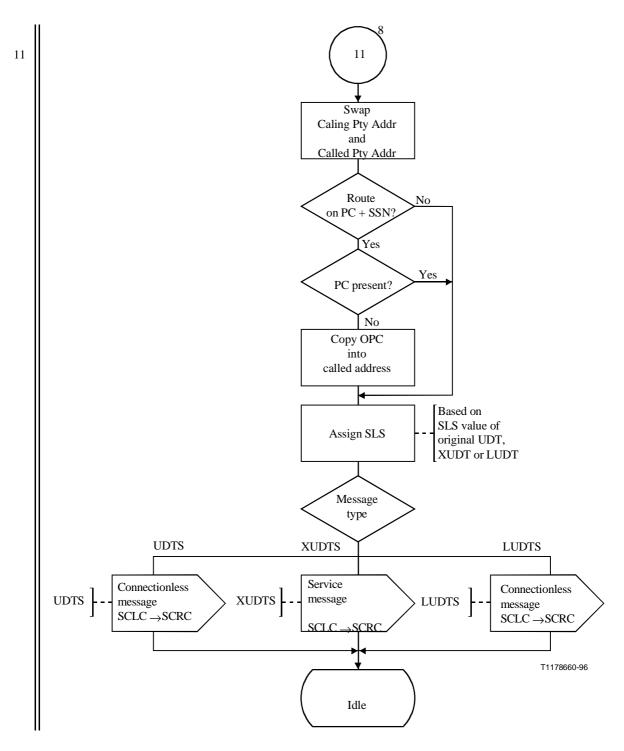
Figure C.12/Q.714 (sheet 9 of 9) – SCCP Connectionless Control (SCLC)
