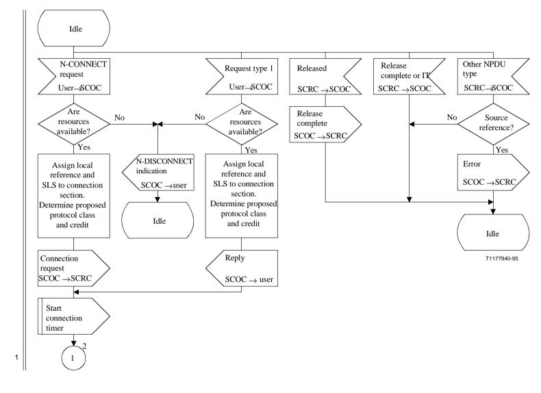
Figure C.2/Q.714 (sheet 1 of 7) – Connection establishment procedures at originating node for SCCP Connection-Oriented Control (SCOC)
