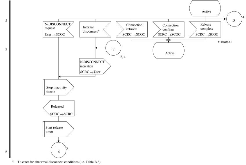
Figure C.3/Q.714 (sheet 3 of 6) – Connection release procedures at destination node for SCCP Connection-Oriented Control (SCOC)
