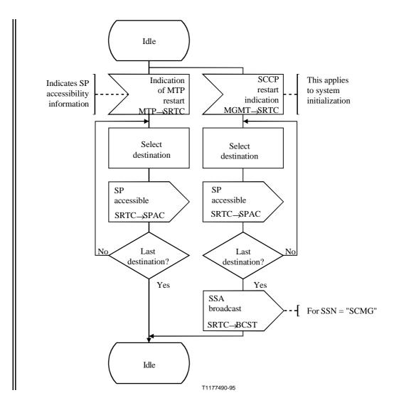
Figure D.11/Q.714 – SCCP restart control (SRTC)
