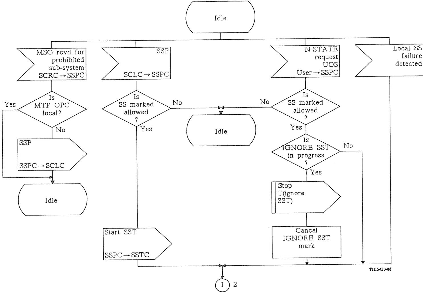
FIGURE D-5/Q.714 (Sheet 1 of 2)
