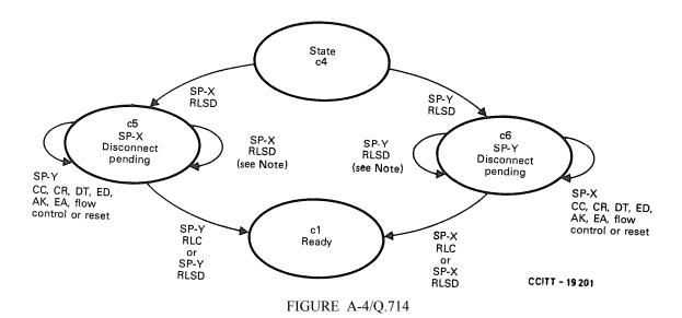
State transition diagram for sequences of messages during connection release
