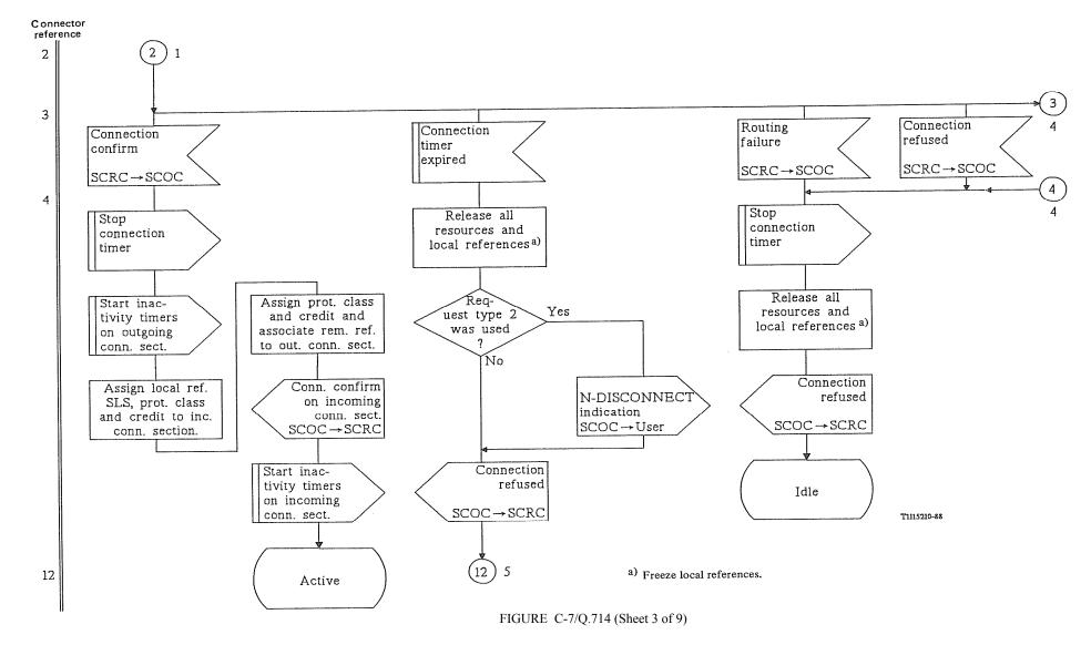
Connection establishment procedures at the intermediate node for SCCP connection-oriented control (SCOC)
