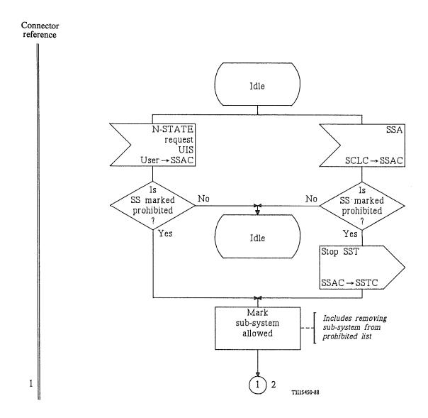
FIGURE D-6/Q.714 (Sheet 1 of 2)
