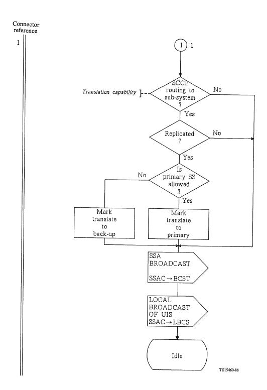
FIGURE D-6/Q.714 (Sheet 2 of 2)
