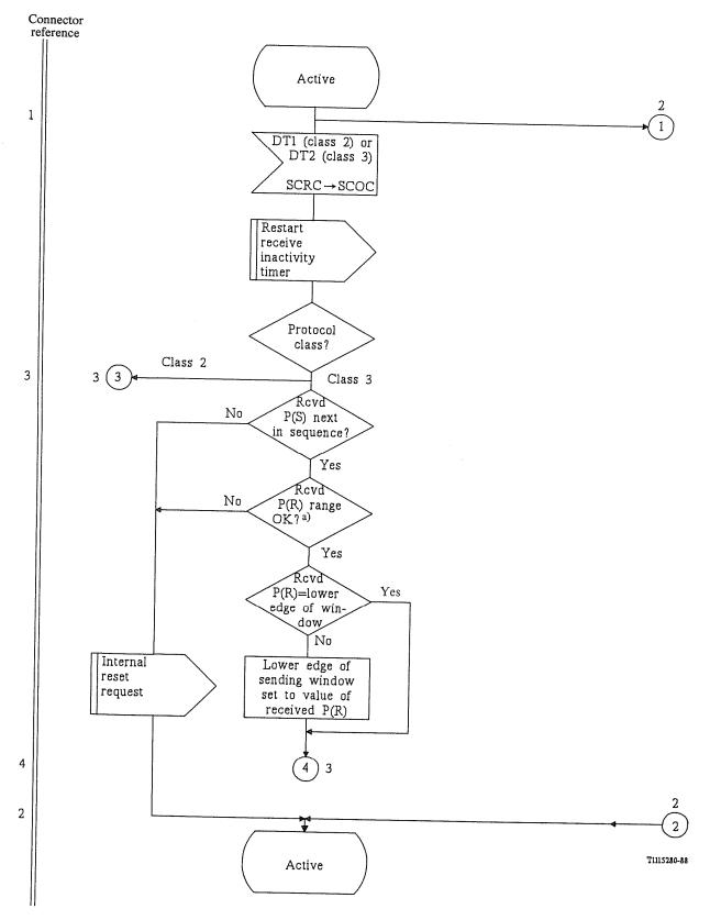
Value of P(R) received must be within the range from the last P(R) received up to including the send sequence number of next message to be transmitted.
