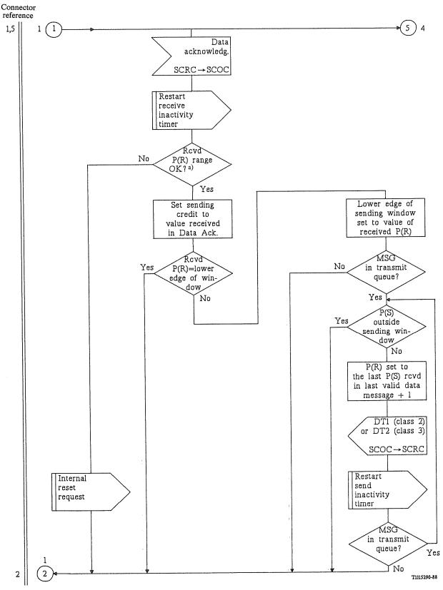
Value of P(R) received must be within the range from the last P(R) received up to including the send sequence number of next message to be transmitted.
