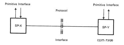
*Note* – SP-X and SP-Y are the signalling points X and Y denoting respectively the origin and destination of the connection section concerned.
