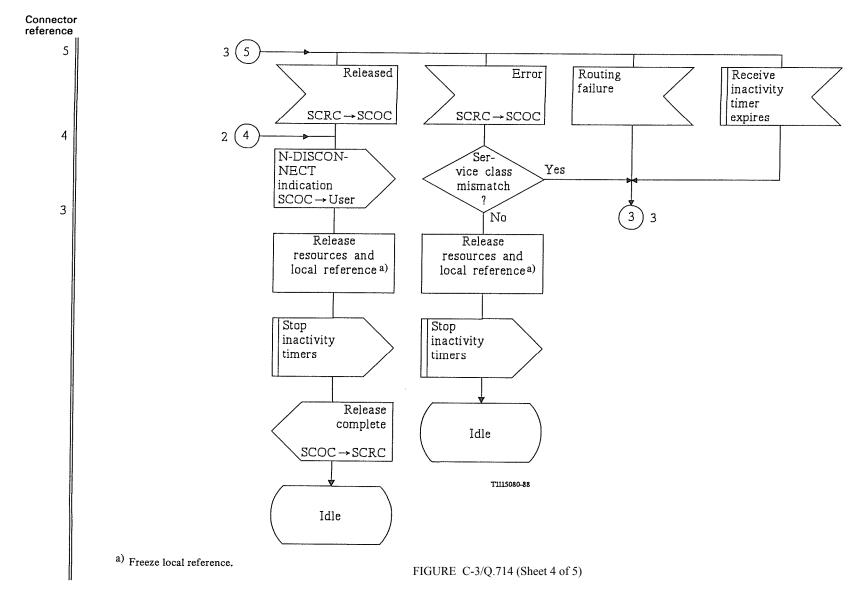
Connection release procedures at destination node for SCCP connection-oriented control (SCOC)
