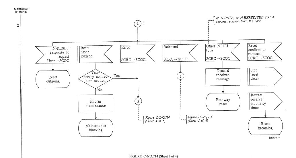
Reset procedures at originating and destination nodes for SCCP connection-oriented control (SCOC)
