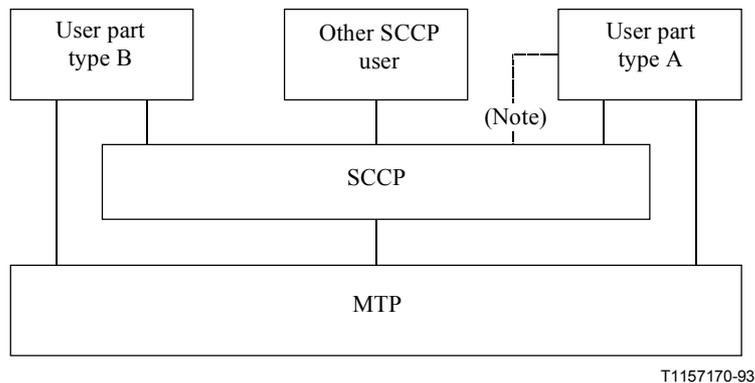
NOTE – Interface using the signals as defined in 6.1.1.3.3, i.e. for the connection-oriented network service.
