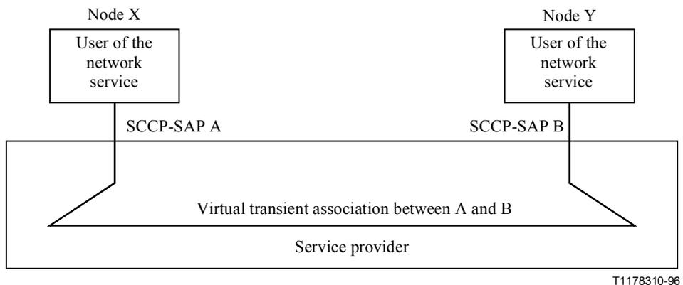
**Figure 5/Q.711 – Model of a network connectionless transmission**
