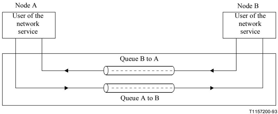
**Figure 4/Q.711 – Model for the internode communication with the SCCP (connection-oriented services)**
