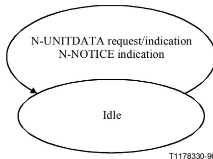
**Figure 9/Q.711 – State transition diagram for sequence of connectionless service primitives at one SCCP-SAP**
