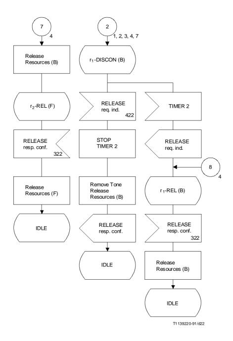
FIGURE 2-14/Q.71 (sheet 5 of 7) CC (FE2)
