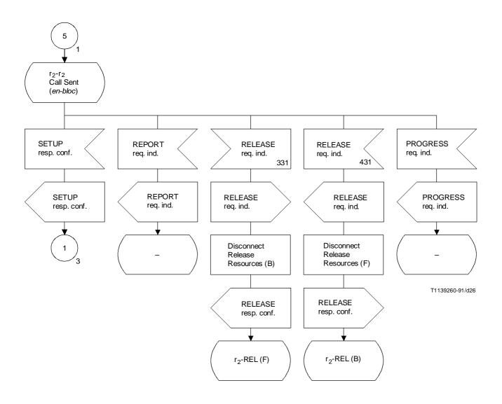
FIGURE 2-15/Q.71 (sheet 2 of 4) **CC (FE3)**
