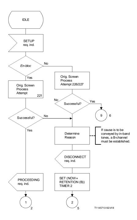
FIGURE 2-14/Q.71 (sheet 1 of 7) CC (FE2)
