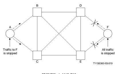
FIGURE A.18/Q.705 Failure of links DF and EF
