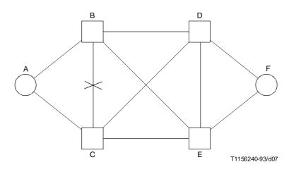
FIGURE A.6/Q.705 Failure of link BC
