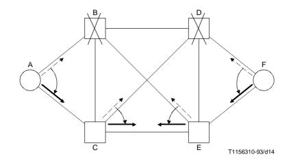
FIGURE A.13/Q.705 Failure of signalling transfer points B and D
