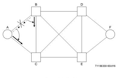
FIGURE A.15/Q.705 Failure of link AB
