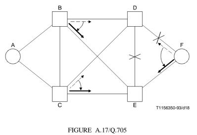
Failure of links DE and DF
