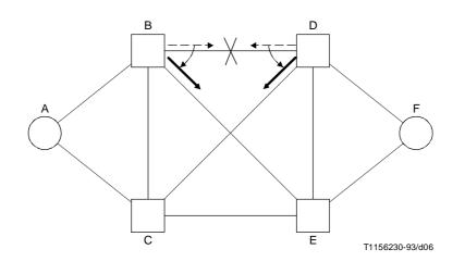
FIGURE A.5/Q.705 Failure of link BD
