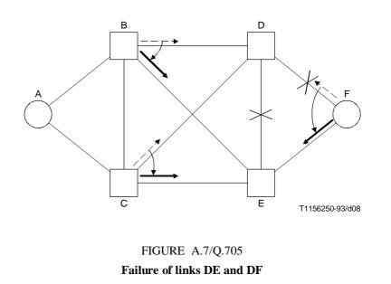
B diverts traffic destined to F from link BD to link BE, because destination F becomes inaccessible via D. It should be noted that only the traffic destined to F is diverted from link BD to link BE, and not all the traffic on link BD. The same applies to C, which diverts traffic destined to F from link CD to link CE. F diverts all the traffic formerly carried by link FD to link FE in the same way as the single link failure example in A.3.3.2.
