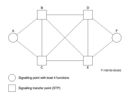
FIGURE A.1/Q.705 Basic mesh network
