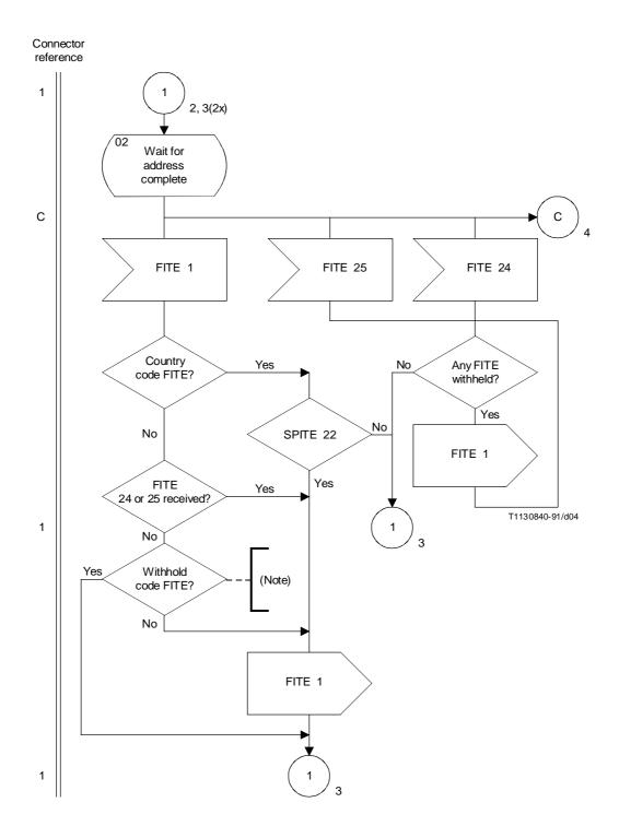
$NOTE-Sufficient\ FITEs\ must\ be\ withheld\ to\ prevent\ an\ address-complete\ signal\ being\ received\ before\ (continuity)\ has\ been\ established\ when\ this\ is\ performed.$
