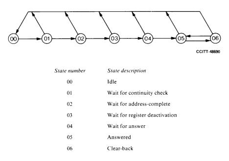
FIGURE 1/Q.654 State overview diagram for interworking of Signalling System No. 6 to R1
