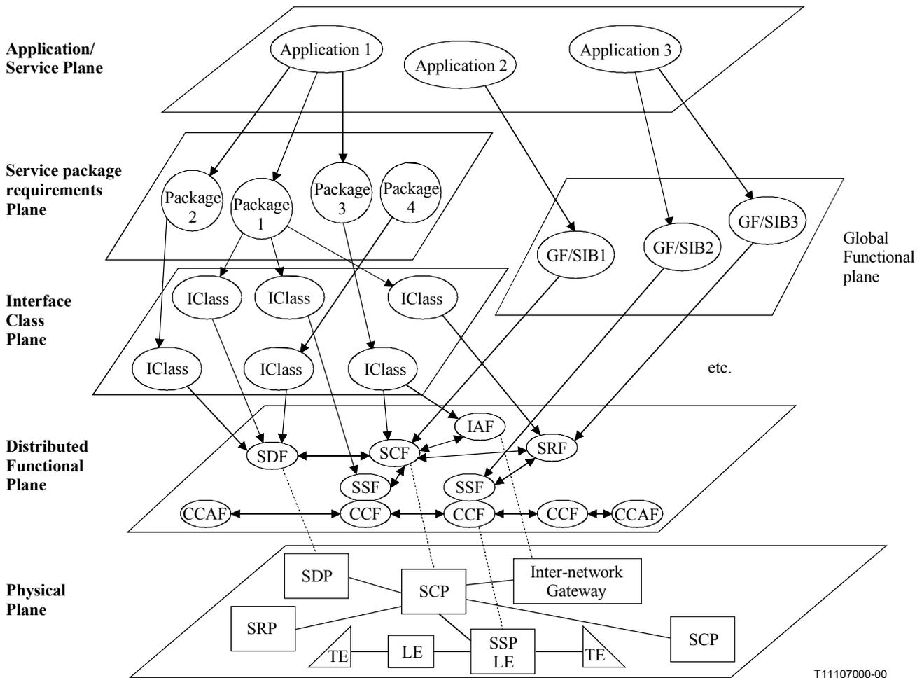
**Figure 1/Q.65 – Conceptual methodology model showing relationships between services, global functions/service-independent building blocks, service packages, interface classes, functional entities and physical entities**
