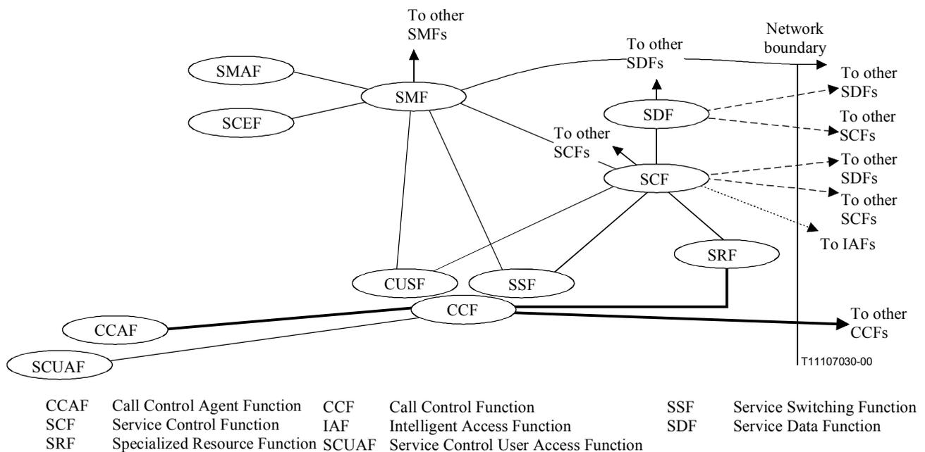
**Figure 3/Q.65 – Unified functional model**
