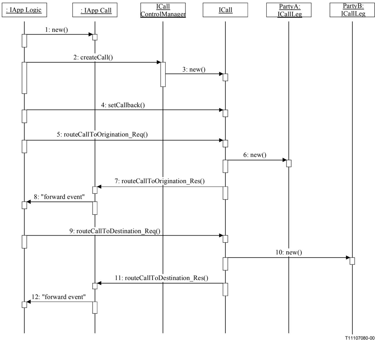
**Figure 25/Q.65 – Example Interface Sequence diagram**
