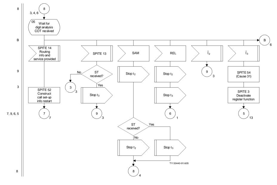
FIGURE 3/Q.617 (sheet 4 of 16) **Incoming Signalling System No. 7 (ISUP)**
