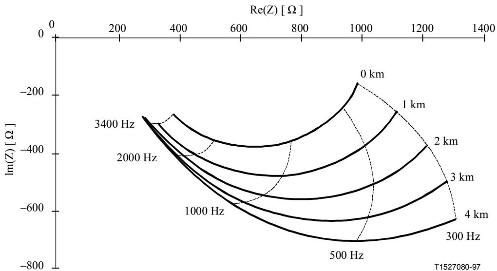
NOTE – The dotted lines connect points of the same frequency but different cable length.
