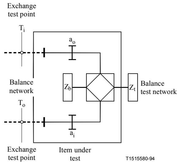
**Figure 9/Q.552 – Arrangement for measuring the loss  $a_{10}$**
