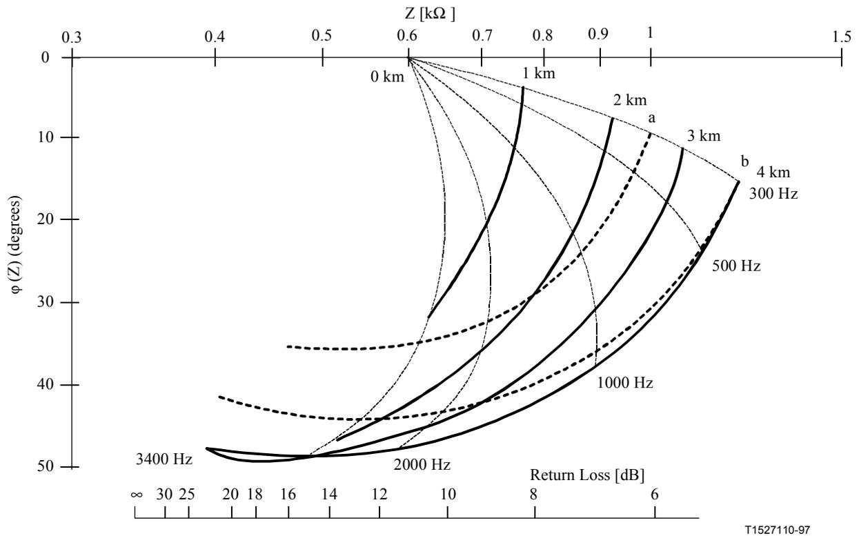
**Figure I.9/Q.552 – Input impedance  $Z_2$  of a 0.5 mm cable with different lengths terminated by  $Z_0 = 600 \Omega$  resistive load in comparison to  $Z_{ETSI}$  (a) and  $Z_{B_{calc}}$  (b)**
