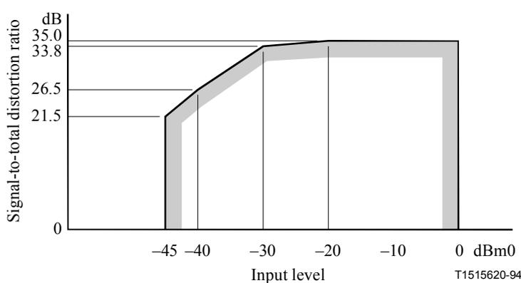
**Figure 13/Q.552 – Limits for signal-to-total distortion ratio as a function of input level; input or output connection with signalling on the speech wires**
