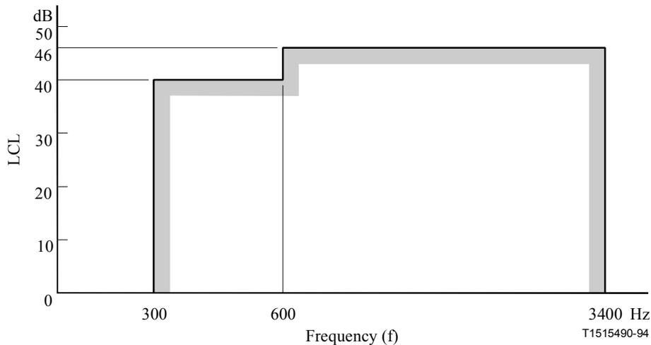
**Figure 2/Q.552 – Minimum values of LCL measured in the arrangement shown in Figure 3**
