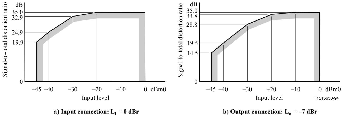
**Figure 14/Q.552 – Limits for signal-to-total distortion ratio as a function of input level including analogue noise**
