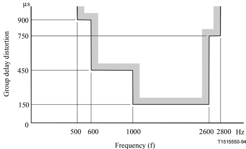
Figure 6/Q.552 – Group delay distortion limits with frequency
