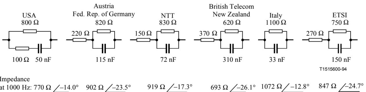
**Figure 11/Q.552 – Examples of test networks to be used by some network operators (applicable to unloaded subscriber lines)**
