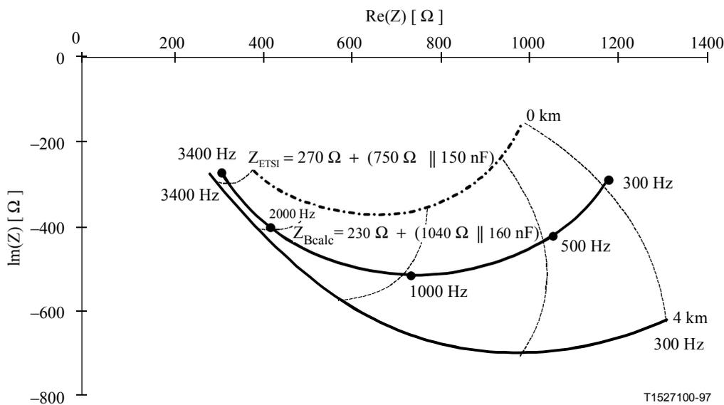
NOTE – The area shown represents the input impedance range of the cable terminated by  $Z_{ETSI}$  (see Figure I.6).
