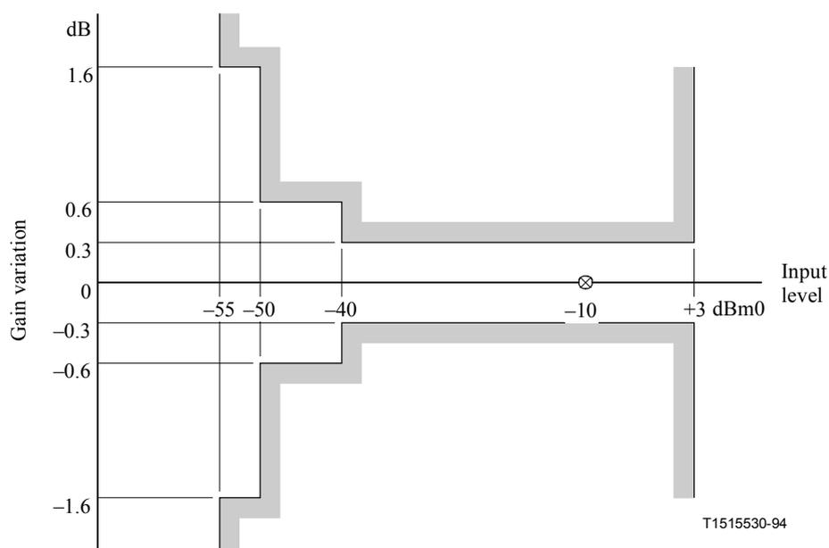
**Figure 4/Q.552 – Variation of gain with input level**
