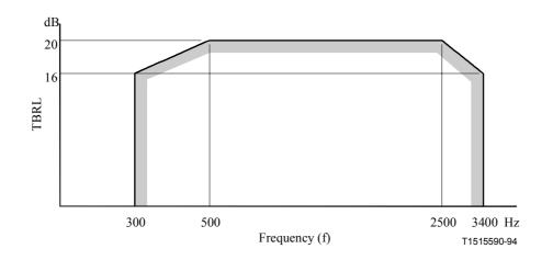
Figure 10/Q.552 – Limits for TBRL
