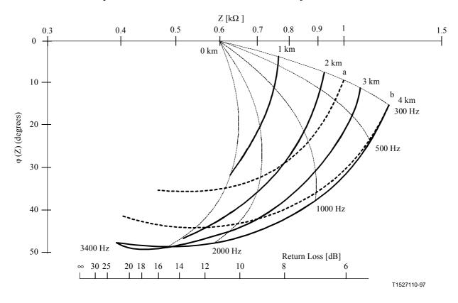
Figure I.9/Q.552 – Input impedance Z<sub>2</sub> of a 0.5 mm cable with different lengths terminated by  $Z_0 = 600 \Omega$  resistive load in comparison to  $Z_{ETSI}$  (a) and  $Z_{B_{calc}}$  (b)
