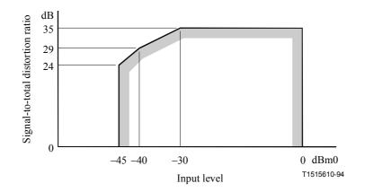
Figure 12/Q.552 – Limits for signal-to-total distortion ratio as a function of input level; input or output connection with signalling on separate wires
