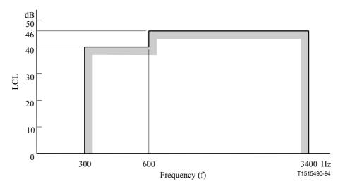
Figure 2/Q.552 – Minimum values of LCL measured in the arrangement shown in Figure 3
