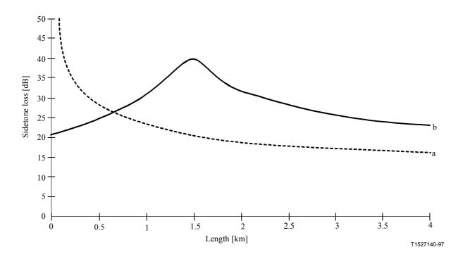
Figure I.12/Q.552 – Sidetone loss for different balance networks in the telephone set
