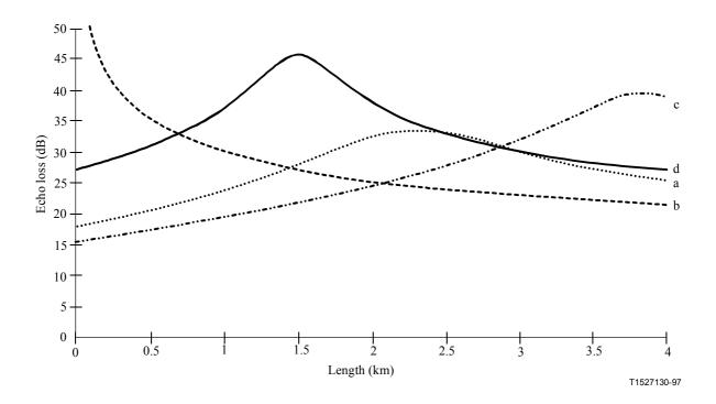
Figure I.11/Q.552 – Echo loss in a network versus different cable length with different hybrid impedances as parameter:
