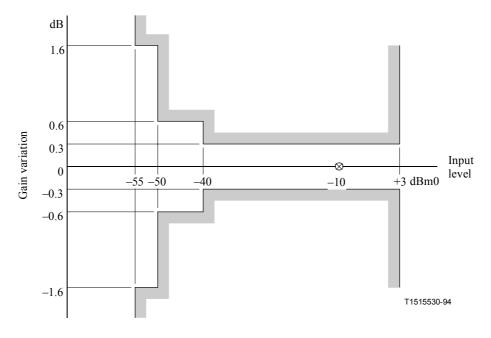
Figure 4/Q.552 – Variation of gain with input level
