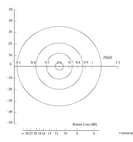
Figure I.4/Q.552 – Constant return loss curves for 10, 15, 20, 30 dB against 600  $\Omega$
