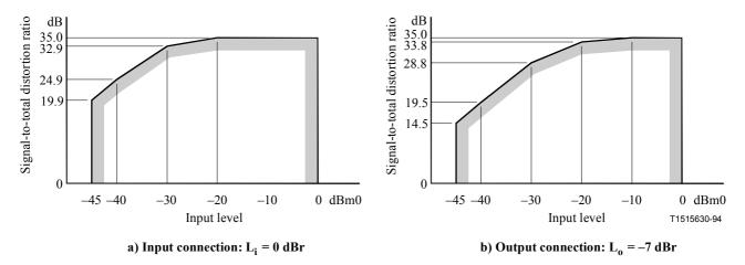
Figure 14/Q.552 – Limits for signal-to-total distortion ratio as a function of input level including analogue noise
