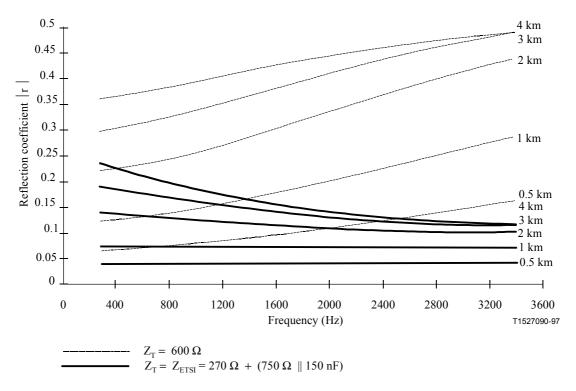
Figure I.7/Q.552 – Reflection coefficient: Impedance  $Z_T$  compared to cable input impedance  $Z_2$  (cable terminated by the impedance  $Z_T$ ) versus frequency
