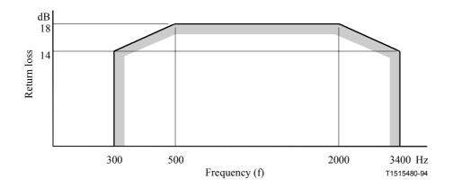
Figure 1/Q.552 – Minimum value of return loss against the test network for the exchange impedance at a 2-wire interface
