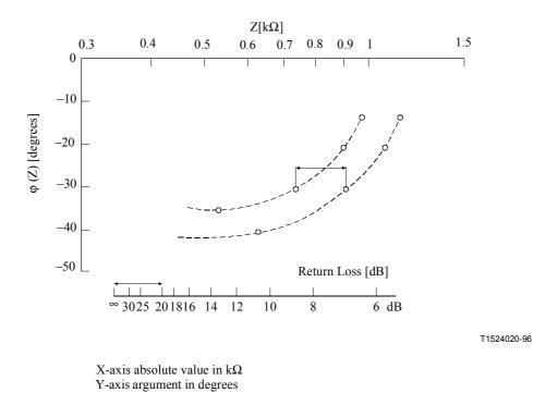
Figure I.3/Q.552 – A special impedance diagram where the return loss between two-impedance points can be read from the "return loss"
