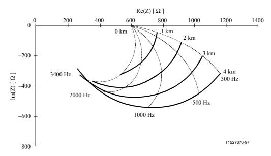
Figure I.5/Q.552 – Input impedance  $Z_2$  of a 0.5 mm cable with different lengths terminated by  $Z_T = 600 \Omega$  resistive load
