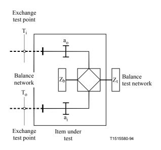
Figure 9/Q.552 – Arrangement for measuring the loss aio
