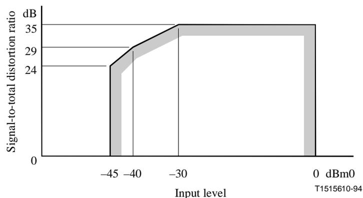
**Figure 12/Q.552 – Limits for signal-to-total distortion ratio as a function of input level; input or output connection with signalling on separate wires**
