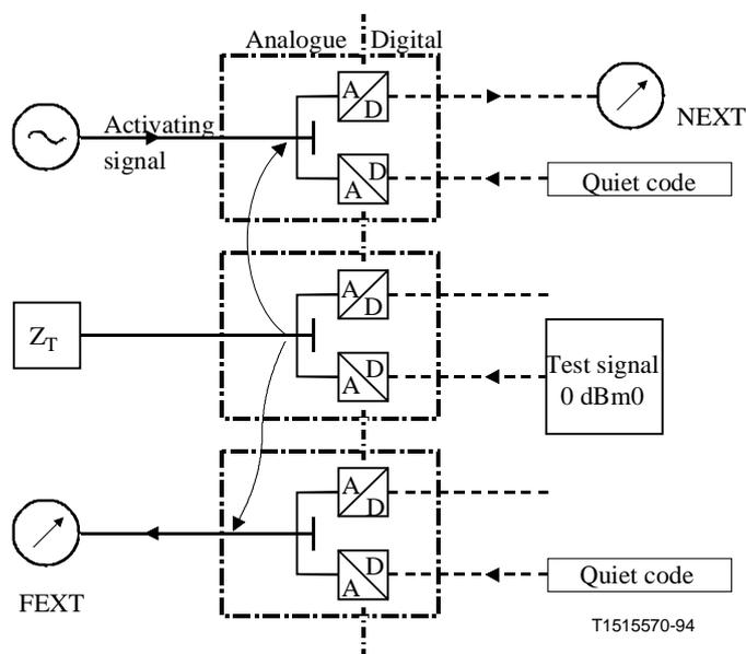
Figure 8/Q.552 – FEXT and NEXT measurements with digital test signal
