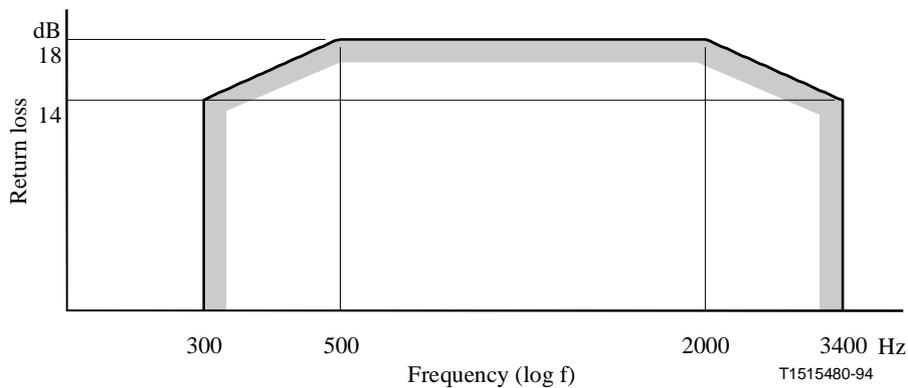
**Figure 1/Q.552 – Minimum value of return loss against the test network for the exchange impedance at a 2-wire interface**
