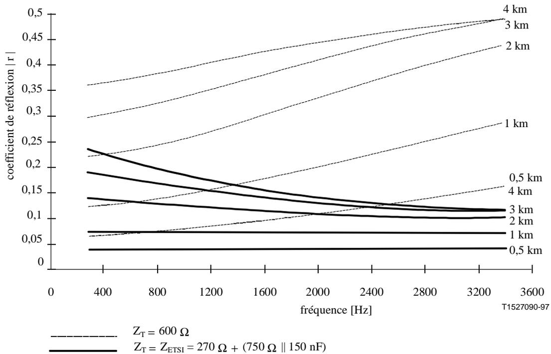
**Figure I.7/Q.552 – Reflection coefficient: Impedance  $Z_T$  compared to cable input impedance  $Z_2$  (cable terminated by the impedance  $Z_T$ ) versus frequency**
