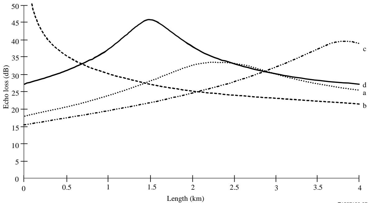
**Figure I.11/Q.552 – Echo loss in a network versus different cable length with different hybrid impedances as parameter;**
