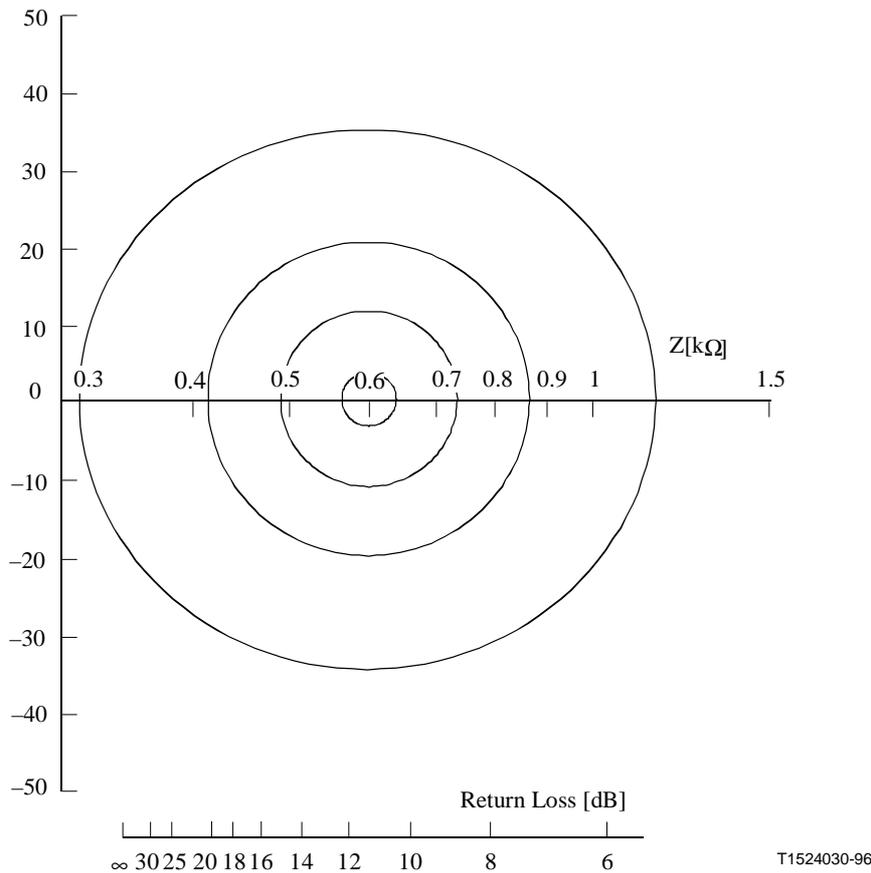
**Figure I.4/Q.552 – Constant return loss curves for 10, 15, 20, 30 dB against 600 Ω**
