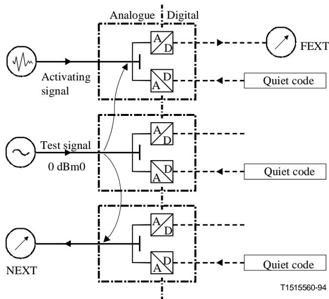
Figure 7/Q.552 – FEXT and NEXT measurements with analogue test signal
