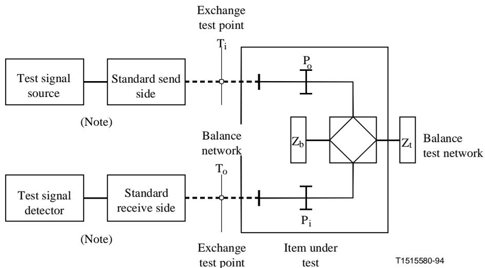
NOTE – This equipment may be all digital, with equivalent functions (see Recommendation O.133). The test signal source and the test signal detector may be as shown in Figure A.1/G.122.
