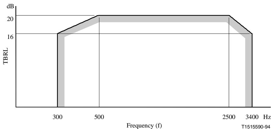
**Figure 10/Q.552 – Limits for TBRL**
