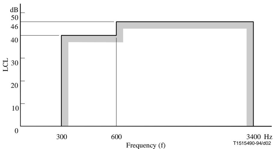
**Figure 2/Q.552 – Minimum values of LCL measured in the arrangement shown in Figure 3/Q.552**
