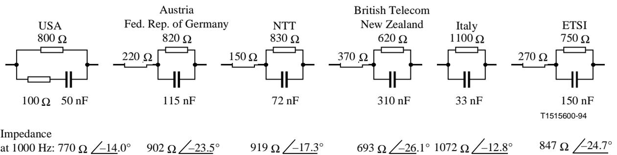
**Figure 11/Q.552 – Examples of test networks to be used by some Administrations
