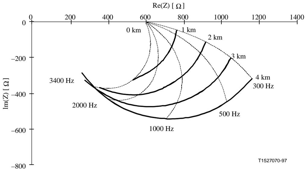
**Figure I.5/Q.552 – Input impedance  $Z_2$  of a 0.5 mm cable with different lengths terminated by  $Z_T = 600 \Omega$  resistive load**
