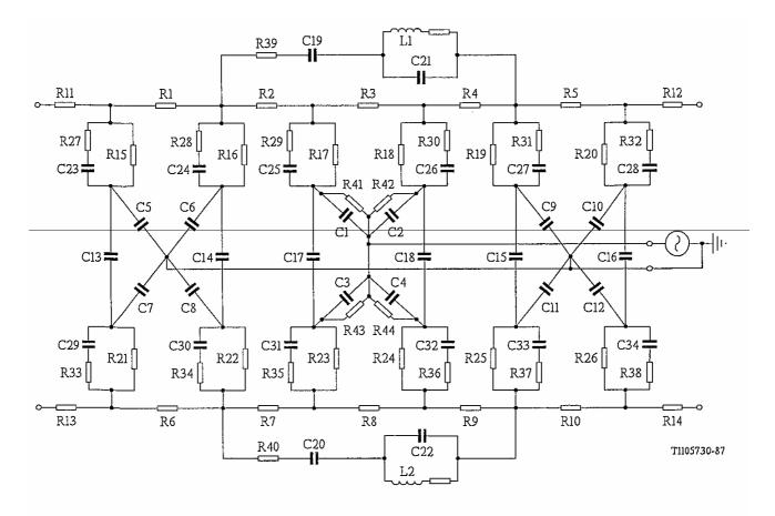
Note - The component values given in Table A-1/Q.552 are applicable to 4 km of 0.4 mm cable with a mutual capacitance of 47 nF/km and a capacitance to earth of 15 nF/km.
