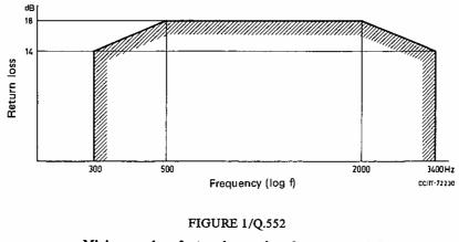
Minimum value of return loss against the test network for the exchange impedance at a 2-wire interface
