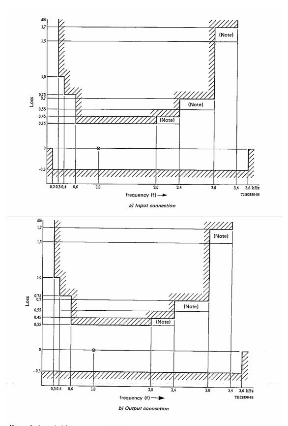
Note — In the marked frequency ranges relaxed limits are shown which apply if the maximum lengths of in-station cabling is used. The more stringent limits shown apply if no such cabling is present.
