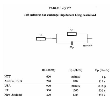
*Note* 1 – The test network and the component values represent a configuration that exhibits the required exchange impedance. It need not necessarily correspond to any actual network provided in the exchange interface.
