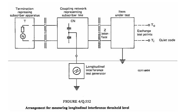
The longitudinal interference test generator should provide the longitudinal interference EMF with the fundamental frequency of the interference source (as appropriate to national conditions, i.e. 16 2/3 Hz, 50 Hz or 60 Hz) with a sinusoidal waveshape, and additionally with a waveshape having a certain amount of harmonic content<sup>1</sup>, e.g. a triangular waveshape.
