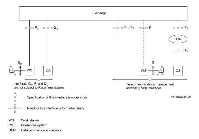
NOTE - An exchange is an example of a network element (NE) as defined in Recommendation M.30.
