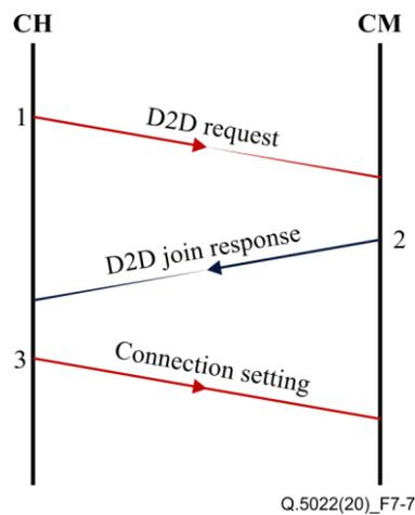
**Figure 7-7 – Signalling diagram for minor discovery stage**
