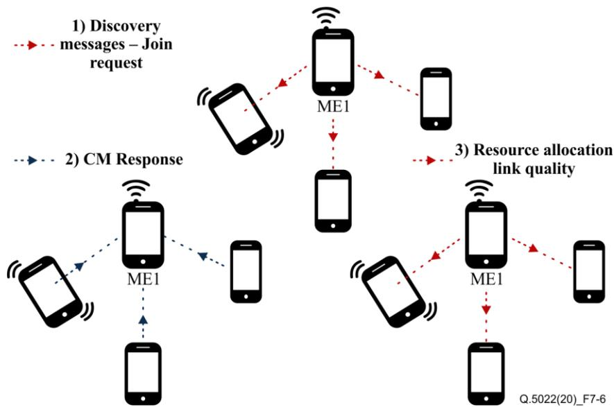
**Figure 7-6 – Minor discovery signalling steps**
