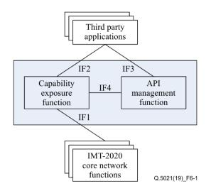
Figure 6-1 – Architecture of capability exposure API management system
