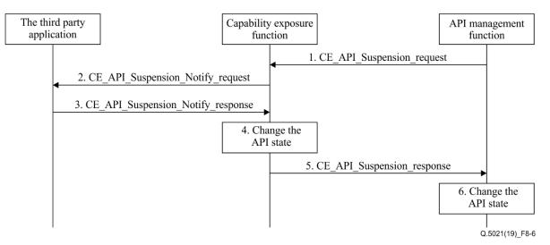
Figure 8-6 – API suspension procedure
