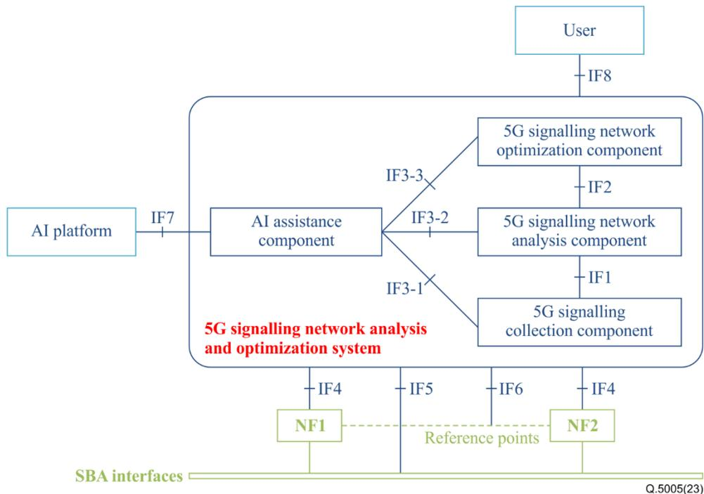
**Figure 8-1 – Framework of IMT-2020 signalling network analysis and optimization**
