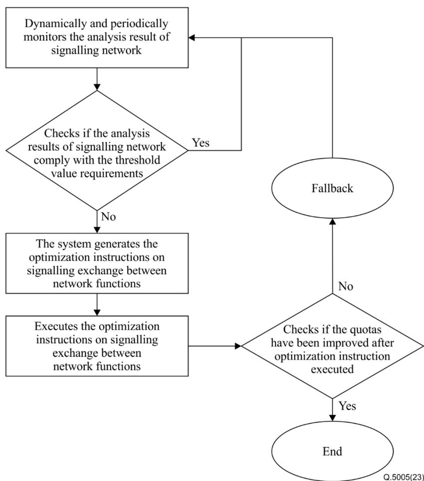
**Figure 10-2 – The process of optimization of signalling exchange between network functions**
