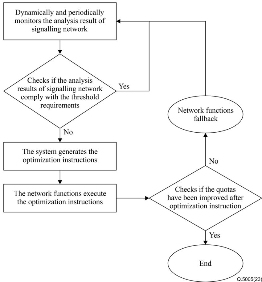
**Figure 10-1 – The process of signalling network optimization on network functions**
