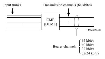
Figure 1/Q.50 – Circuit Multiplication Equipment gain
