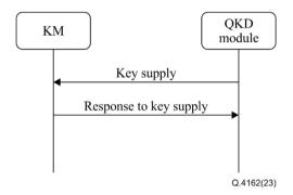
Figure 1 – Signalling procedures for proactive key supply mode at the Kq-1 interface
