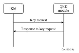
Figure 2 – Signalling procedures for key supply upon request mode at the Kq-1 interface
