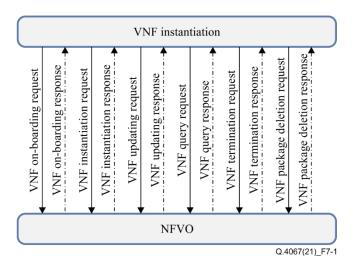
Figure 7-1 – Messages of the VNF lifecycle management in the testing environment
