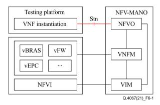
Figure 6-1 – The VNF lifecycle management signalling architecture in a testing environment
