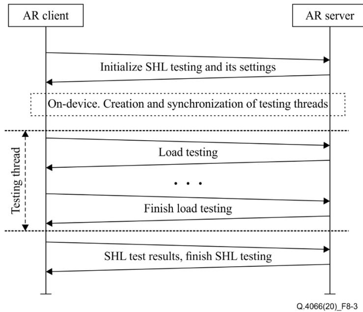
**Figure 8-3 – Server high-load testing scenario**
