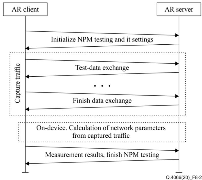
**Figure 8-2 – Network parameters measurement testing scenario**
