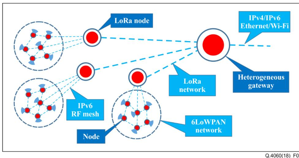
**Figure 1 – Example of a gateway in a heterogeneous network**
