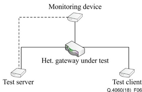
**Figure 6 – Typical gateway test configuration**
