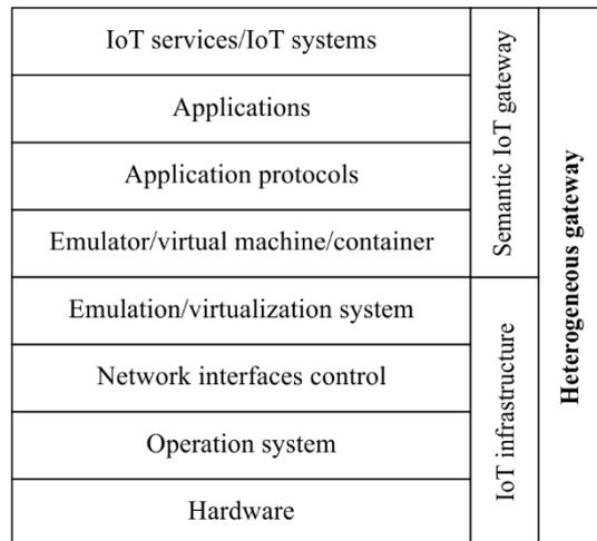
**Figure 3 – Structure of heterogeneous gateway**
