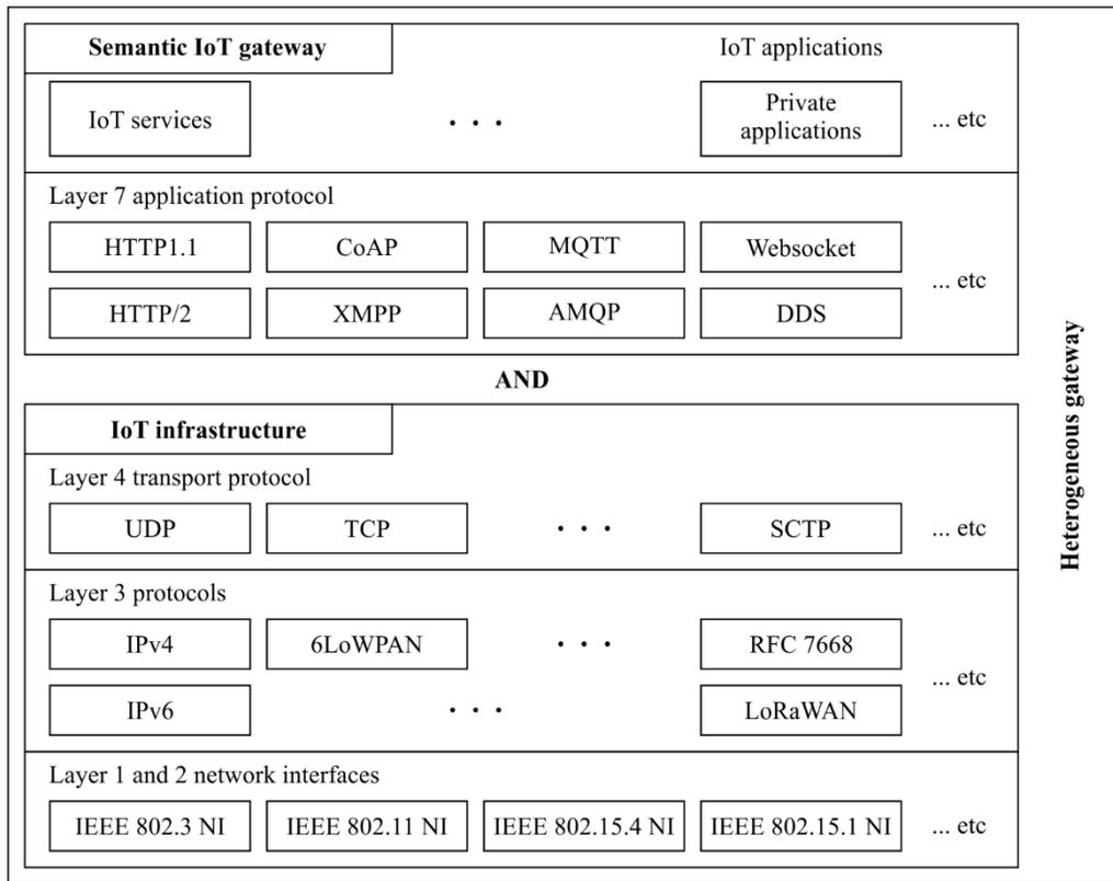
**Figure 2 – Functional architecture of an IoT gateway using a semantic IoT gateway**
