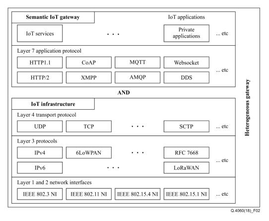
Figure 2 – Functional architecture of an IoT gateway using a semantic IoT gateway
