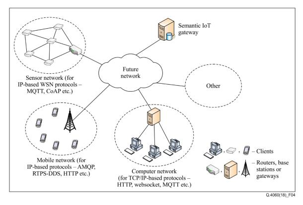
Figure 4 – Example of inter-protocol communication via future network using semantic gateways
