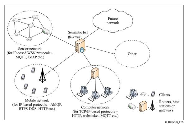
Figure 5 – Example using a semantic gateways scheme to construct local networks
