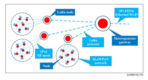
Figure 1 – Example of a gateway in a heterogeneous network
