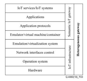
Figure 3 – Structure of heterogeneous gateway
