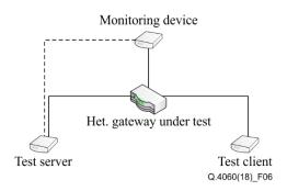
Figure 6 – Typical gateway test configuration
