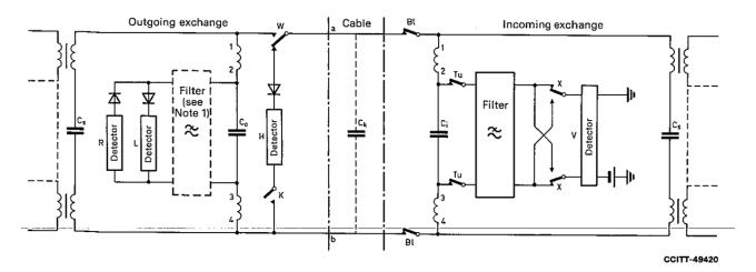
Note 1 - This filter is optional. Note 2 - The detector V and the contacts X for the reversal of the direction of the current may be interchanged.
