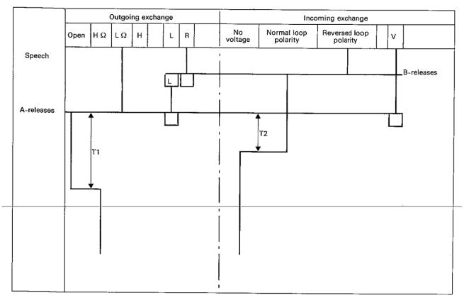
d) In-connection with subscriber releasing the incoming exchange blocks by means of open loop (without metering) CCITT-49460
