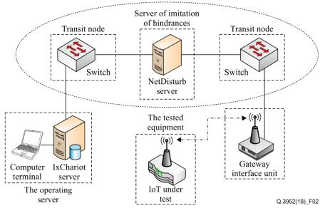
Figure 2 – Block diagram of the base part model network
