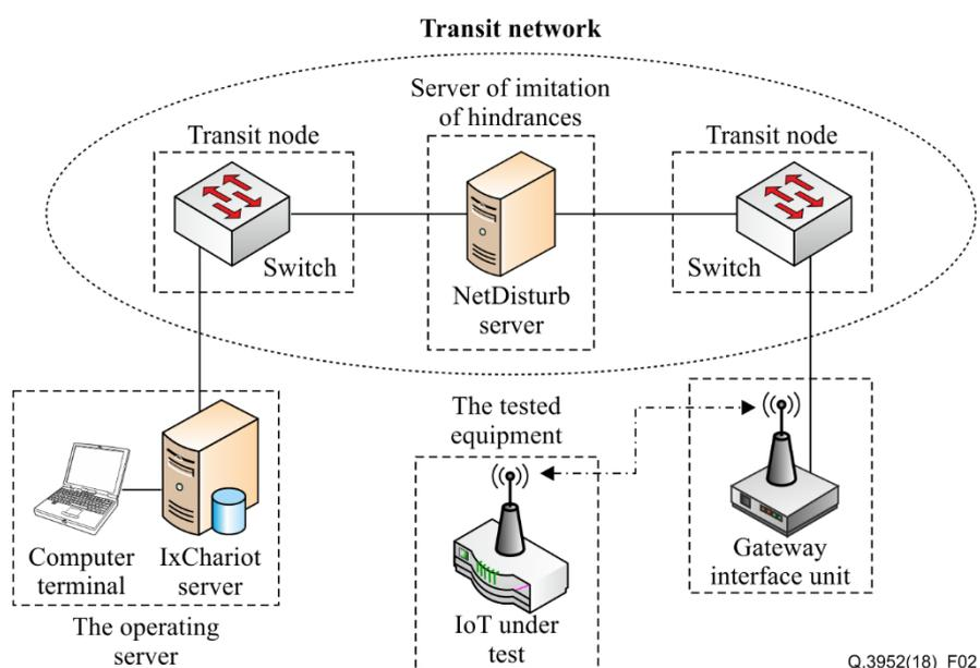
**Figure 2 – Block diagram of the base part model network**
