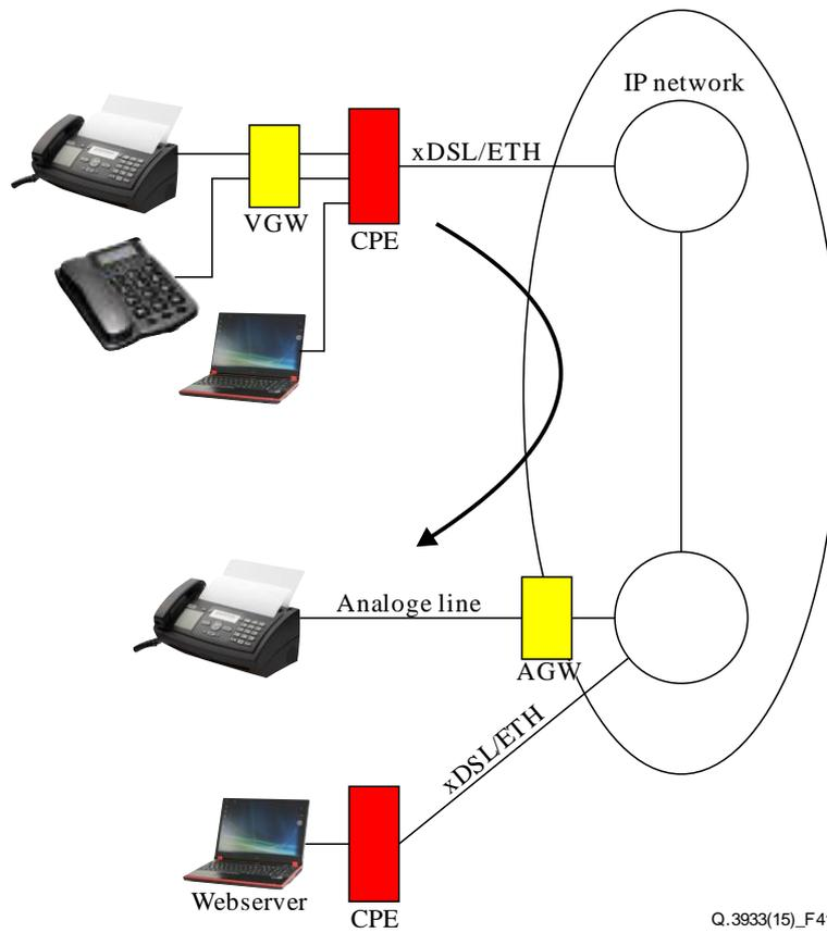
**Figure 41 – Call between VGW fax UE with additional data traffic and AGW fax UE**
