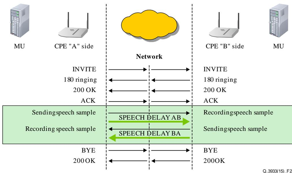
**Figure 27 – VoIP measurement of the speech delay**
