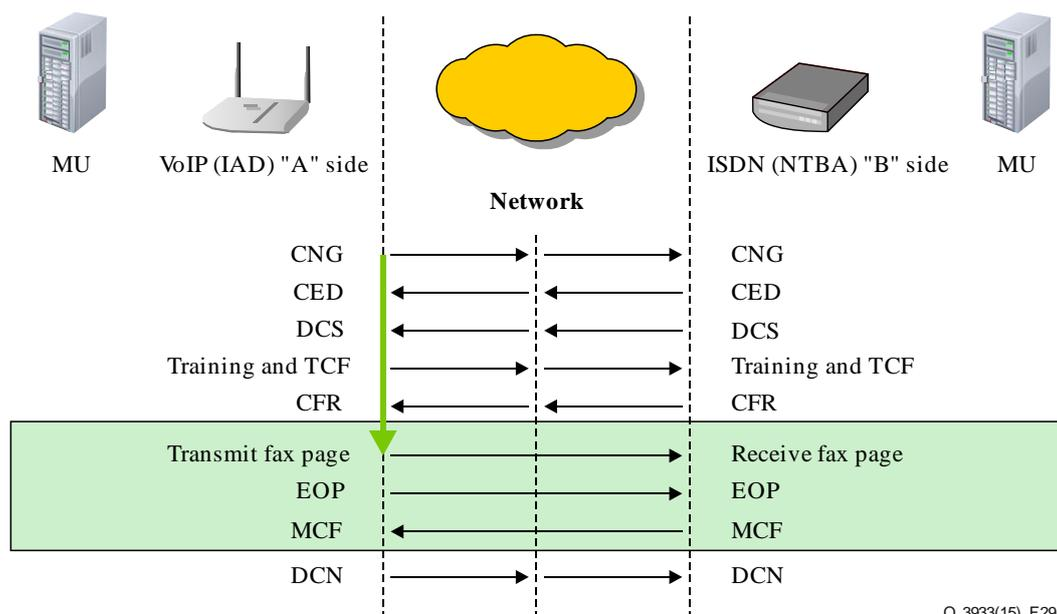
**Figure 29 – Fax set-up duration**
