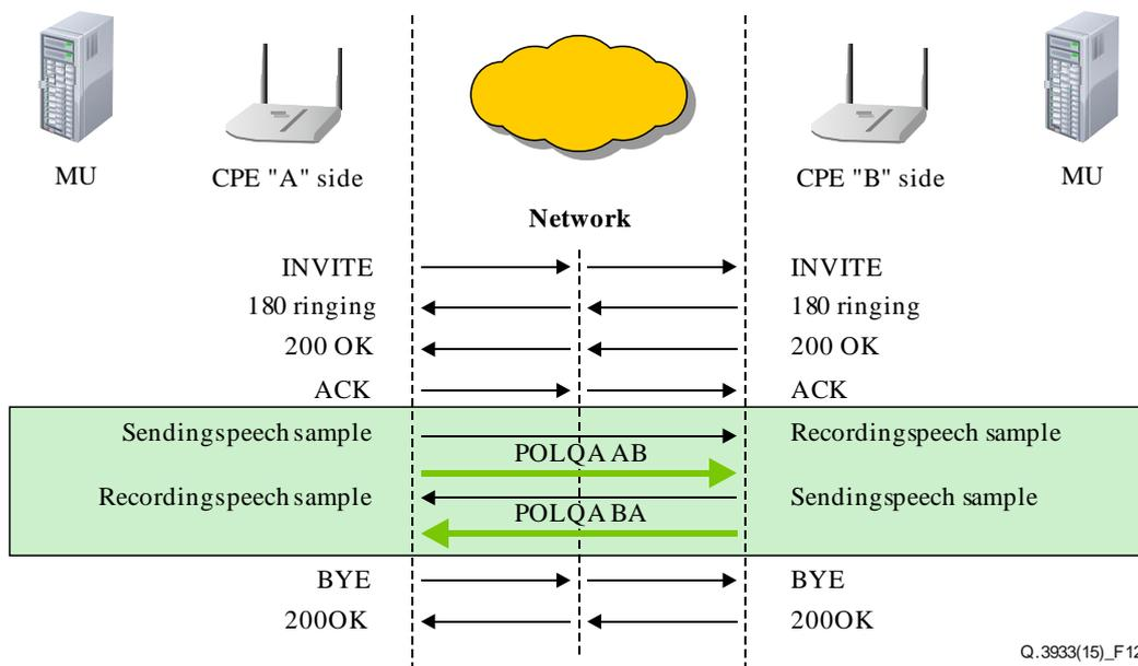
**Figure 12 – VoIP measurement of voice quality, MMTel fixed to MMTel fixed**
