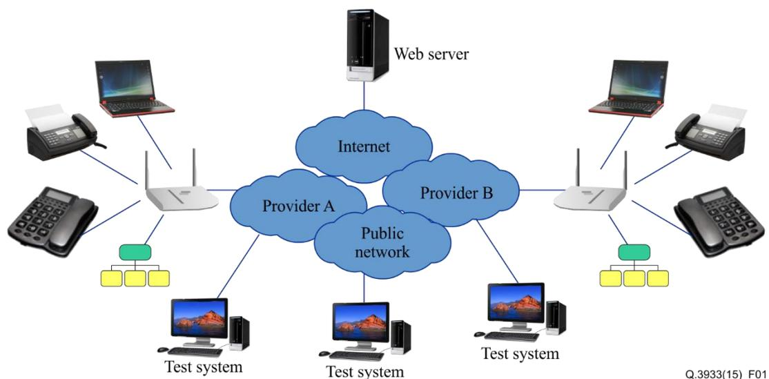
Figure 1 – Set-up of the benchmarking platform
