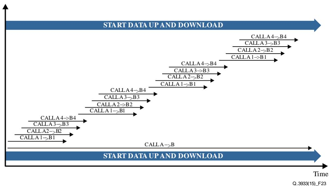
**Figure 23 – Multiple voice channel access test**
