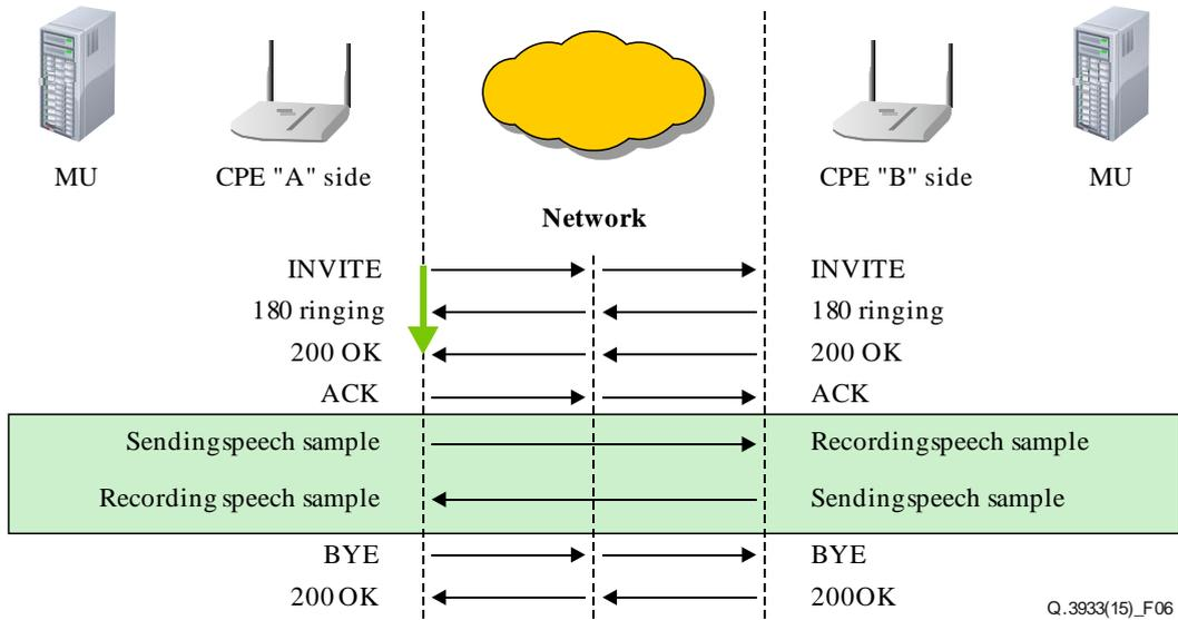
**Figure 6 – VoIP measurement of the call set-up duration, option A with 200 OK**
