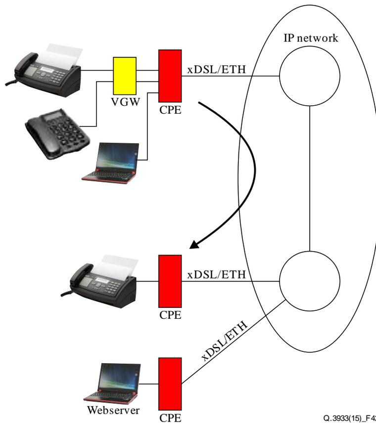
**Figure 42 – Call between VGW fax UE with additional data traffic and MMTel (IMS)**
