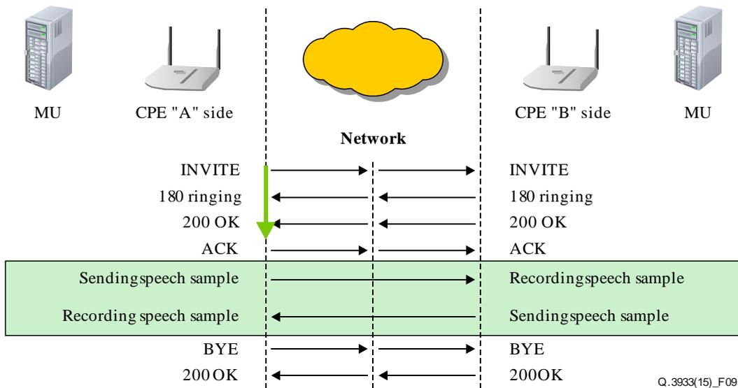
**Figure 9 – VoIP – determination of the call drop ratio**
