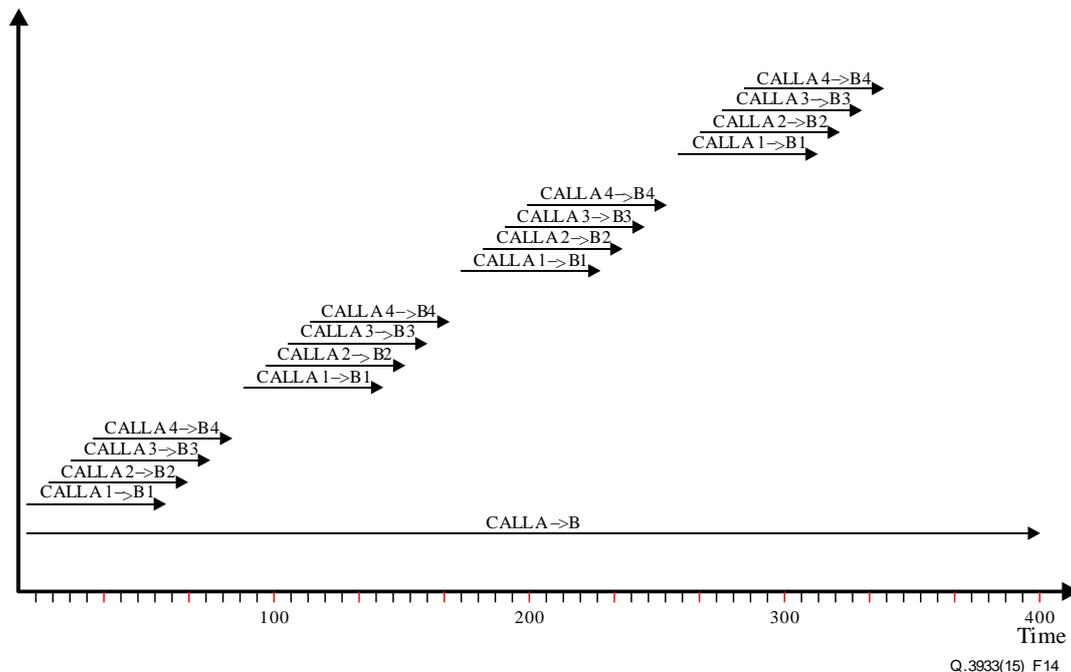
**Figure 14 – Example of multiple voice channel access test**
