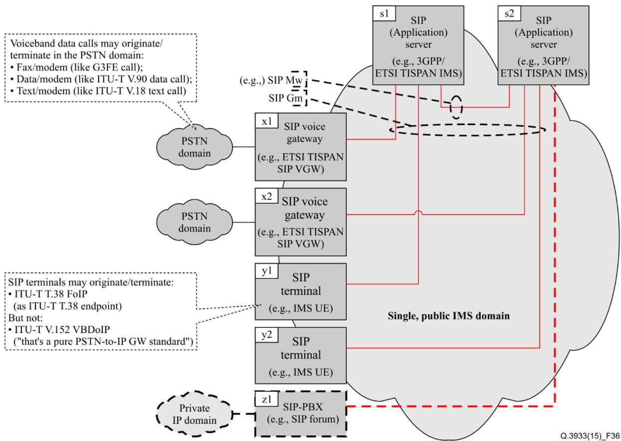
**Figure 36 – Mix of SIP VGWs (IMS-based PES) & SIP user equipment (UE) (IMS)**
