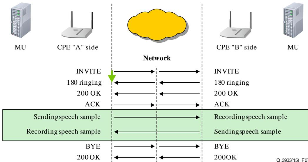
**Figure 7 – VoIP measurement of the call set-up duration, option B with 180 Ringing**
