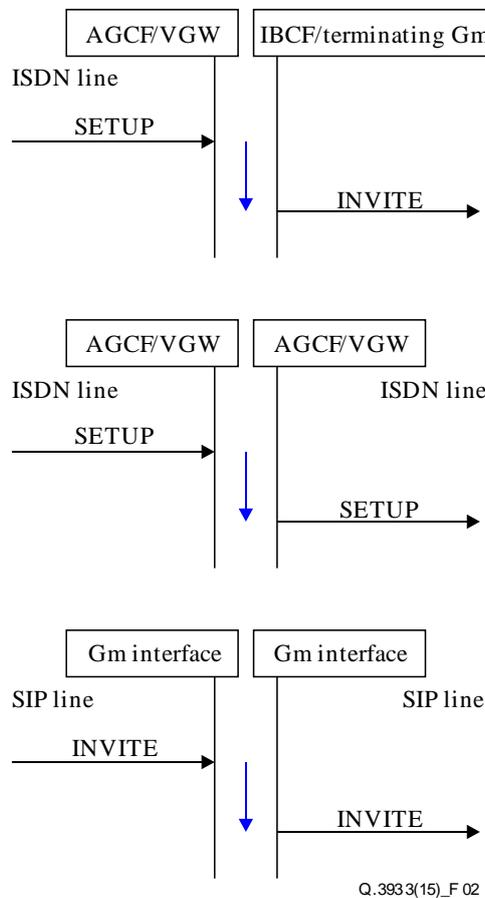
**Figure 2 – Call set-up delay and session initiation call set-up delay: En-bloc sending is used**
