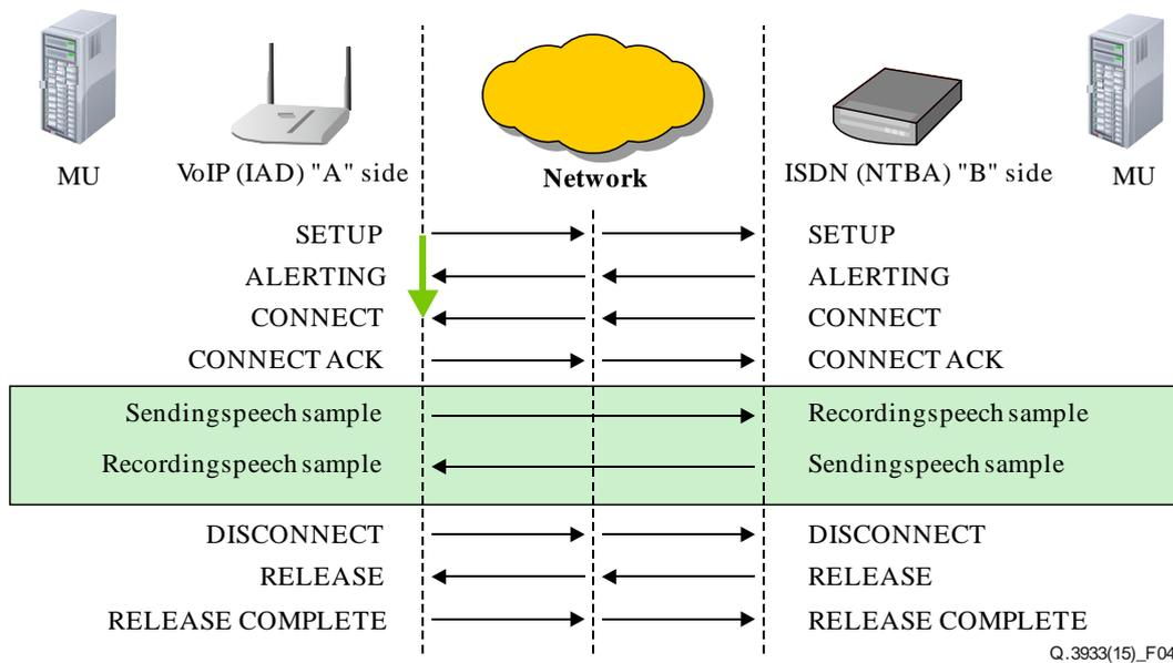
**Figure 4 – Measurement of the call set-up duration, option A with CONNECT**
