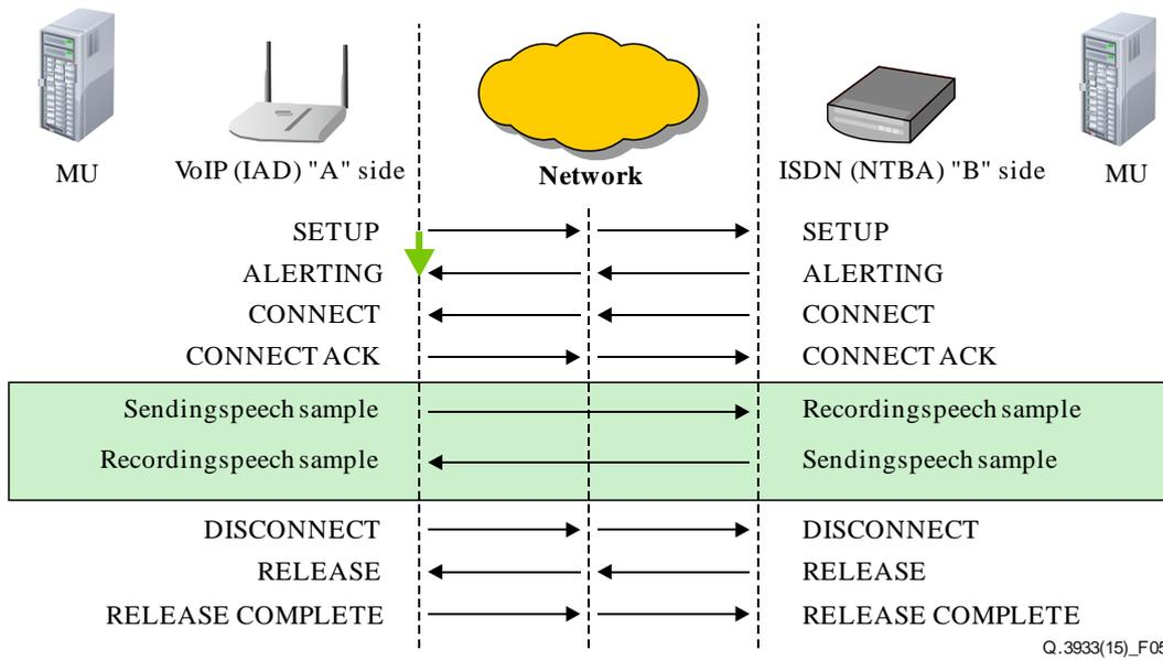
**Figure 5 – Measurement of the call set-up duration, option B with ALERTING**
