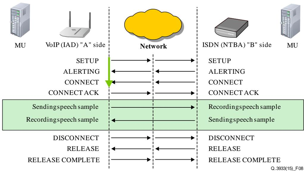
**Figure 8 – Determination of the call drop ratio**
