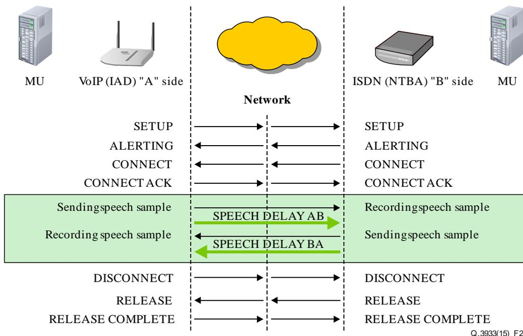
**Figure 26 – Measurement of the speech delay**
