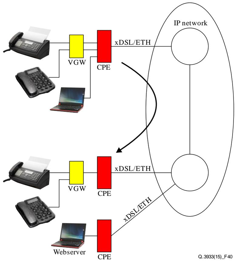
**Figure 40 – Call between two VGW fax UE with additional data traffic**
