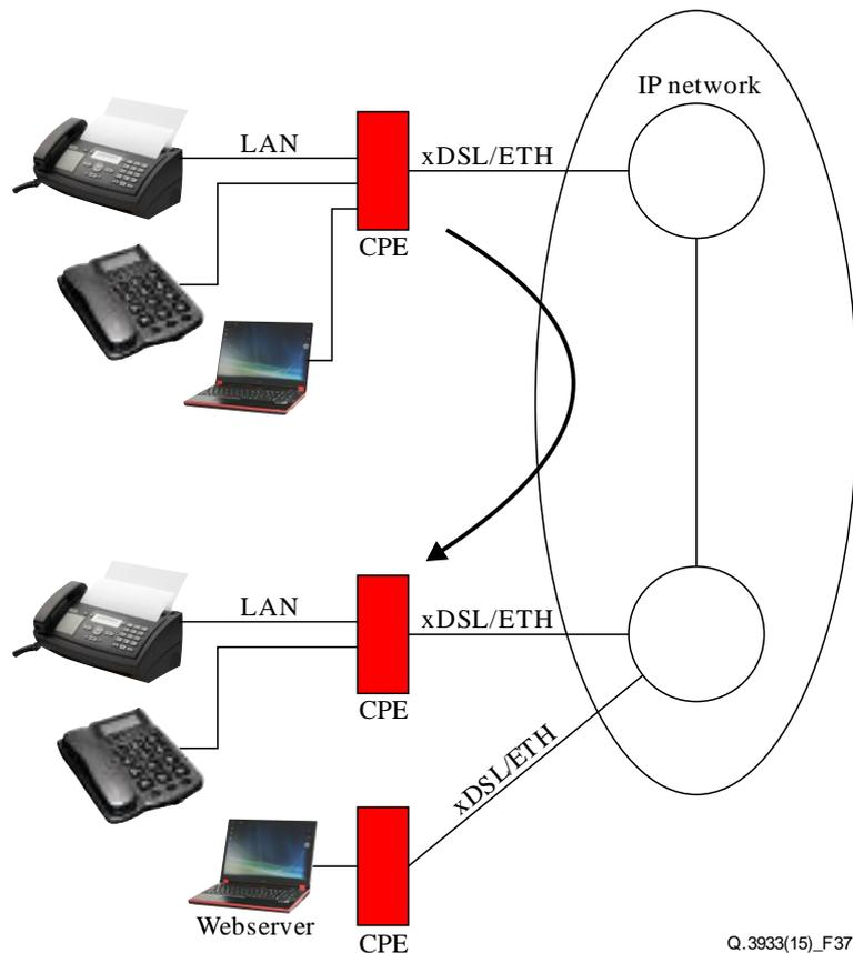
**Figure 37 – Call between two MMTel (IMS) fax UE with additional data traffic**
