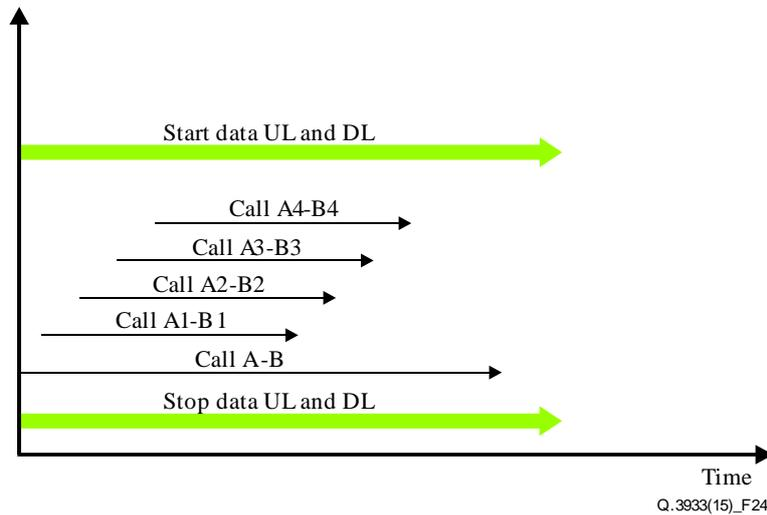
**Figure 24 – Parallel quality measurement of multiple voice channels and data transmission speed**
