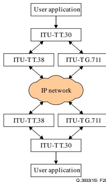
**Figure 28 – FAX Stack for FoIP**
