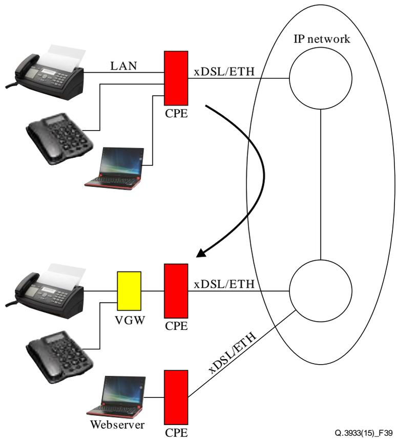
**Figure 39 – Call between MMTel (IMS) fax UE with additional data traffic and VGW fax UE**
