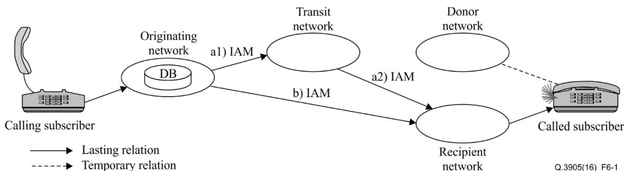
**Figure 6-1 – The signalling transfer for the method "all call query"**
