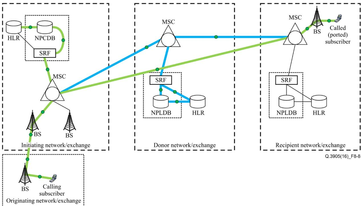
**Figure 8-8 – Network Configuration for test case 8.11**
