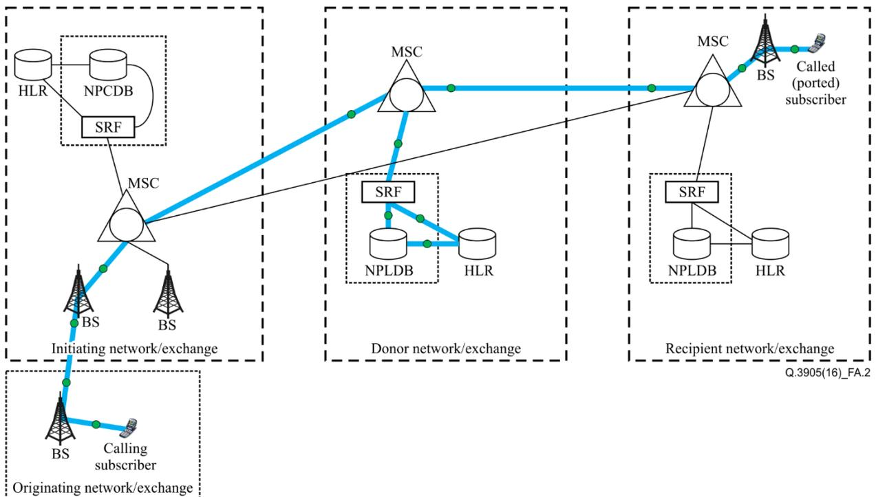
**Figure A.2 – Network configuration for test case A.02**
