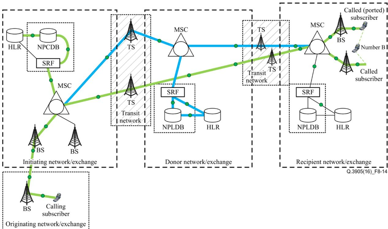
Figure 8-14 – Network configuration for test case 8.20
