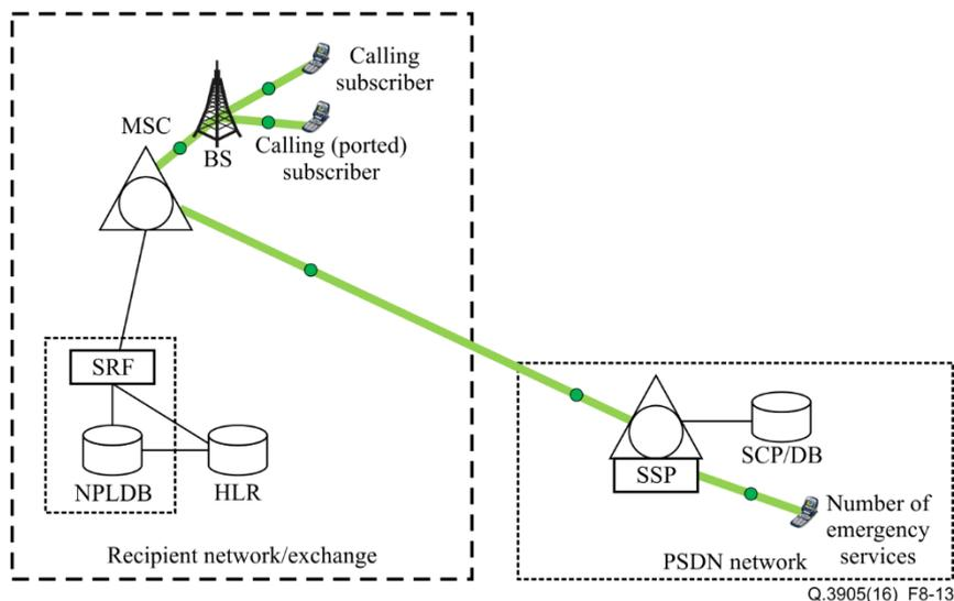
**Figure 8-13 – Network configuration for test case 8.17**
