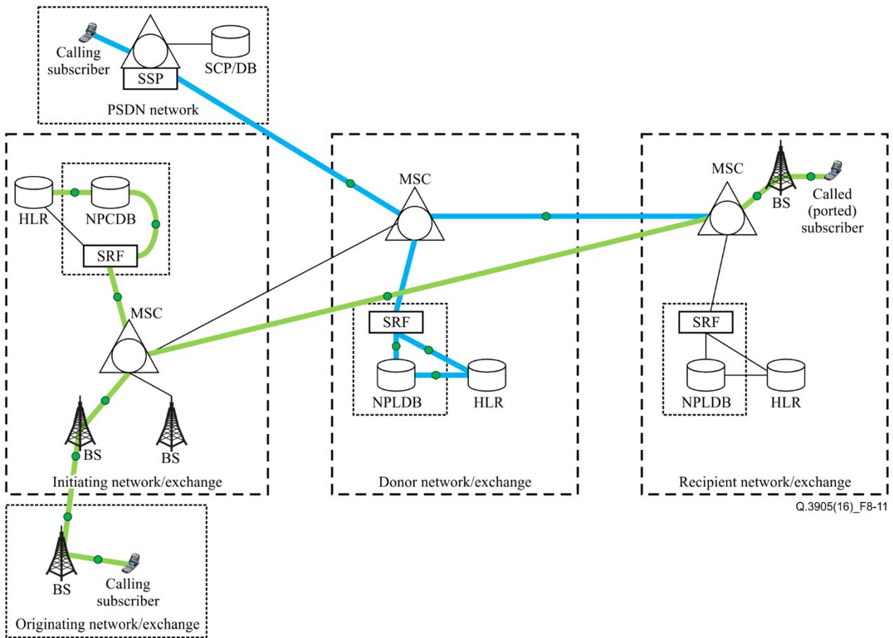
**Figure 8-11 – Network configuration for test case 8.15**
