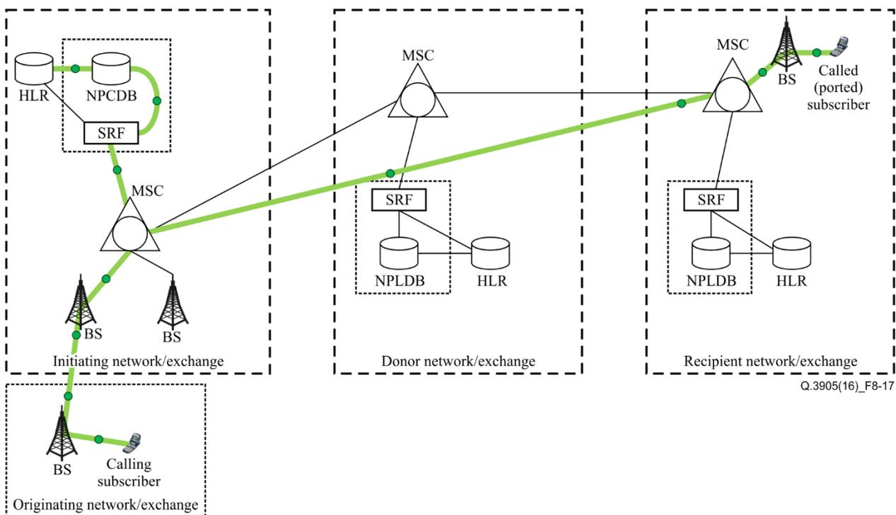
**Figure 8-17 – Network configuration for test case 8.25**
