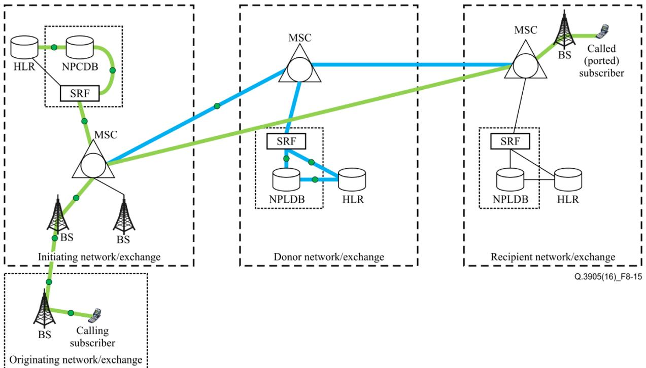
**Figure 8-15 – Network configuration for test case 8.22**
