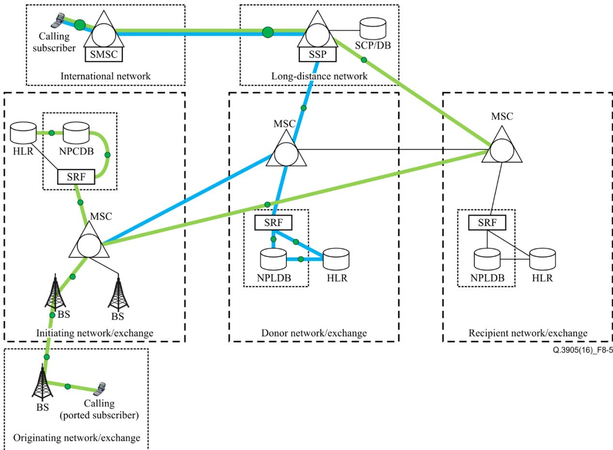
Figure 8-5 – Network configuration for test case 8.06
