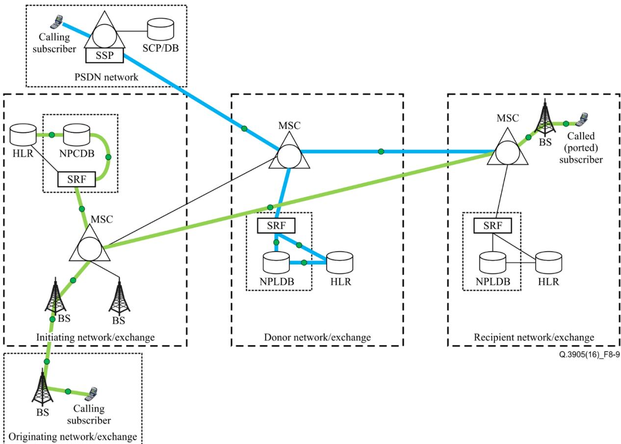
**Figure 8-9 – Network Configuration for test case 8.12**
