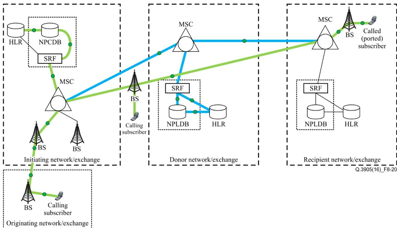
Figure 8-20 – Network configuration for test case 8.30
