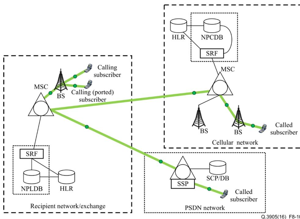
**Figure 8-10 – Network configuration for test case 8.13**
