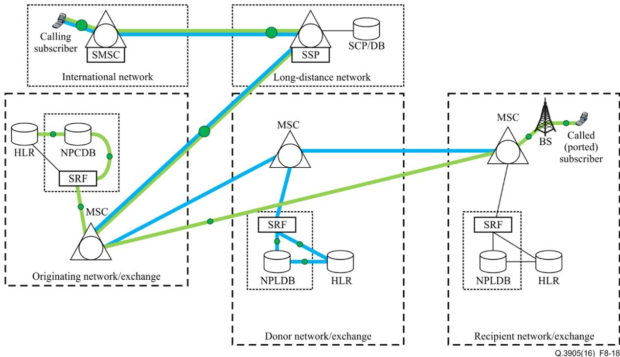
Figure 8-18 – Network configuration for test case 8.26
