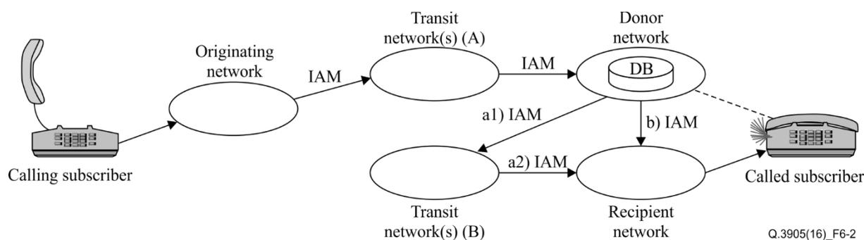
**Figure 6-2 – The signalling transfer for the method "onward routing"**
