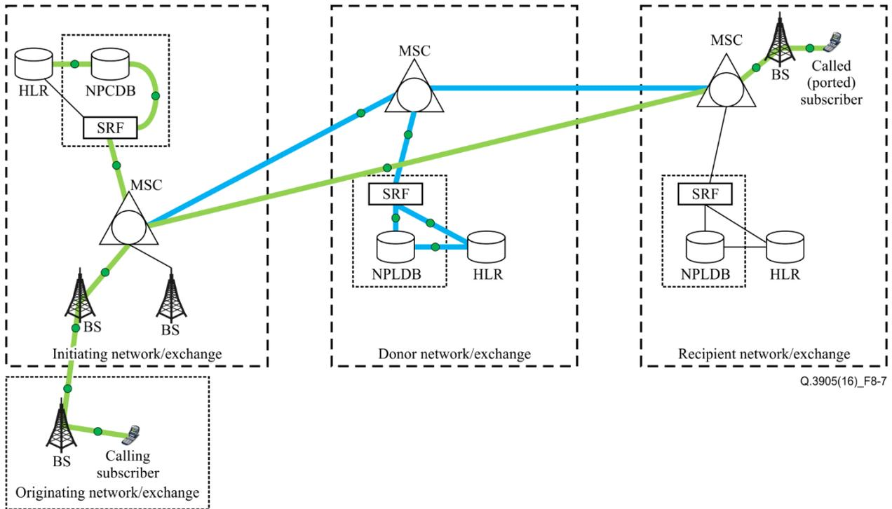
Figure 8-7 – Network configuration for test case 8.10.
