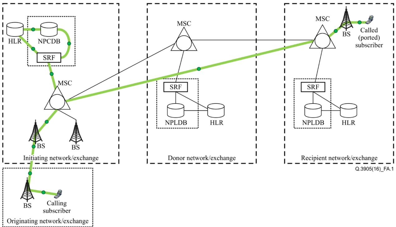
**Figure A.1 – Network configuration for test case A.01**
