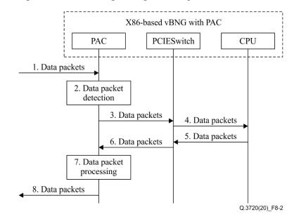
Figure 8-2 depicts the procedure for data packet processing in in-line mode.
