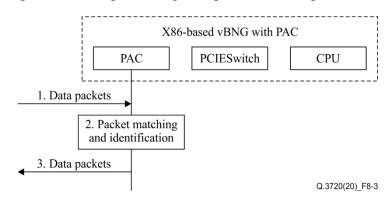
Figure 8-3 – Procedure for processing data packets in fast-path mode
