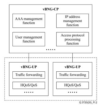
Figure I.2 – Distributed deployment of vBNG with PAC
