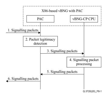
Figure 8-1 – Procedure for processing signalling packets
