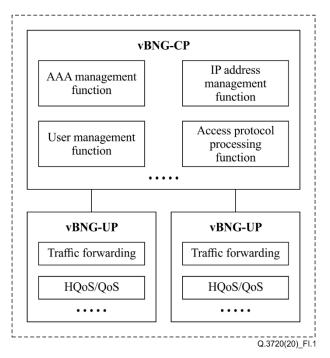
Figure I.1 –Centralized deployment of vBNG with PAC
