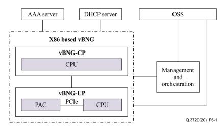
Figure 6-1 – Framework for X86-based vBNG acceleration with PAC
