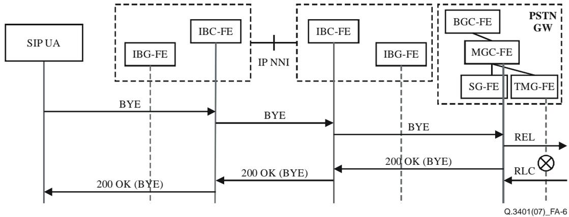
**Figure A.6 – Normal call release from SIP to ISUP**
