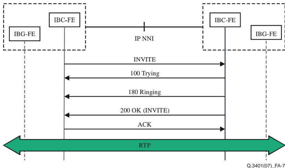
**Figure A.7 – Successful call setup at IP-IP SIP NNI**
