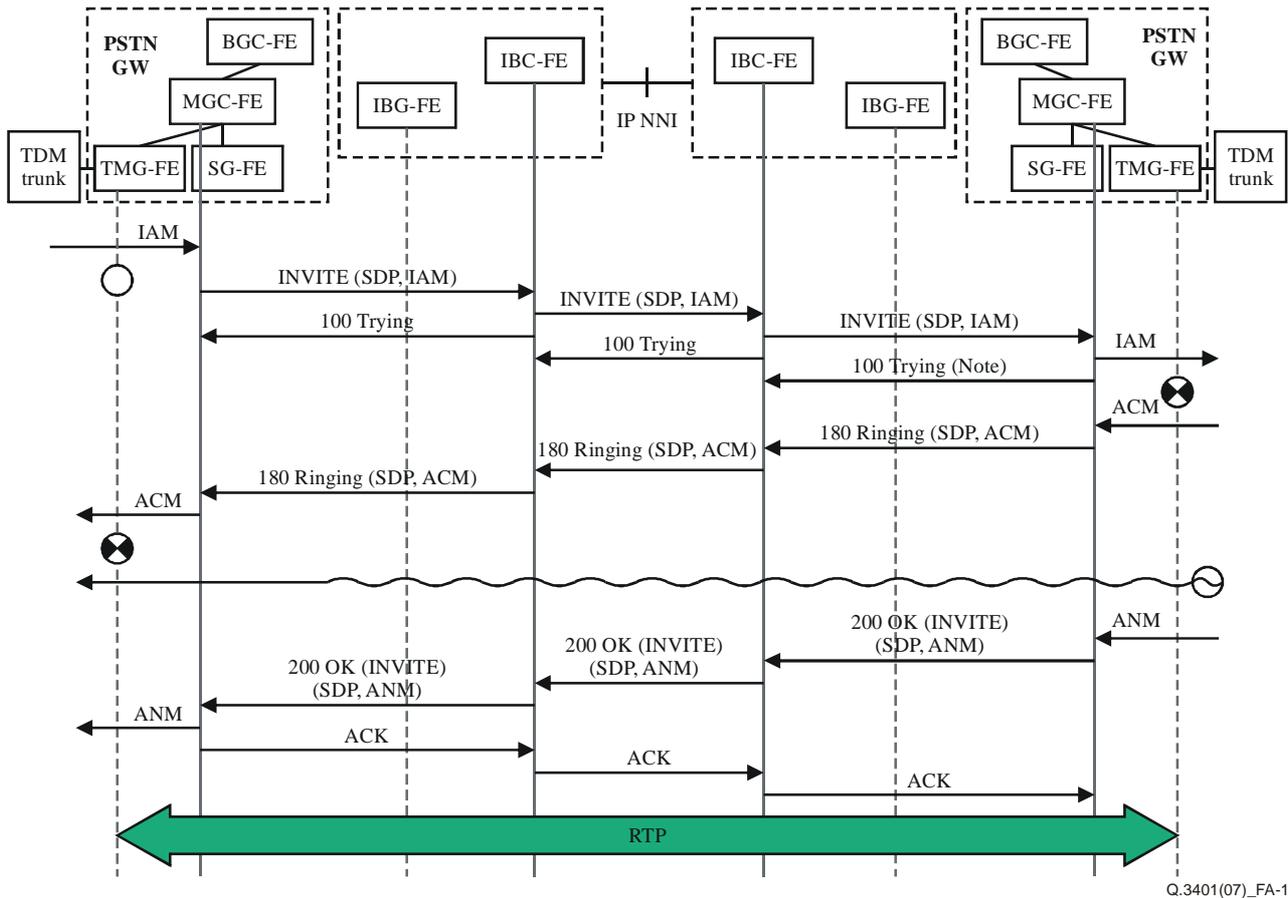
NOTE – The generation of the 100 Trying response is necessary if the PSTN gateway knows that it will not generate a provisional or final response.
