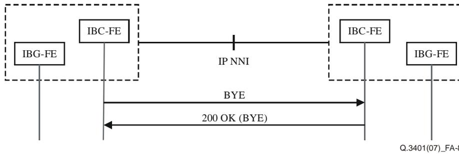
**Figure A.8 – Normal call release at IP-IP SIP NNI**
