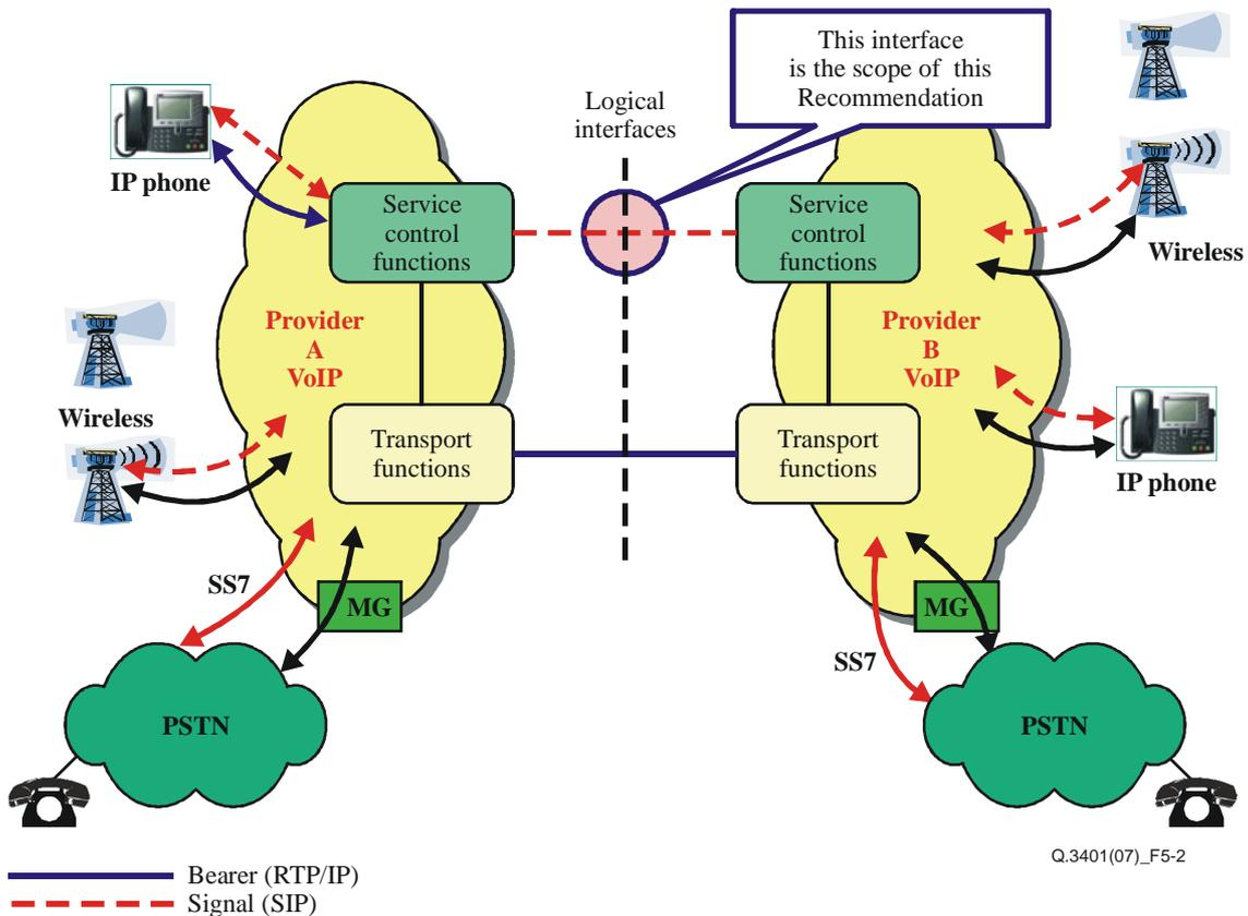
Figure 5-2 – VoIP interconnection reference model
