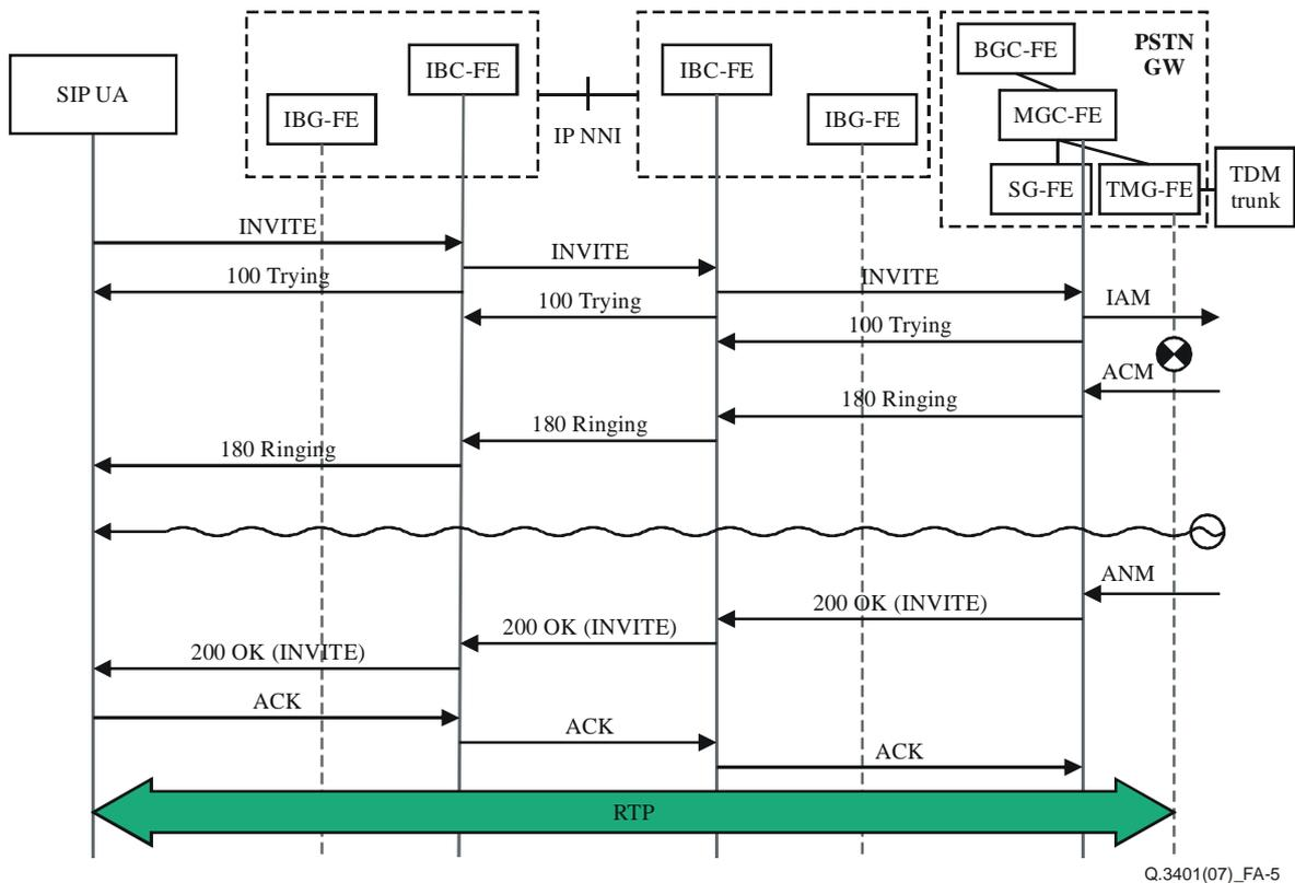
Figure A.5 – Successful call setup from SIP to ISUP
