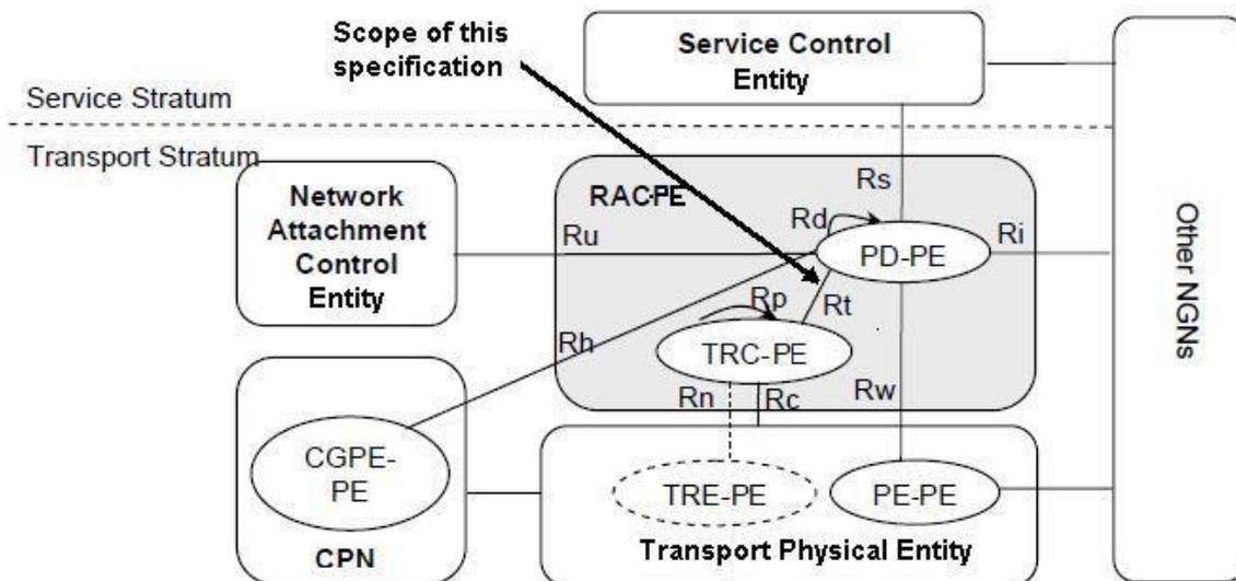
**Figure 6-1: Localization of the Rt reference point in the generic resource and admission control functional architecture in NGN**
