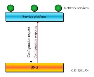
Figure 4 – Service configuration message types on BNG
