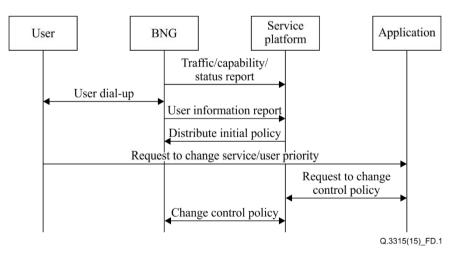
Figure D.1 – Service/user control procedure
