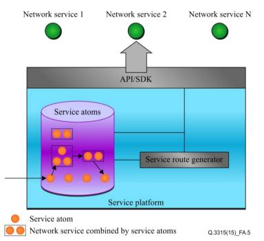
Figure A.5 – Service atoms in the service platform
