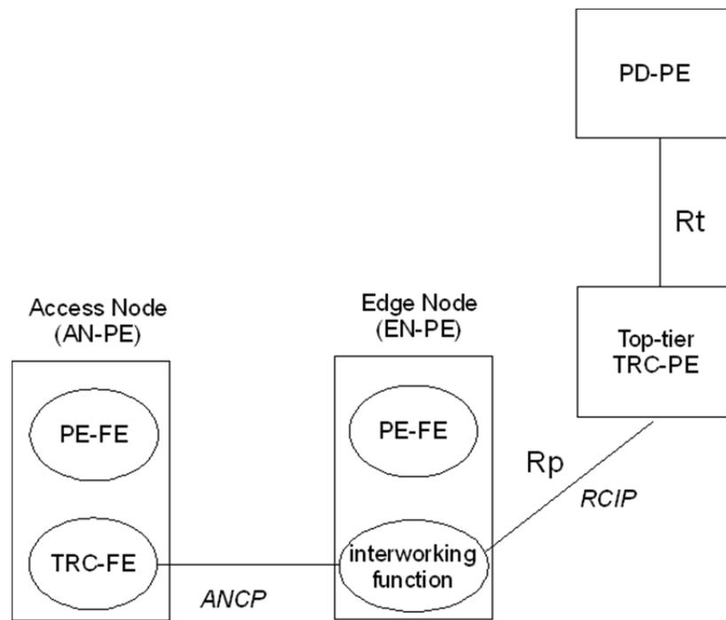
**Figure 6-1 – Architecture for joint use of ANCP and RCIP on the Rp interface**
