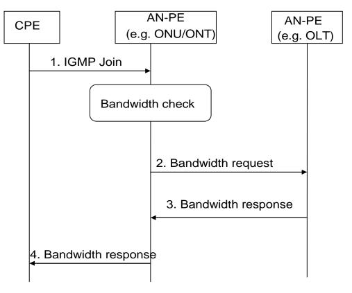
Figure 9-1 – Multicast admission control procedure when there is sufficient bandwidth in AN-PE
