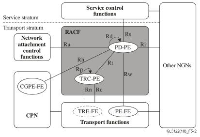
Figure 5-1 – Basic protocol architecture
