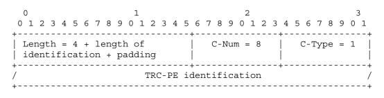
Figure 8-18 – Identity identification object content
