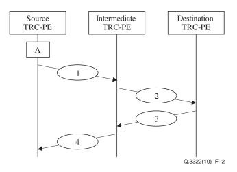
Figure I.2 – Forward unidirectional QoS path establishment information flows
