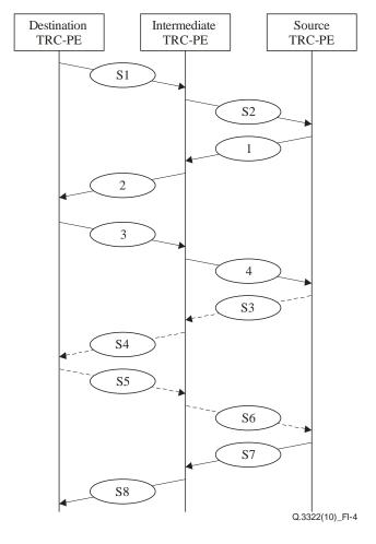
Figure I.4 – Separately-allocated forward-and-backward-resource information flows
