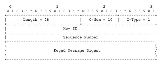
Figure 8-20 – Data consistency object content
