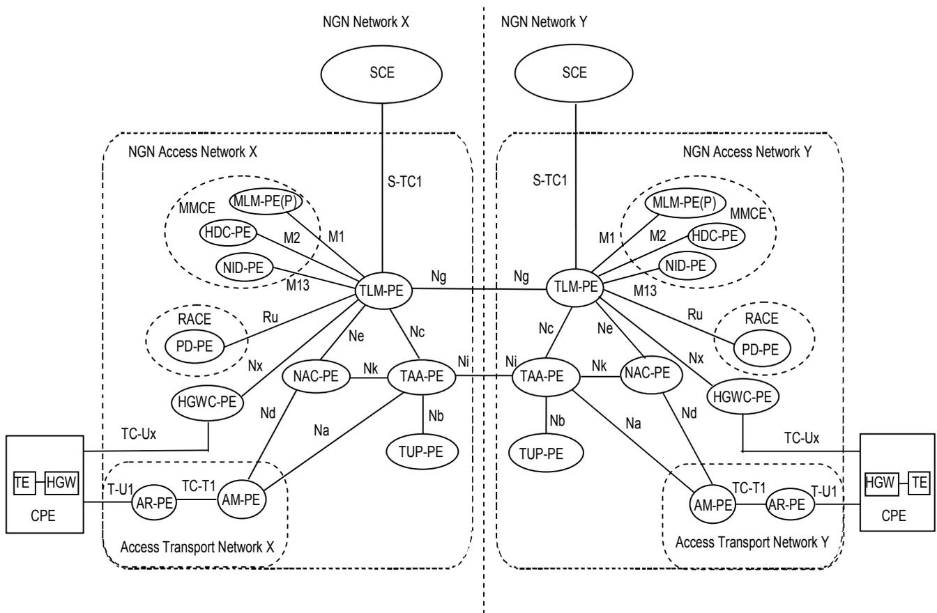
**Figure 7-2 – Example physical realization of the NACF revision 1 architecture**
