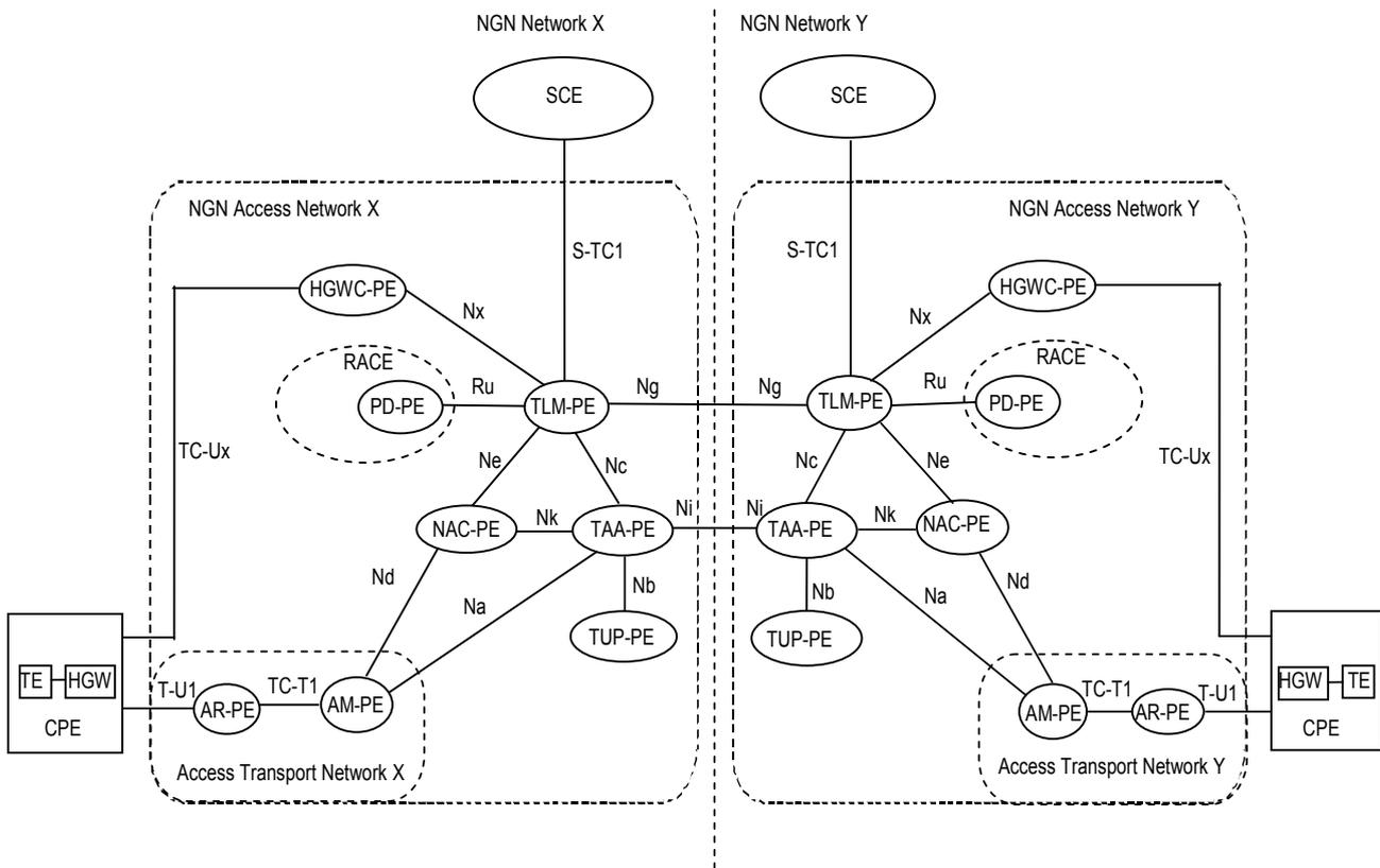
**Figure 6-2 – Example physical realization of the NACF architecture**
