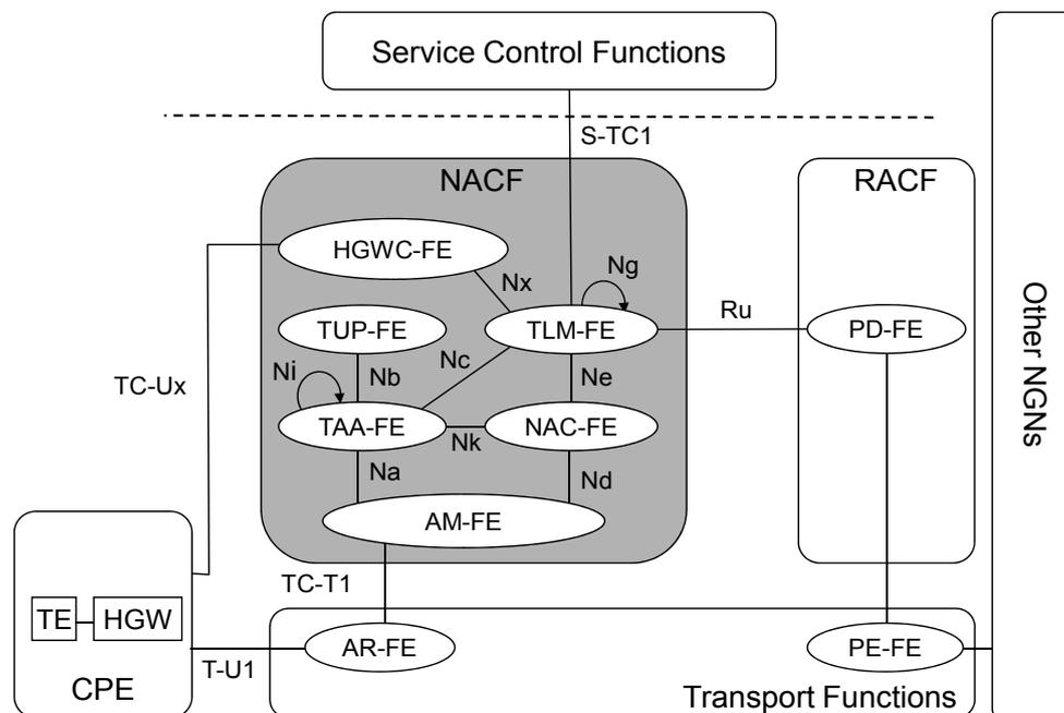
**Figure 6-1 – NACF functional architecture**
