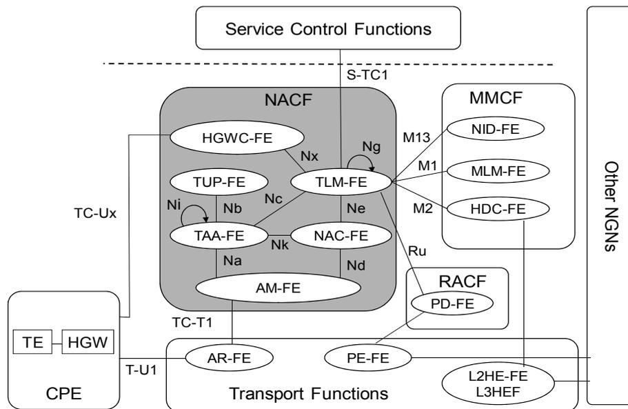
**Figure 7-1 – NACF revision 1 functional architecture**
