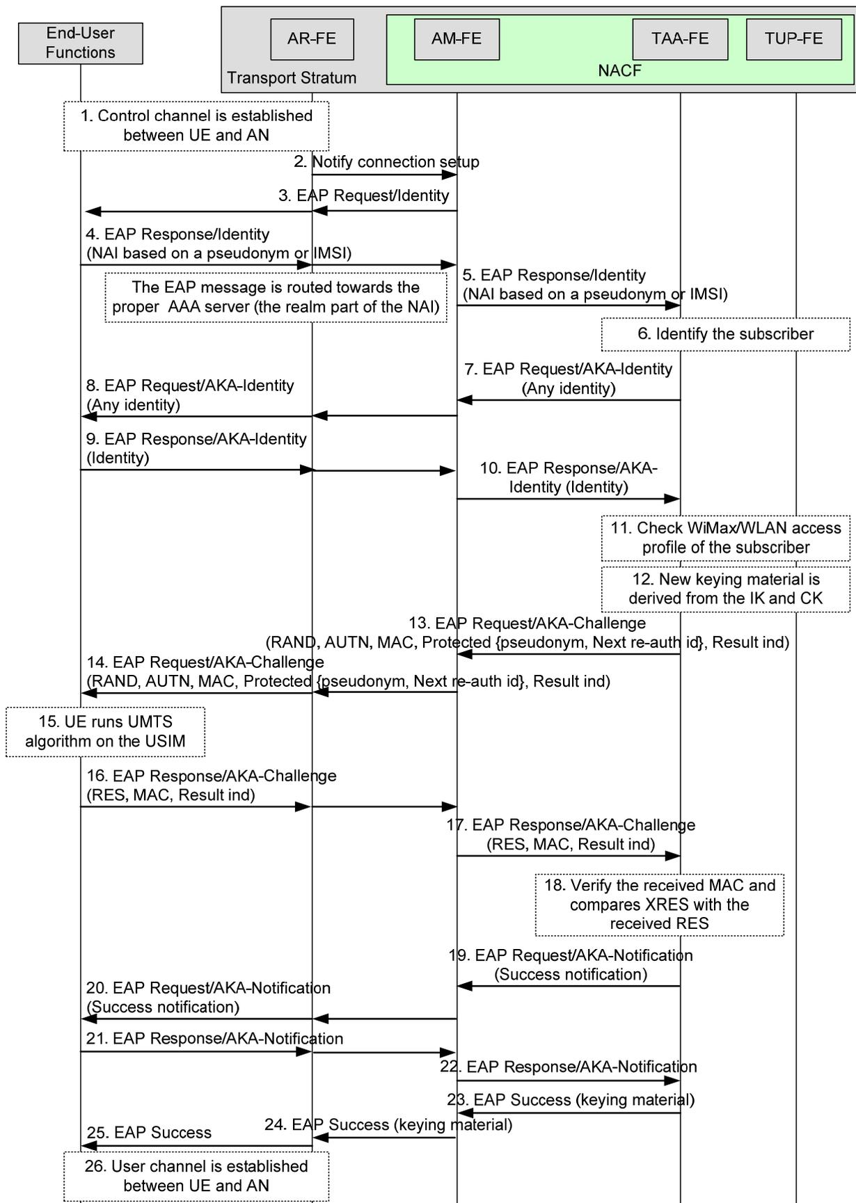
Figure I.1 – Authentication protocol based on EAP-AKA scheme with UICC in NGN
