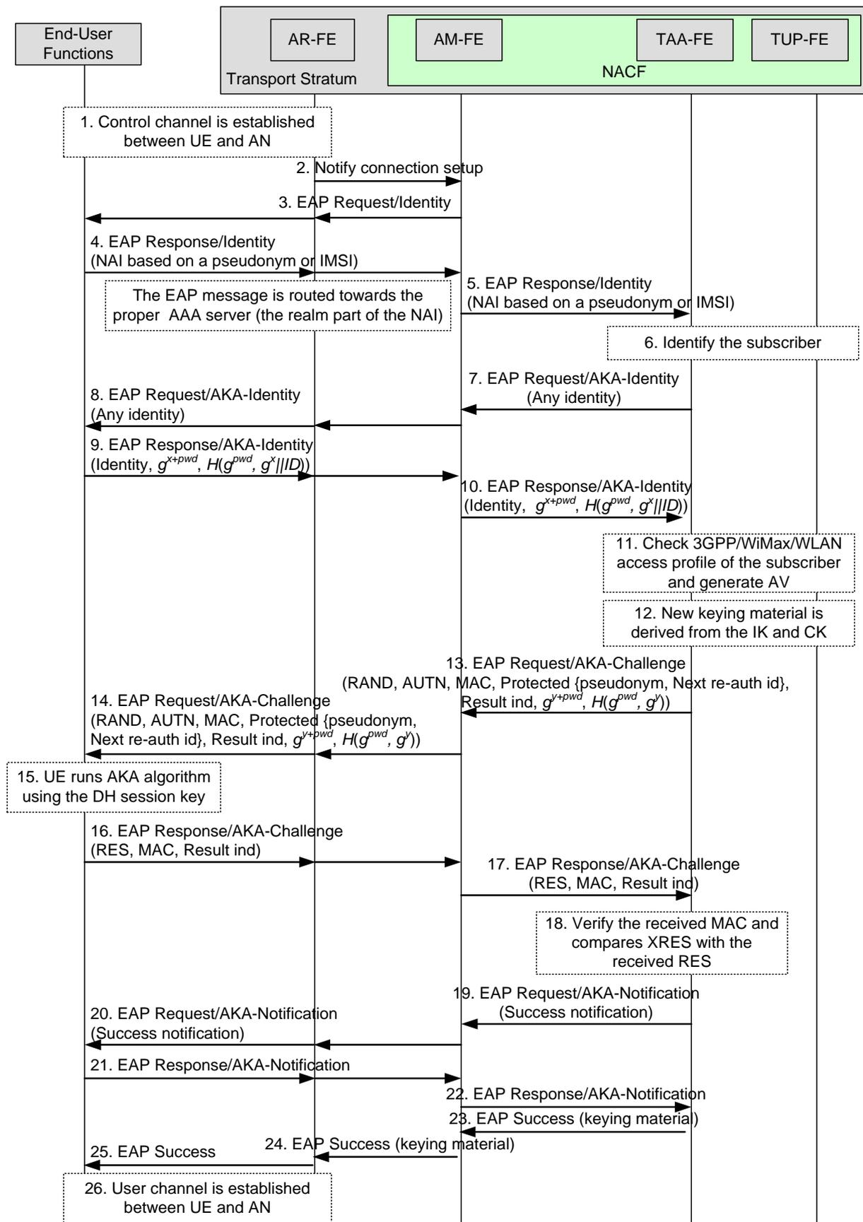
Figure I.2 – Authentication protocol based on EAP-AKA scheme with non-UICC in NGN
