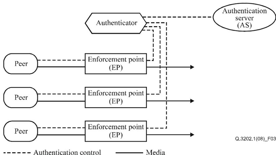
**Figure 3 – Integrated authentication model**
