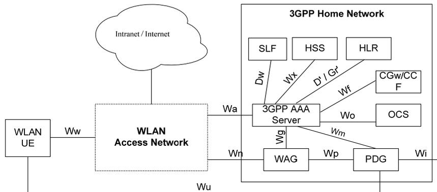
**Figure 1 – 3GPP system-based authentication model**
