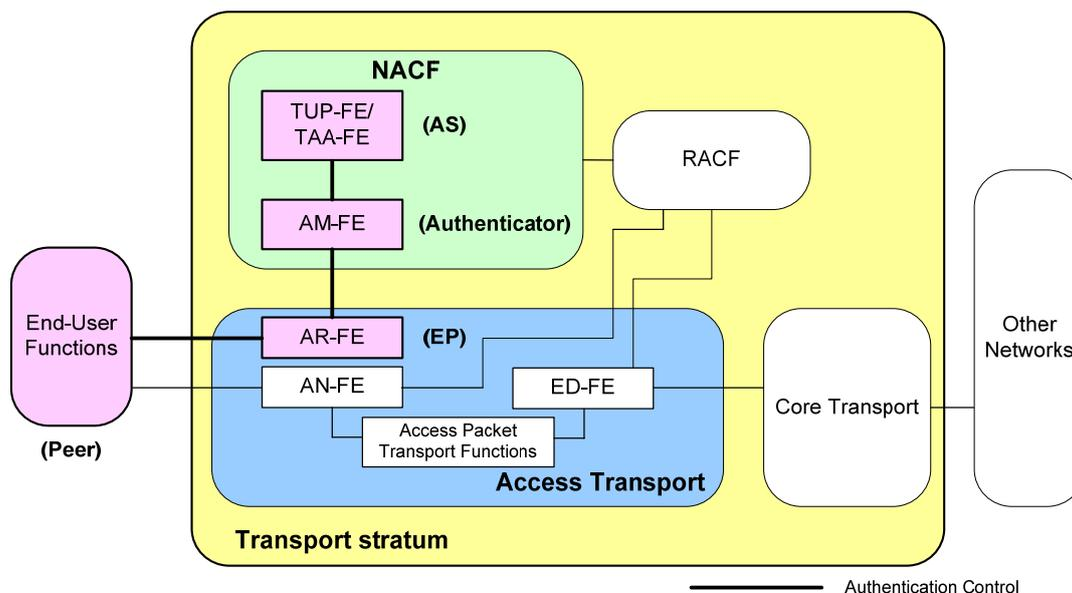
**Figure 4 – An example of an integrated authentication model in NGN**
