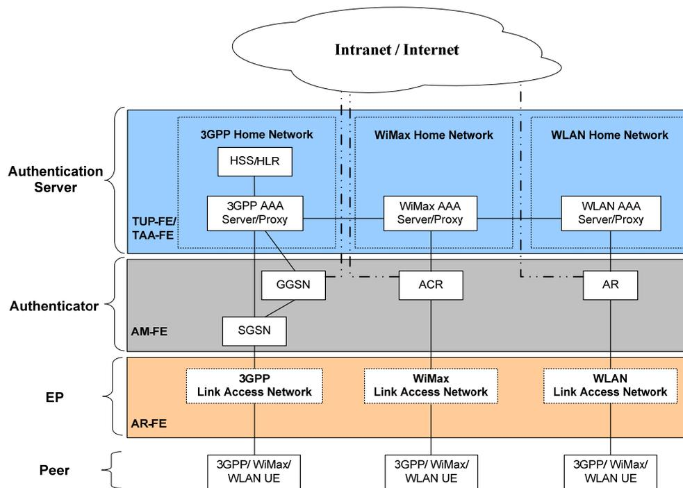
**Figure 2 – An example authentication architecture for interworking among wireless access networks in NGN**
