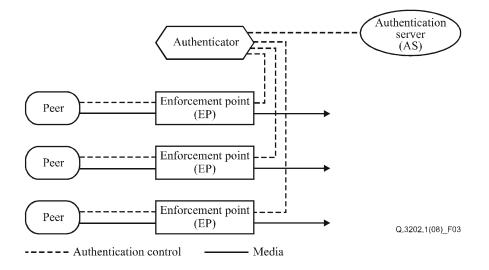
**Figure 3 – Integrated authentication model**
