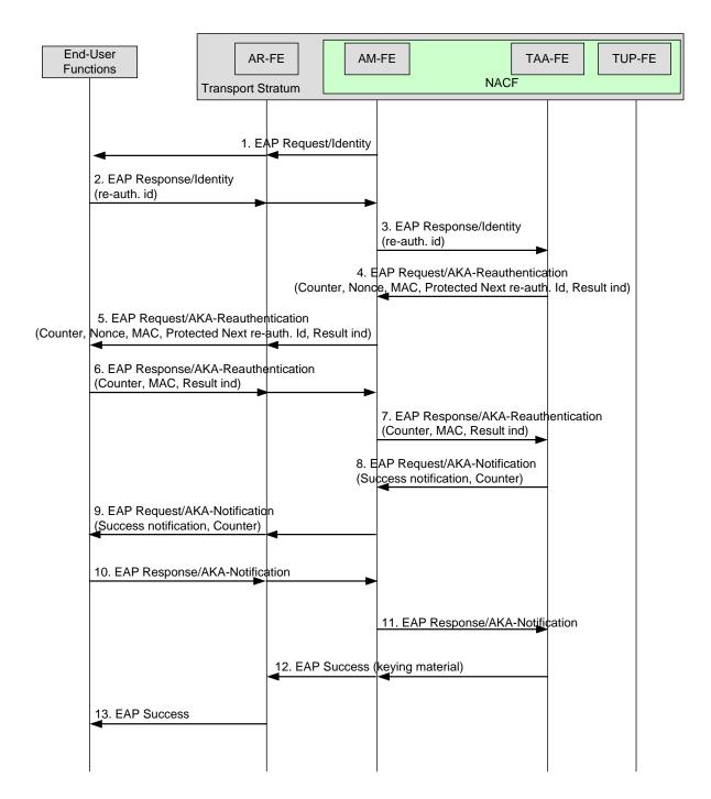
Figure I.3 – Fast re-authentication procedure of the EAP-AKA protocol in NGN
