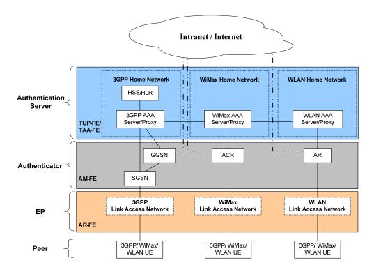
Figure 2 – An example authentication architecture for interworking among wireless access networks in NGN
