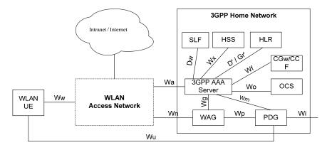
Figure 1 – 3GPP system-based authentication model
