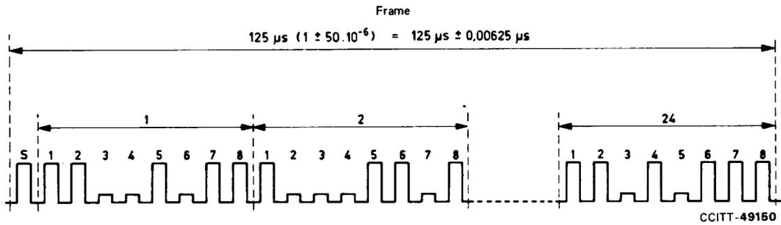
**Sampling frequency**  $8000 (1 \pm 50 \times 10^{-6}) \text{ Hz} = 8000 \pm 0.4 \text{ Hz}$
