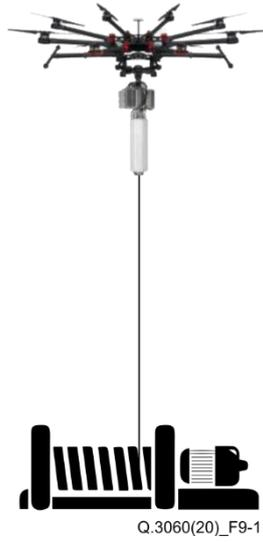
**Figure 9-1 – Tethered high-altitude unmanned platform application example**
