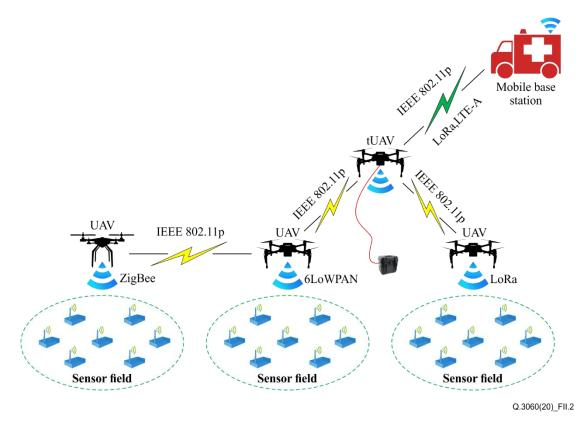
Figure II.2 – Architecture for data collection from sensor fields in a flying network for emergencies using tethered multicopters
