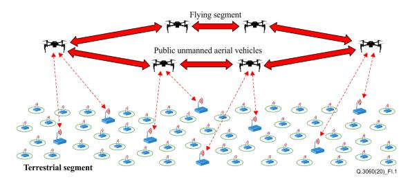
Figure I.1 – Flying ubiquitous sensor network architecture
