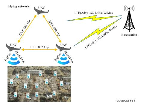
Figure 6-1 – Structure of a fast-deployment flying emergency services network for data collection from a sensor field
