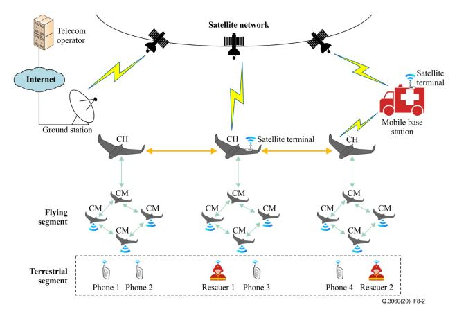
Figure 8-2 – An architecture for flying ad-hoc network for emergency
