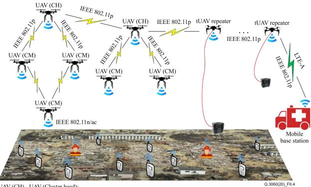
UAV (CH) - UAV (Cluster head); UAV (CM) - UAV (Cluster member); tUAV - Tethered UAV.
