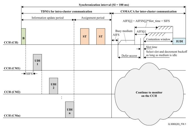
Figure III.1 – Operation of CMMpP including IntraCP and InterCP on the CCH
