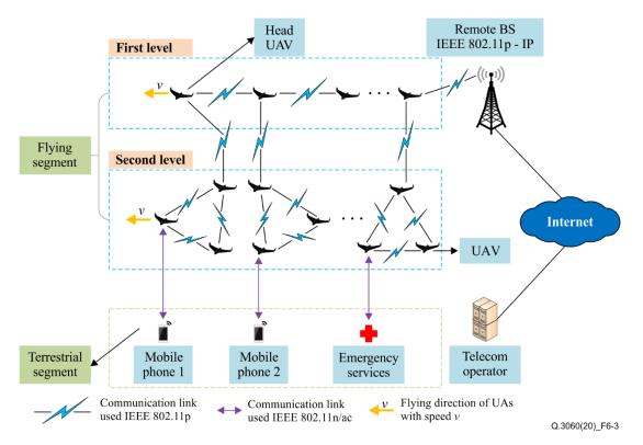
Figure 6-3 – UAV hierarchical structure for providing voice services
