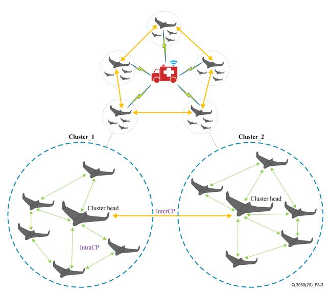
Figure 8-3 – Groups of mission-oriented UAVs around a mobile base station
