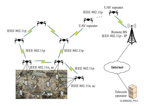
Figure 6-2 – Structure of a fast-deployment flying emergency services network providing communications between subscribers
