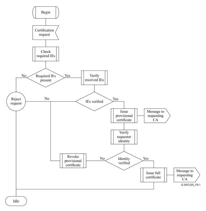
Figure 9-1 – signalling procedures of TSCA
