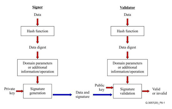
Figure 6-1 – PKI digital signature verification process [ITU-T X.509]
