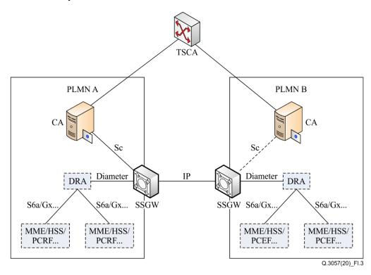
Figure I.3 – Security Diameter transaction architecture
