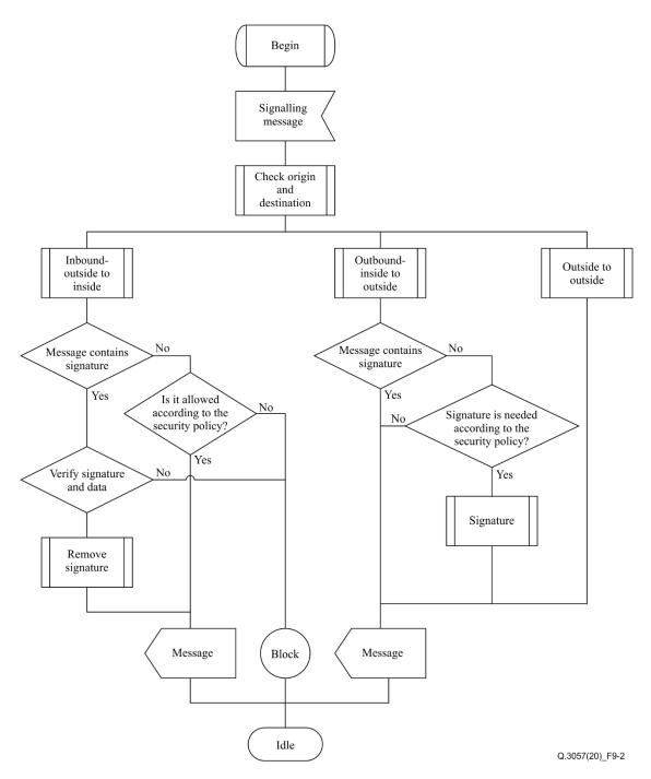
Figure 9-2 – Signalling procedures of SSGW
